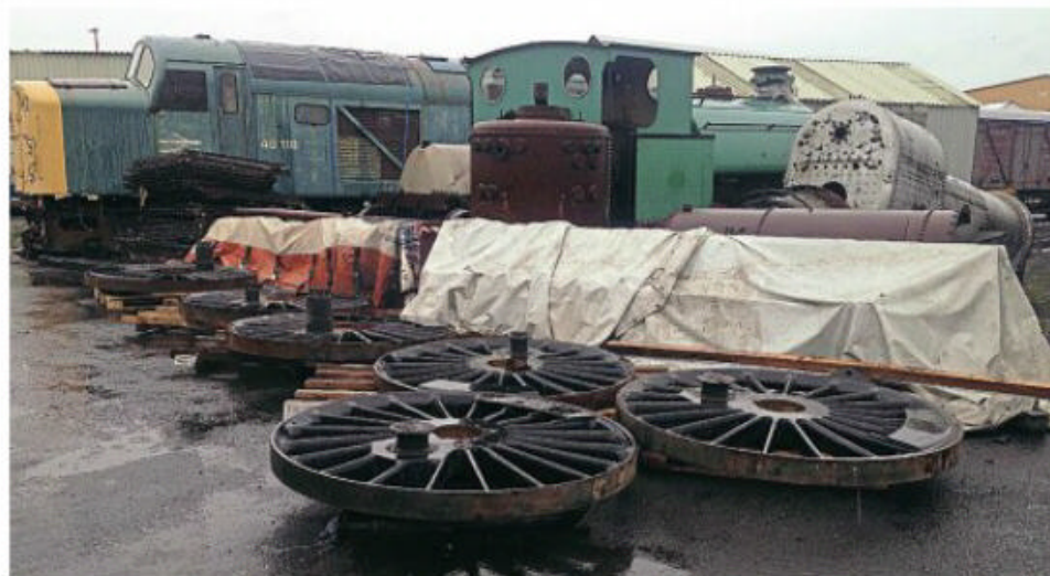
Above: Members of the team at Tyseley Locomotive Works have completed the welding up of the driving wheel bores. TREVOR TUCKLEY
