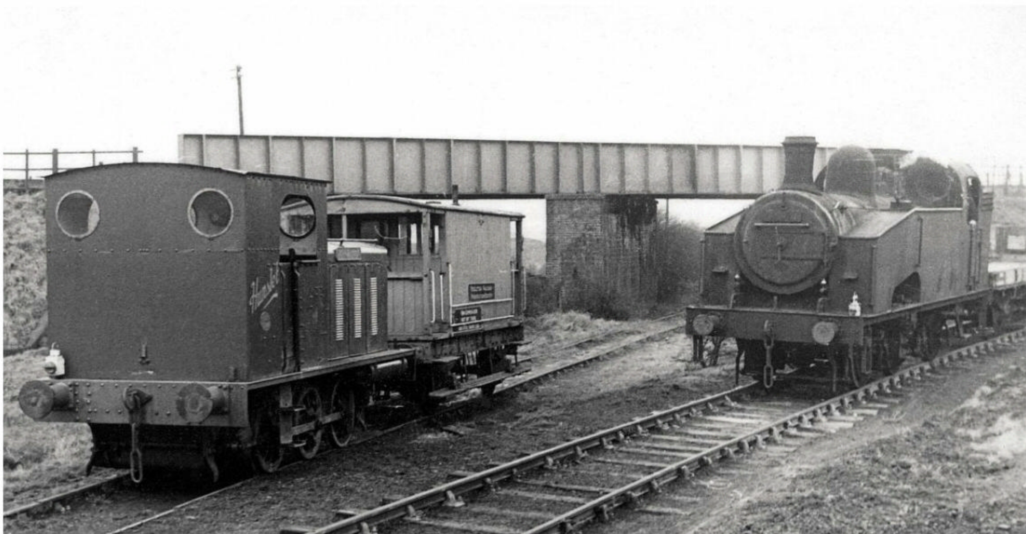
The volunteer-run freight operation saw up to three trains a day leave via the main line link, at first behind GNR J50 0-6-0Ts. Here, No. 1697 and the line's 'new' brake van are seen alongside Ardsley shed's J50 No. 68941 in January 1961. MRT COLLECTION
