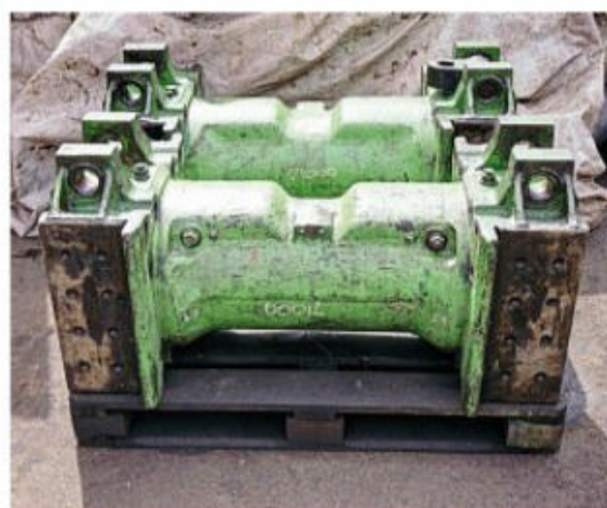
Above: Members of the team at Tyseley Locomotive Works have completed the welding up of the driving wheel bores. TREVOR TUCKLEY
