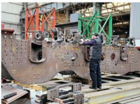
John Hind of ASTT works on Hengist 's frame stretchers. CLAN PROJECT
