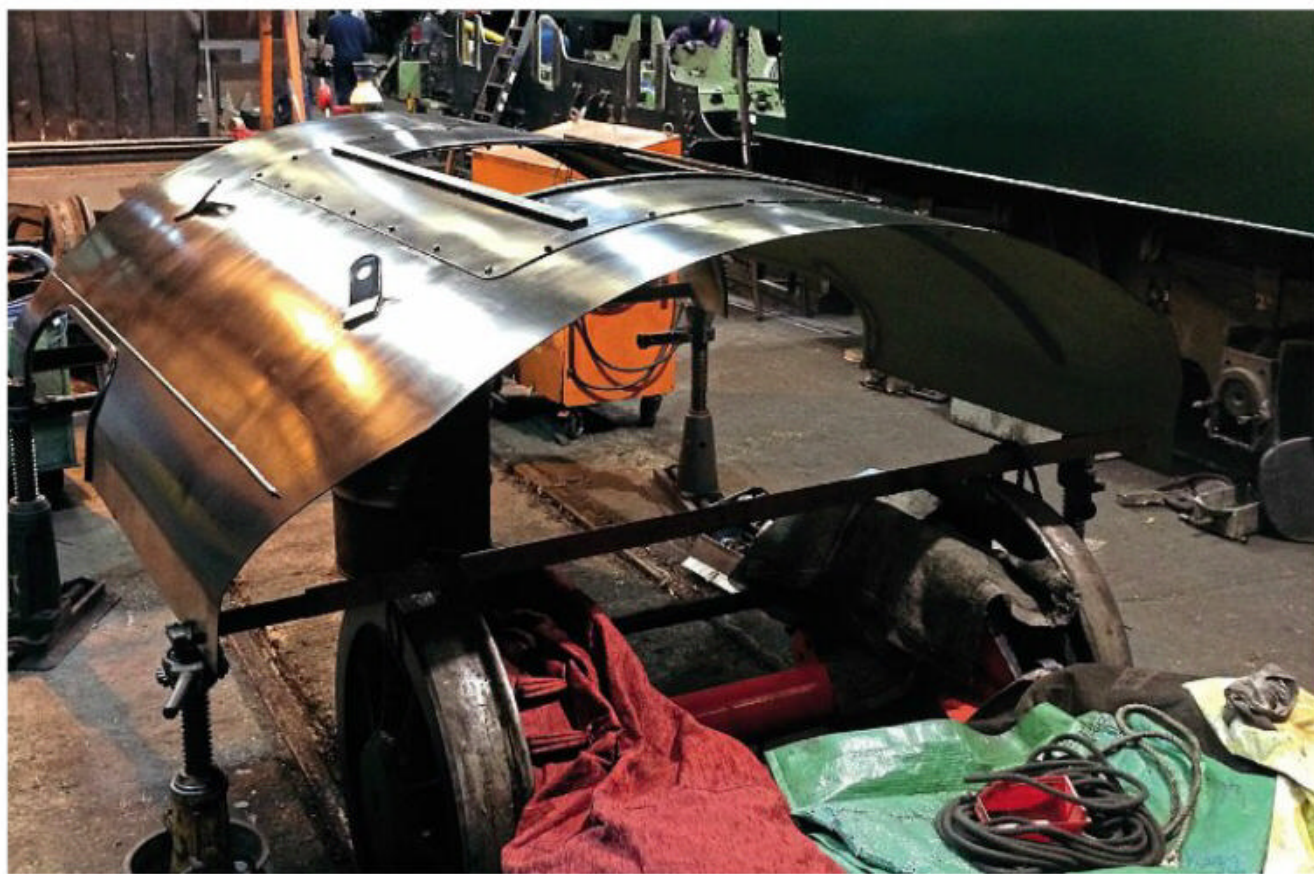
The locomotive's original cab roof disappeared during No. 80150's time at Barry scrapyard. Its replacement is seen at Ropley Works. MARTIN ORFORD
