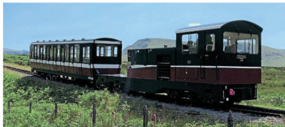
One of the newly-delivered Clayton diesel-battery hybrids, which has been given No. 14 in the Snowdon fleet. SMR
