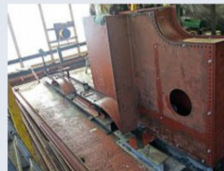
The construction of new tanks for GWR 0-6-2T No. 5668 is underway at Rolvenden works. KELVIN WILLIAMS
