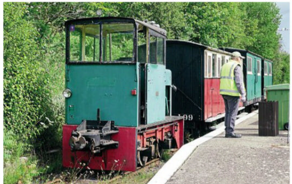
Hudson-Hunslet 4w DM No. 4182 of 1953 Victor ready to leave Kemsley Down on Sunday, July 5 with a works track clearing train. The leading coach, No. 199, is originally from the nearby Chattenden & Upnor Railway. SKLR
