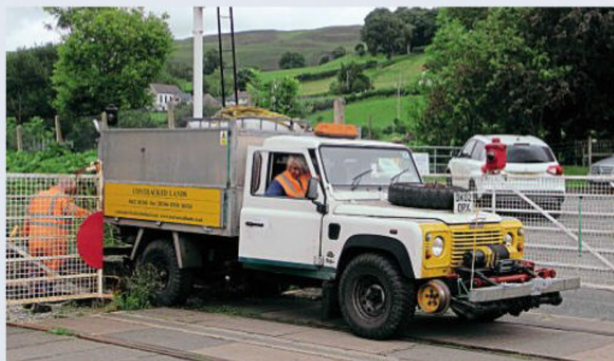
The Land Rover Defender road-rail vehicle is seen at Glyndyfrdwy level crossing, where it made a U turn to reverse direction. GEORGE JONES
