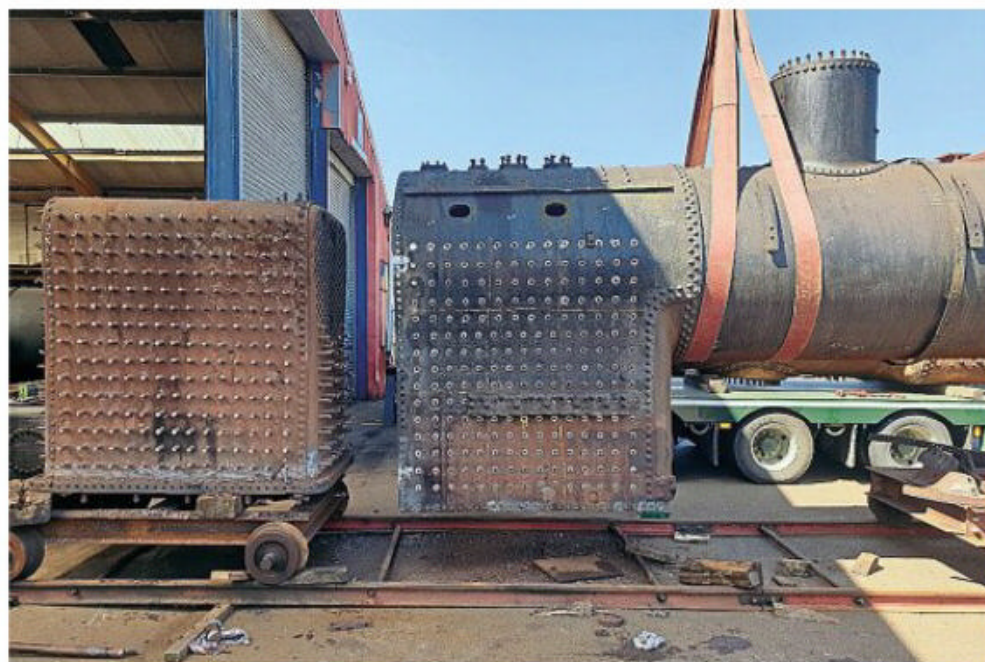
The old inner firebox for No. 65033 removed; copper sheeting for the new one is on order. LCLT
