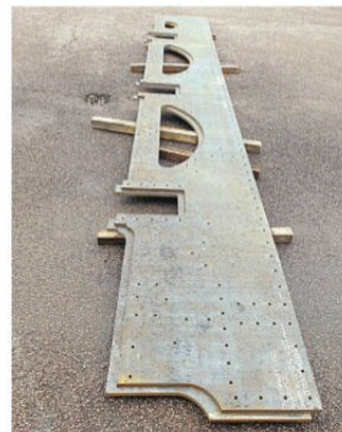
The new tender frame plates for the J21. LCLT
