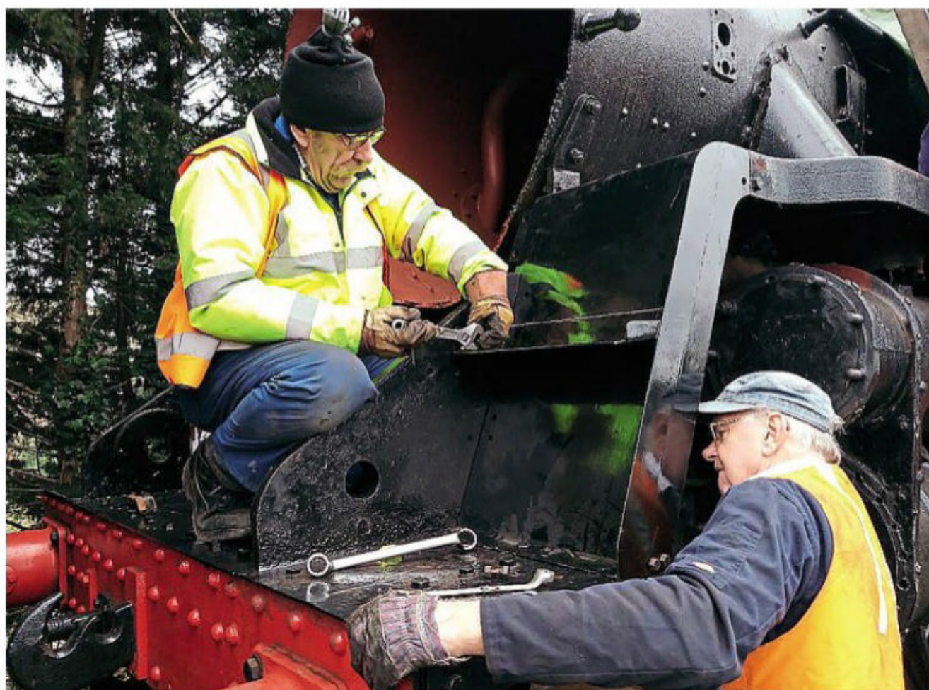
Tasks completed on the last working party on No. 80150 before the Covid-19 lockdown included refitting part of the running plate. Les Wateridge and Mike Savage are seen at work on March 17, 2020. RICHARD BRYAN
