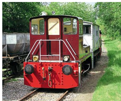
Left: Yorkshire Engine Company 'Half Janus' 0-6-0DE No. 1382, newly arrived in May 2019 following restoration to running order. RBR
