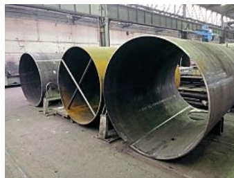
Conical boiler barrel sections for Tornado and Prince of Wales . CHRISTOPHER WÖRFEL, DBM/A1SLT
