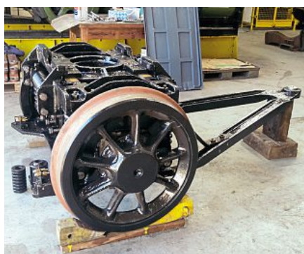
Above: The completed pony truck for BR Standard 4MT No. 76077. TSLL
