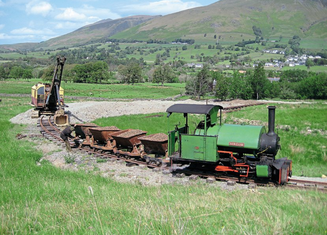
Bagnall 0-4-OST No. 2135 of 1926 Sir Tom heads a works train as Threlkeld Quarry and Mining Museum extends its current half-mile running line, aided by its collection of vintage machinery. TQMM
