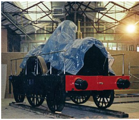
The non-working replica of pioneer GWR broad gauge 2-2-2 North Star was constructed for the 1925 Stockton & Darlington Railway centenary celebrations, using some of the parts of the original which had been scrapped in 1906. It is seen partially covered by a dustsheet during preparations to set up STEAM. SBC
