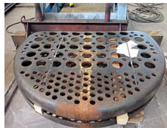
Firebox tubeplates for both locomotives. CHRISTOPHER WÖRFEL, DBM/A1SLT
