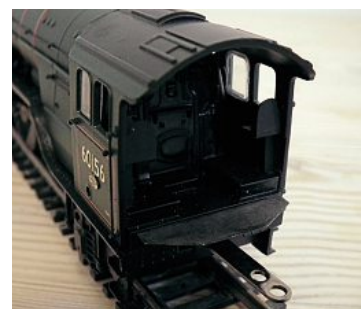
Firebox, cab and tender details are captured well, although the backhead of this original model features just rudimentary mouldings. PETE KELLY
