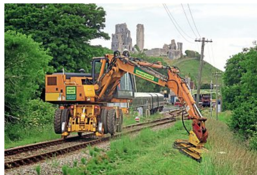
One of the Swanage Railway's two road-rail vehicles cuts embankment grass south of Corfe Castle station on June 9. This was the spot where British Rail's demolition contractors Eagre & Company of Scunthorpe started track lifting on the Swanage branch on Monday, July 10, 1972. ANDREW PM WRIGHT
