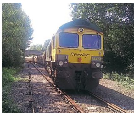
Class 66 No. 66414 setting back at Allerford Junction in preparation to discharge. The Freightliner shunter is proceeding on foot out of shot, all movements being controlled by radio communication with the driver. PAUL FLEET
