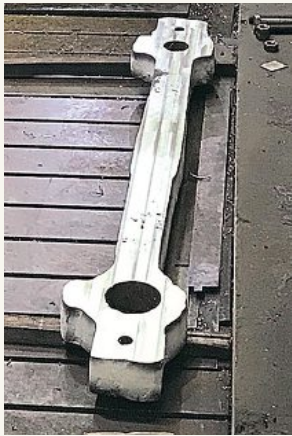
Coupling rod for No. 2007 on the straddle milling machine. STEPHENSON ENGINEERING LTD/ A1SLT
