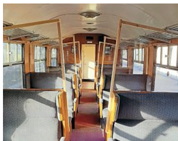
Hand-made by senior management, seating screening has been fixed into each Dartmouth Steam Railway carriage used for the comeback services. DSRRC
