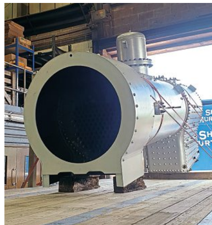
The second new boiler built by the Severn Valley Railway for the Isle of Man Railway's Beyer Peacock 2-4-0Ts was shipped out to its new owner on May 15, following the successful testing, official examination and approval earlier in the month. "Built by Severn Valley Railway Bridgnorth" is proudly displayed on the boiler barrel. The SVR is building five boilers for the IOMR, with the third to be completed later this year. JOSHUA HARVEY/SVR
