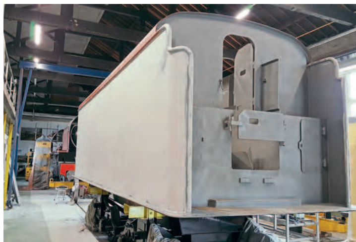
The fireman's side of the P2's tender tank ready to be primed. IAN MATTHEWS
