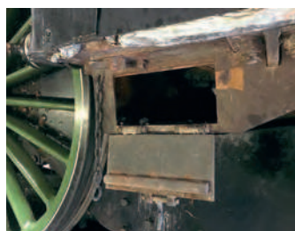
Tornado's ashpan side ash doors have been left open to allow the air to circulate. A1SLT
