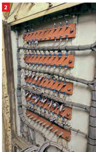
1. D5705's completed brake frame with new wiring being pulled through. C15PS
