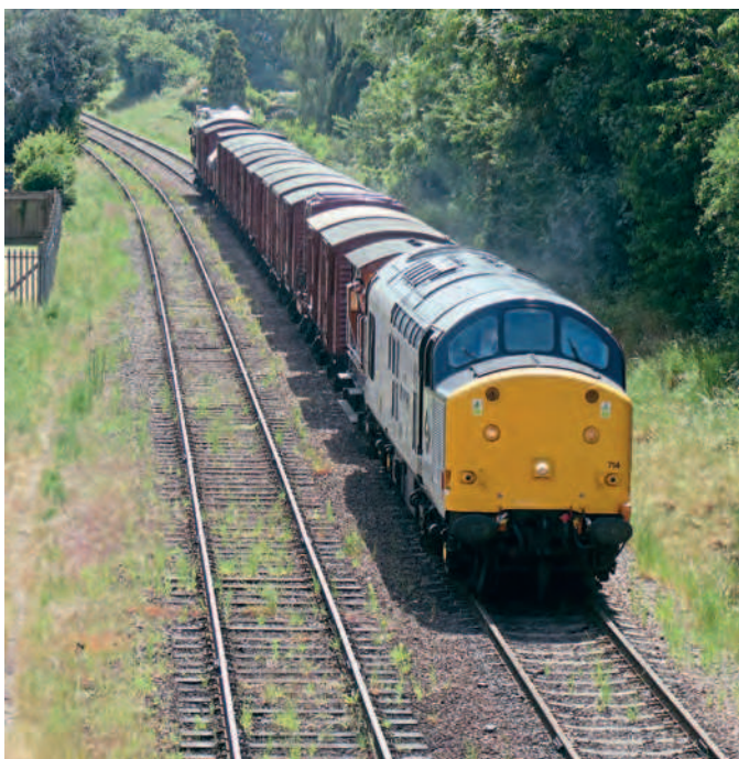
Above: Seconds after passing No. 78018 in the opposite direction, Trainload Freight (Metals)-liveried 1961-built Class 37 No. 37714 Cardiff Canton approaches Loughborough with a mixed freight rake primarily of box vans.
