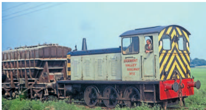
Then: During its latter operational days prior to closure in 1981, the Derwent Valley Railway's motive power was two Class 04 diesels bought from BR. One, formerly D2245, is pictured in September 1971 in its post-BR guise as DVR No. 2 on a freight train from York Layerthorpe, while a smartly-dressed gentleman surveys proceedings from the cab. DAVID TILLOTSON
