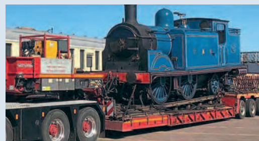
The trailer being used to carry the Scottish Railway Preservation Society's Caledonian Railway 419 class 0-4-4T No. 419. JJP HOLDINGS
