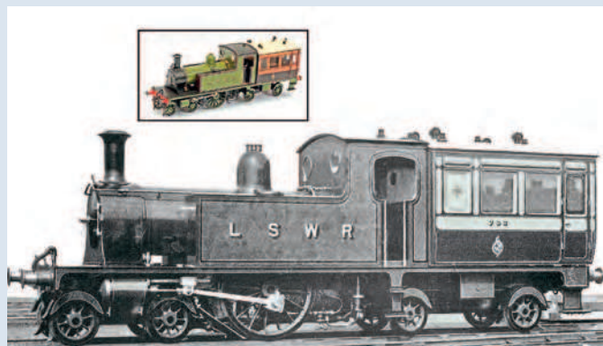
Drummond's transport: An official LSWR photograph of 4-2-4T and attached saloon nicknamed 'The Bug' which was built at Nine Elms in 1899 for the personal use of locomotive superintendent Dugald Drummond. CREATIVE COMMONS Inset: An O-gauge model of the unique locomotive and saloon combination that topped the model railway charts in a Vectis auction on April 30 with a realisation of £500. VECTIS AUCTIONS
