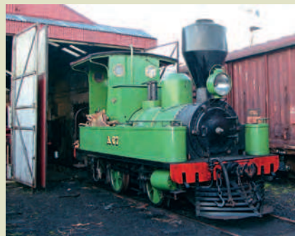
New Zealand Railways A class 0-4-0 A67 was built by Dubs & Co in Glasgow in 1873, and was bought by the Ocean Beach Railway in 1967. OBR
