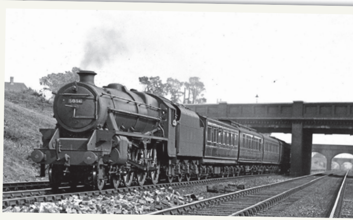
Note the period rolling stock as one of the original batch of 50 Stanier 'Black Five' 4-6-0s built by the Vulcan Foundry at Newton-le-Willows, Lancashire, in 1934/5. No. 5056 heads a 4.40pm London St Pancras to Bedford train near Mill Hill circa 1938. E R WETHERSETT/ RAILWAY MAGAZINE ARCHIVE
