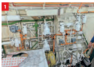
1. D5705's completed brake frame with new wiring being pulled through. C15PS
