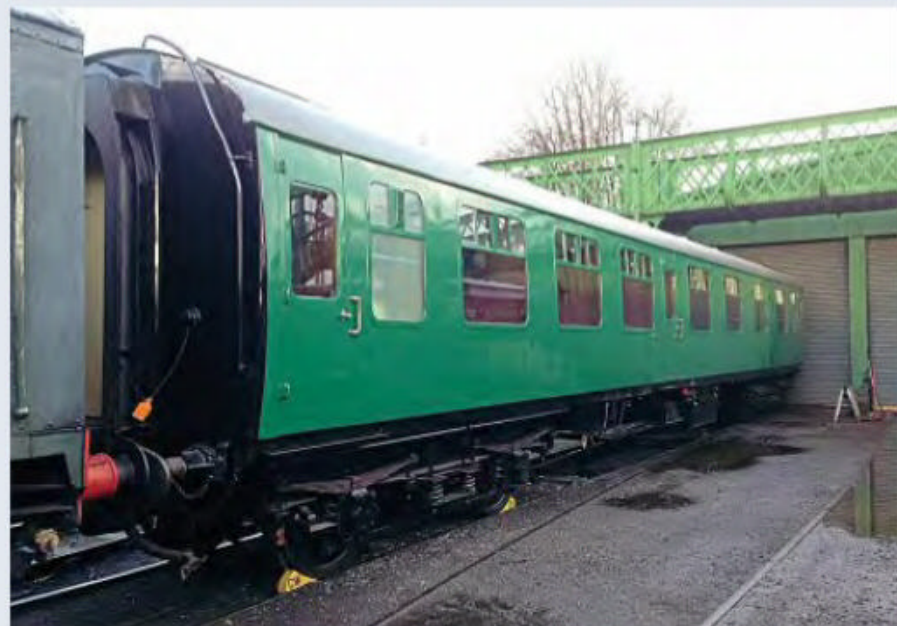
Mk.1 CK No. 16083 has been returned to as-new condition in the Ropley workshops. The carriage was built by Metro Cammell in 1959. MHR
