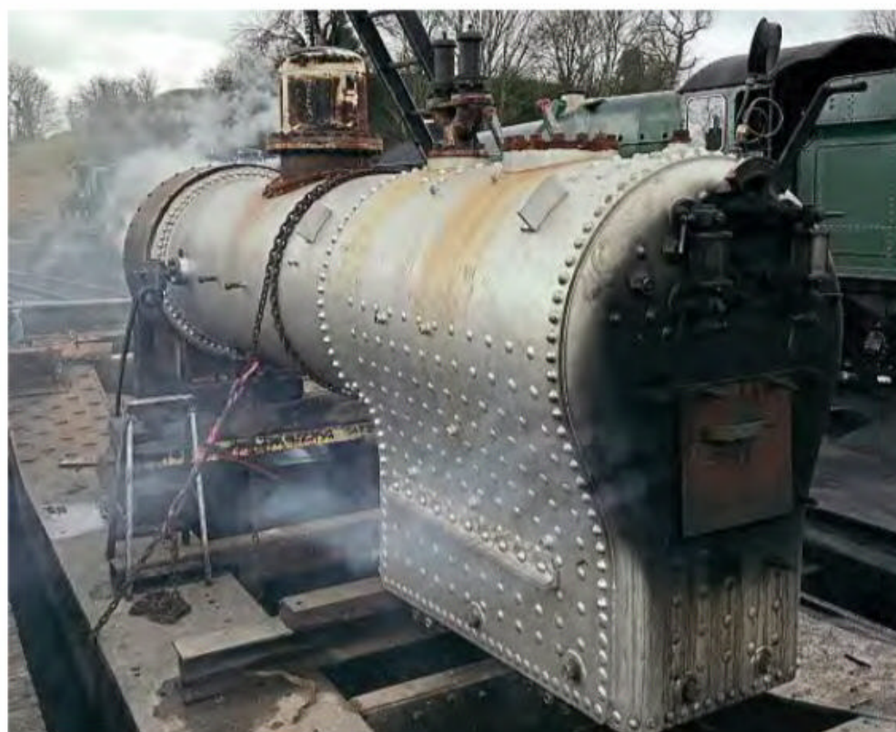
The first of five new boilers built by the Severn Valley Railway for the Isle of Man Railway (IoM) was steamed in Bridgnorth yard on March 7. This follows delays caused by an issue with the dome base design, which has now been rectified, meaning that two of the new-build boilers have been completed simultaneously rather than sequentially. The boilers, which will replace life-expired boilers in the IoM's fleet of Beyer Peacock 2-4-0Ts – originally built in the late 1800s – will first be fitted to No. 11 Maitland , whose bottom end overhaul is almost complete at Alan Keefe Ltd's works at Ross-on-Wye and go direct to Douglas for fitting to either No. 10 G.H. Wood or No. 12 Hutchison . The third boiler is also due for completion later this year and will be fitted to the other of No. 10 or 12, while the other two are on schedule for completion next year. PAUL APPLETON
