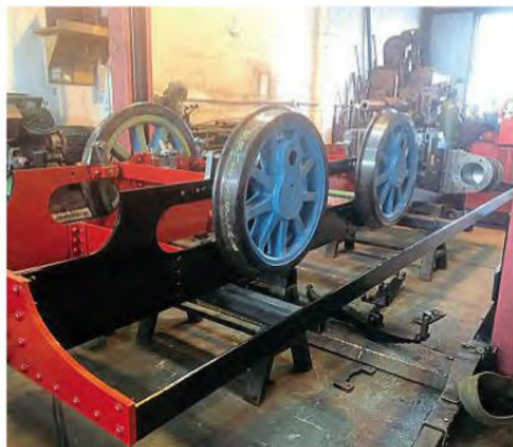
The wheels for the new Blyth fitted at North Bay Railway Engineering Services in Darlington. NBRES
