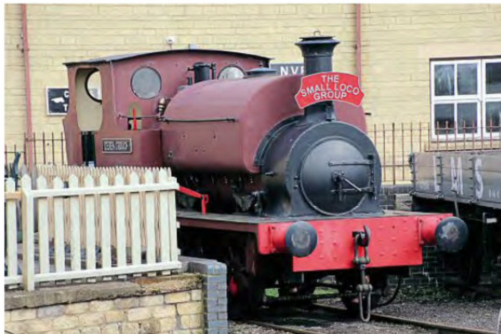
Currently serving as the footplate-accessible locomotive at Wansford, parts of Hudswell Clarke 0-6-0ST Derek Crouch have been labelled in readiness for stripping. The 1924-built engine is seen on March 14 – the headboard being a reminder of the team of younger volunteers who will carry out its return to steam. GARETH EVANS
