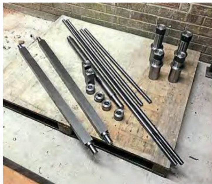
A brake part and crank pins for replica Sharp Stewart 2-4-0T Blyth . NBRES
