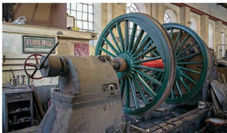
Above: One of the T3 driving wheelsets on the Flour Mill lathe for thrust face machining and journal polishing. 563LG
