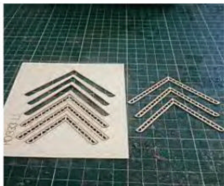
The laser-cut barge boards are a delicate work of art, and when fitted add lots of period charm to the building.
