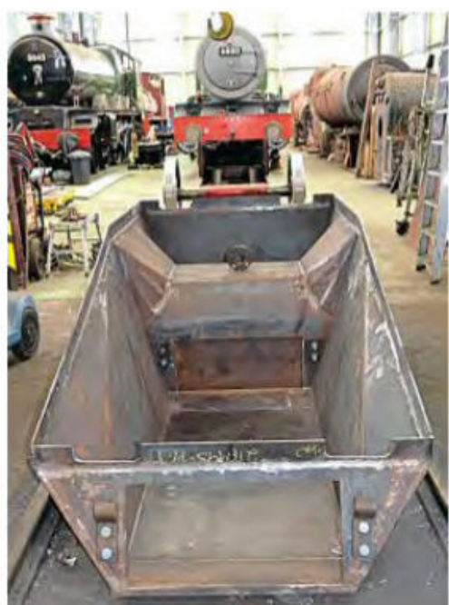
The new ashpan for No. 6880 Betton Grange , prior to fitting on March 18.
