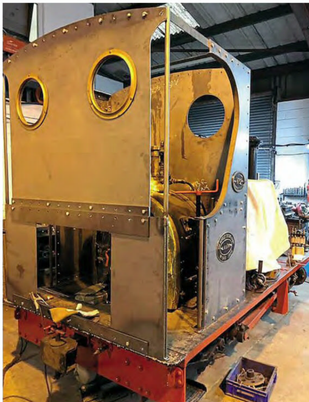
The new cab built for Llanberis Lake Railway Hunslet 0-4-0ST Thomas Bach , also known as Wild Aster . NBRES
