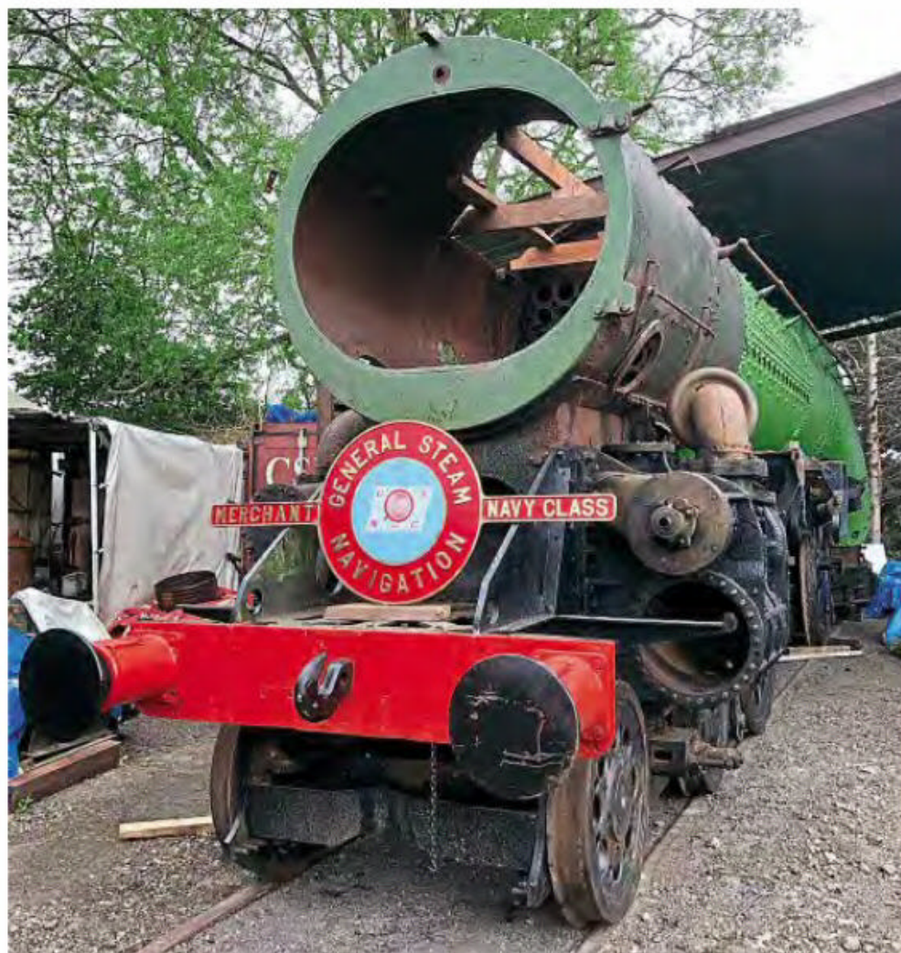
Bulleid Merchant Navy Pacific No. 35011 General Steam Navigation now at Blunsdon needs a boiler life to pave the way for the next stages of its restoration and back-conversion to original condition. GSNLRS
