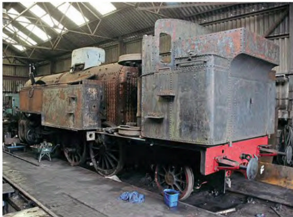
Swedish State Railway 2-6-2T No. 1178 is seen inside the running shed at Wansford on March 23, 2019. The boiler and tanks are loosely fitted to the frames. GARETH EVANS
