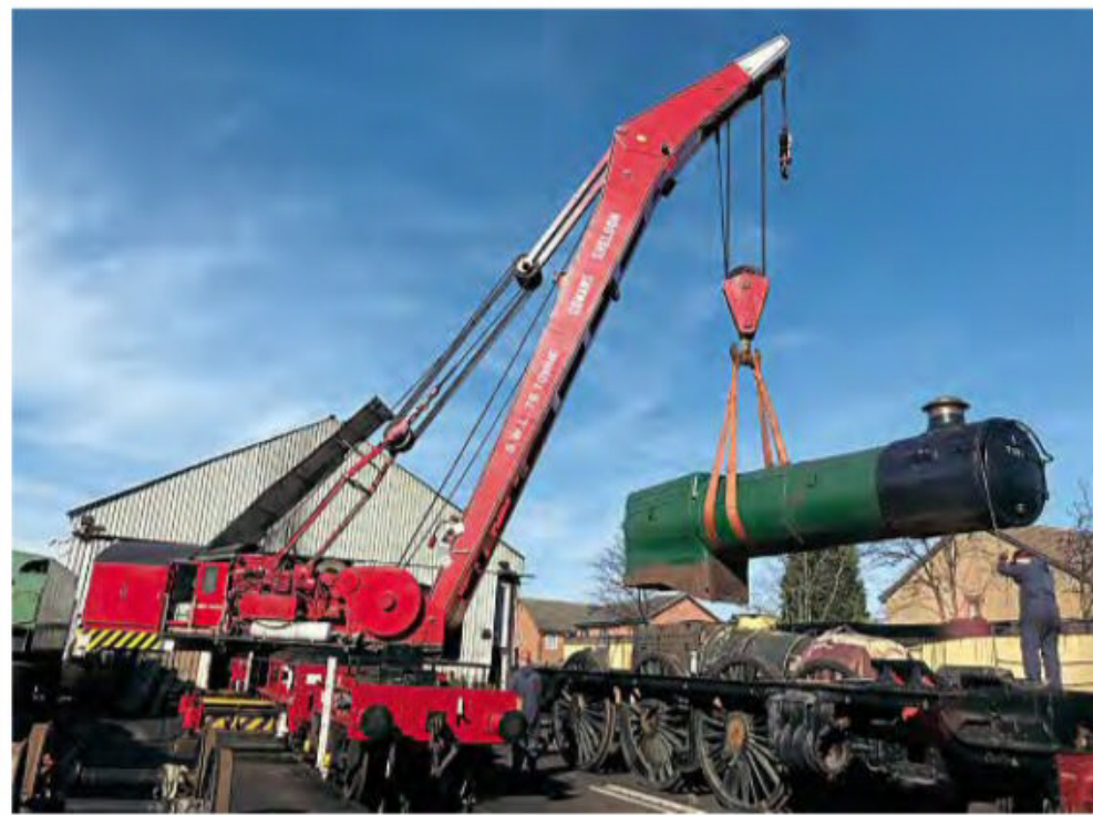
THE boiler of WR 4-6-0 No. 7027 Thornbury Castle was lifted at the Great Central Railway's Loughborough Works on March 23. Meanwhile, the team carrying out the restoration has appealed for spare parts. Anyone who might have a suitable GWR boiler pressure gauge (measuring up to 320psi), GWR steam heat pressure gauge, oil gauge for the cylinder lubrication or safety valve bonnet is asked to make contact via www.facebook.com/7027-Thornbury-Castle-114458853436676 CRAIG STINCHCOMBE
