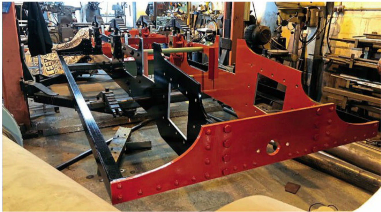
Above: A replica of Sharp, Stewart 2-4-0 No. 3 Blyth is under construction at North Bay Engineering Services Ltd. The locomotive’s frames are seen freshly painted on January 11. NBES
