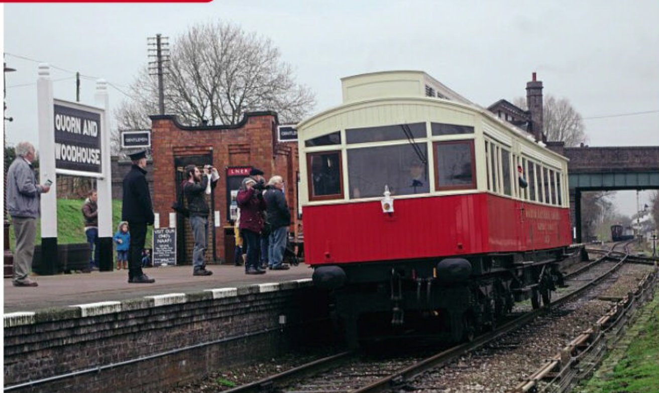
Making its inaugural visit in service to a heritage line away from its Embsay & Bolton Abbey Steam Railway home was NER petrol-electric autocar No. 3170, the world's first internal-combustion passenger vehicle. Working its first service on the GCR, the 11.05 from Loughborough to Leicester North on January 25, it is seen stopping at Quorn & Woodhouse. ROBIN JONES
