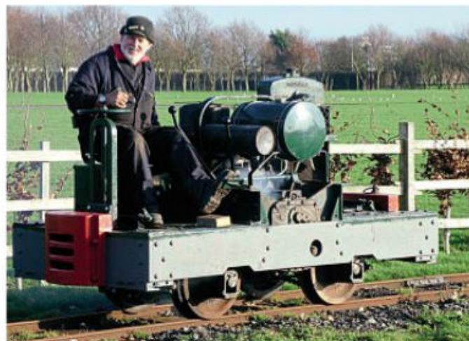
Simplex No. 9264 of 1947, which was swamped in the 1953 East Coast floods at Mablethorpe and later used in brickworks there and in Skegness, is seen undergoing testing in January as part of its restoration to working order. CHRIS BATES/LCLR
