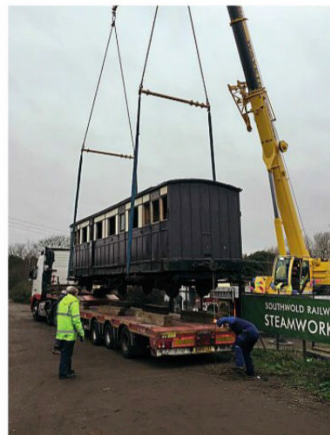
Manx Northern Railway carriage No. 3 is seen on arrival at Steamworks on January 7, 2019. The 1879-built vehicle, which shares the same Cleminson three-axle system as the original Southwold Railway carriages, is being preserved as a museum piece for now. SRT
