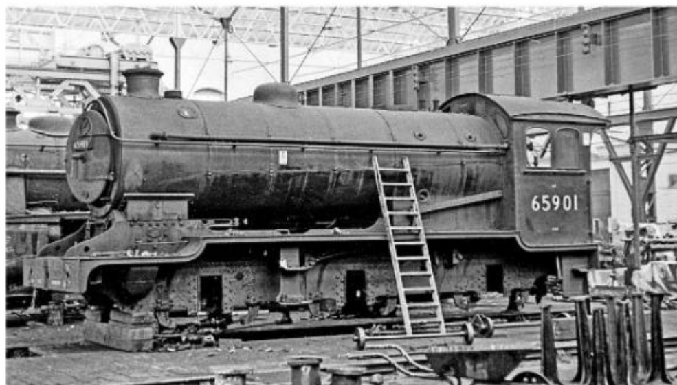
The full works: LNER J38 class 0-6-0 No. 65901 undergoes overhaul at Inverurie Works in 1964. The entire Nigel Gresley-designed class of 35 locomotives was based in Scotland, nearly half of them allocated to Thornton Junction (62A), including No. 65901, which was built at Darlington in January 1926 and was one of the last to be withdrawn, in April 1967. TRANSPORT TREASURY/NORRIS FORREST
