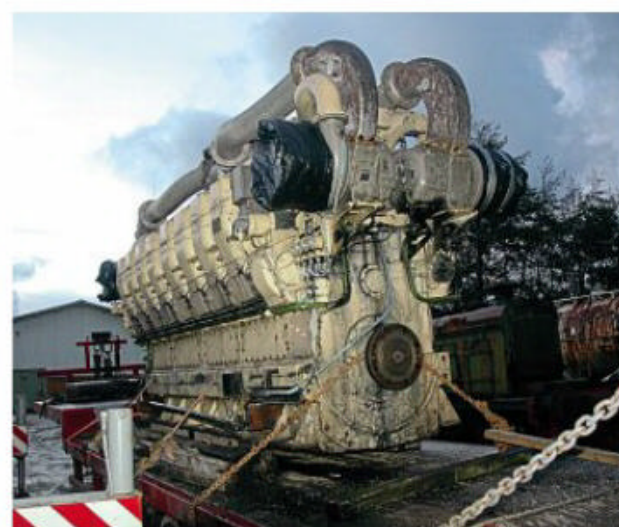
The Ivatt Diesel Re-creation Society's 16SVT engine seen during a previous lift. IDRS
