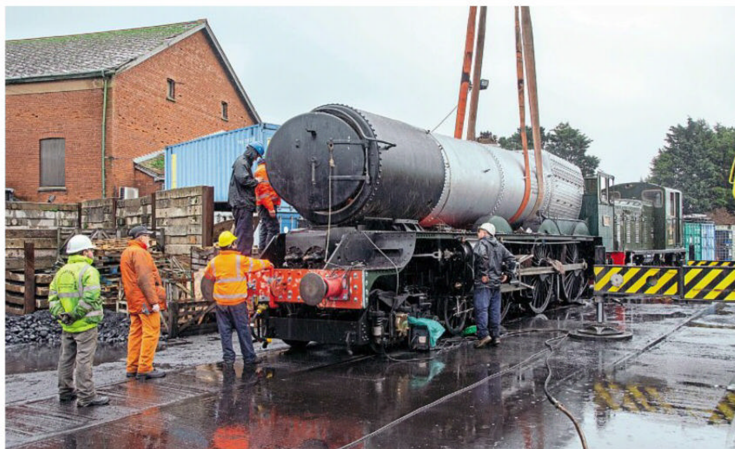
The boiler of No. 6024 King Edward I was reunited with the frames at Minehead on January 9, after slight adjustment to the newly-fabricated ashpan. MARTIN BANE / 6024 SOCIETY
