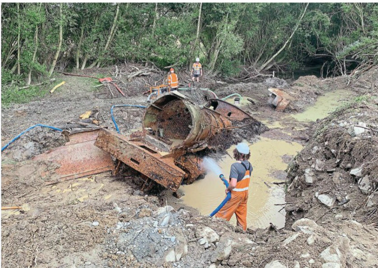
Workers blast 93 years of silt from No. 127 before craning it out of the riverbed mud. LUMBSDEN HERITAGE TRUST
