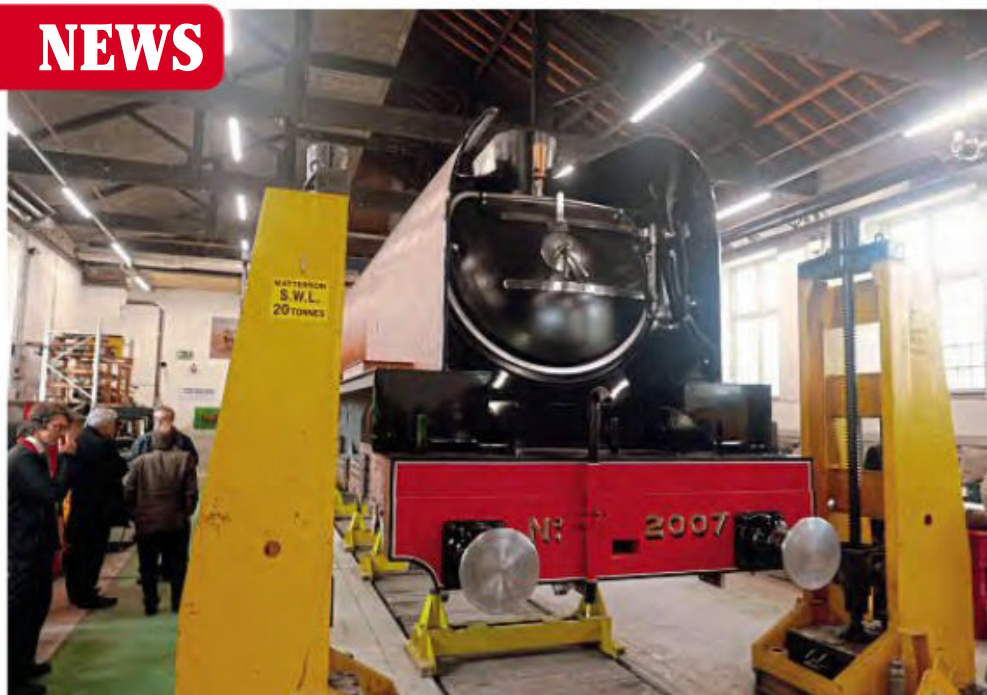
New P2 2-8-2 No. 2007 Prince of Wales under construction in Darlington on June 15, 2019. The plans for the new Rail Heritage Quarter include the possibility of a new home for builder The A1 Steam Locomotive Trust with public viewing facilities and a main line connection. ROBIN JONES
