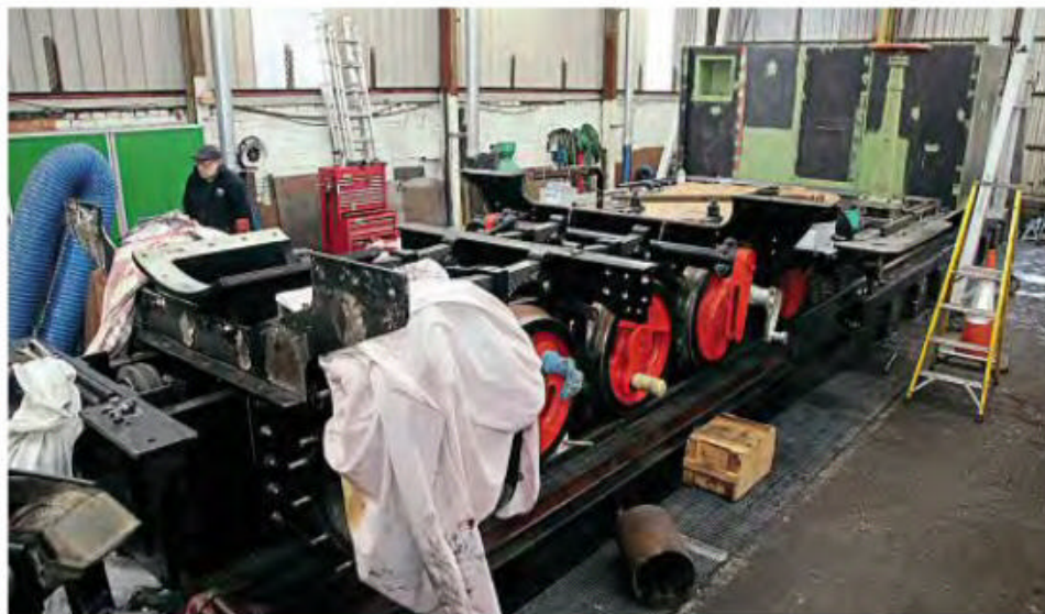
Sir Drefaldwyn is seen inside Llanfair's workshop on December 28. The new handbrake and coal bunker are readily apparent. GARETH EVANS
