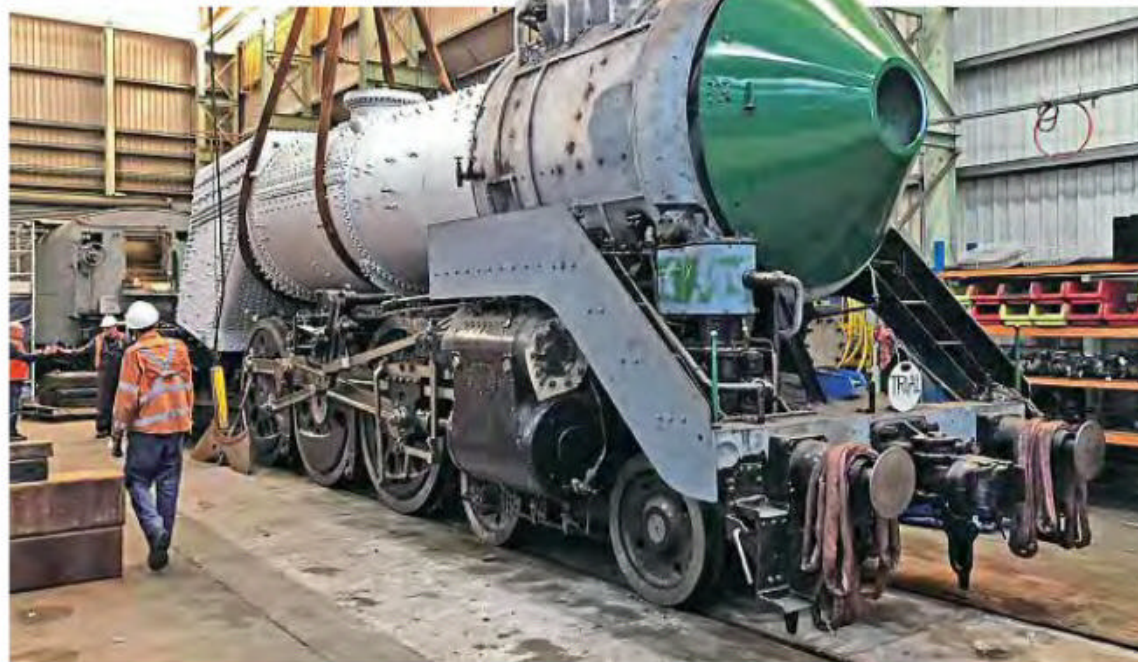
Reunited at last: The overhauled boiler of NSW Government Railways' No. 3801 is reunited with its frames in a test fitting at the Chullora works near Sydney in early July, nearly 12 years after the controversial restoration of the flagship streamlined Pacific was started. TRANSPORT HERITAGE NSW/ STEVE BURROWS
