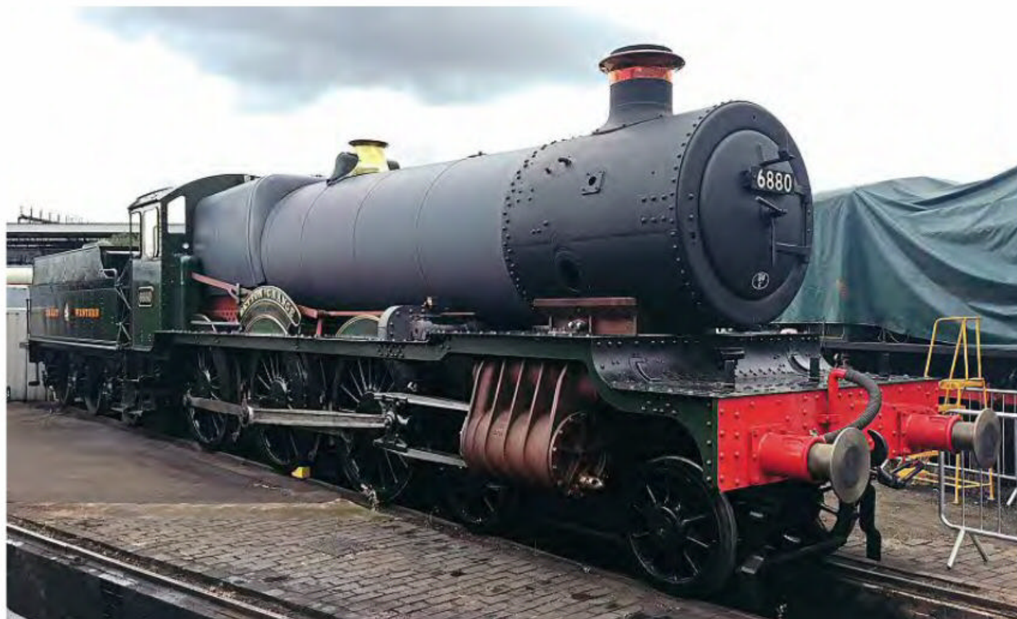
Aiming for a main line future: new GWR 4-6-0 No. 6880 Betton Grange at the Tyseley Locomotive Works open weekend of June 2017, with the boiler from No. 5952 Cogan Hall in the frames and a borrowed 28XX tender. QUENTIN MCGUINNESS/6880
