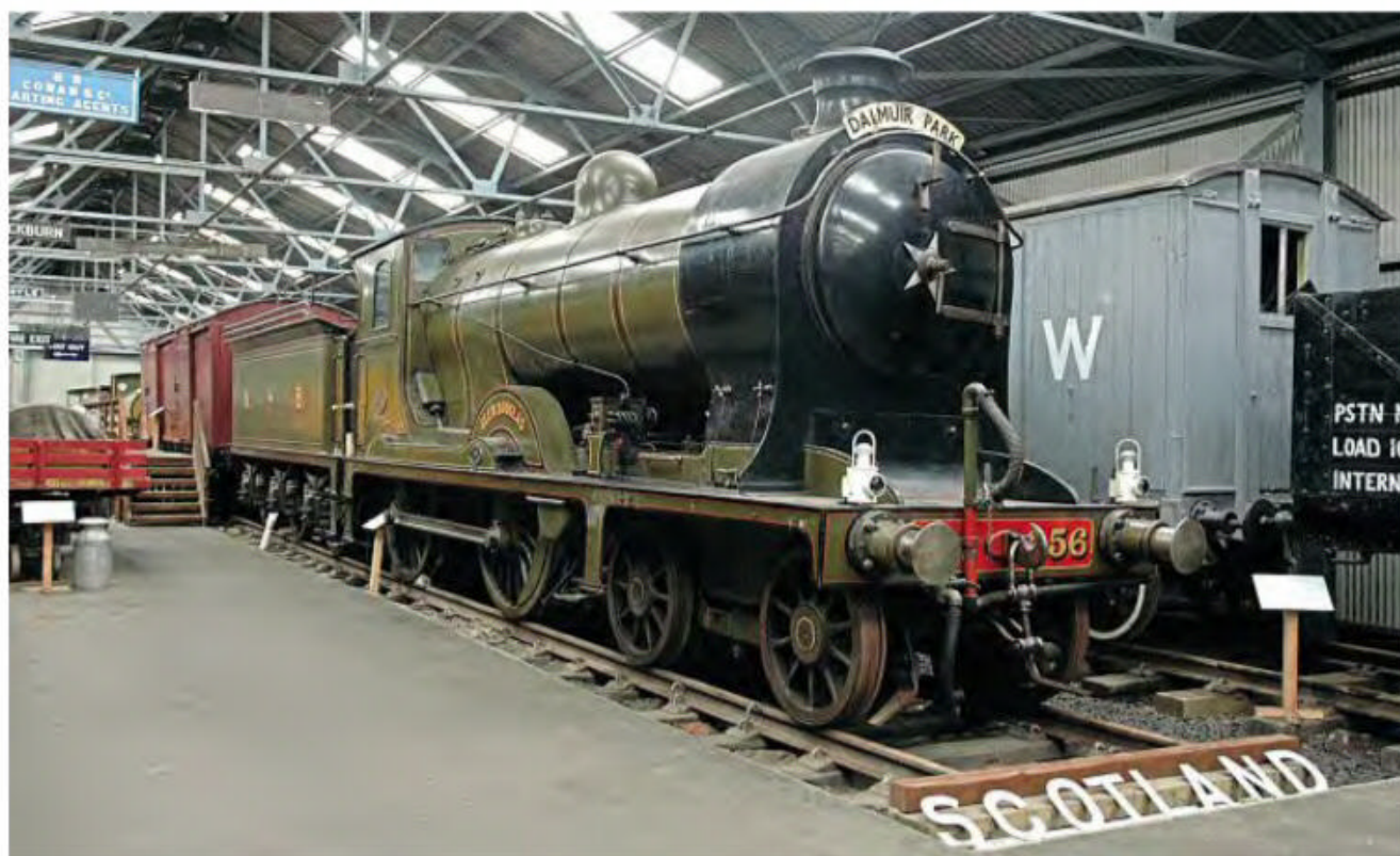
North British Railway K class 4-4-0 No. 256 Glen Douglas was designed by William Reid and built in 1913. No Reid Atlantic survives but the 4-4-0 features the large boiler following the example set by McIntosh on the Caledonian Railway with his Dunalastair 4-4-0. BRIAN SHARPE
