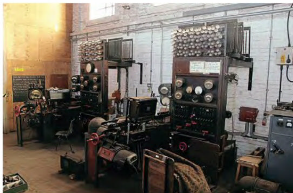
Kidderminster carriage works is home to dynamo and regulator test rigs of LNER origin, rescued from Wolverton Works. The lucky survivors date from 1898. GARETH EVANS
