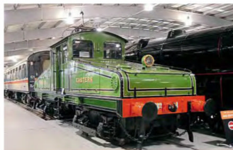
Right: North Eastern Railway Bo-Bo electric No. 1, built by Brush and British Thompson Houston in 1905 for the electrified Quayside branch on Tyneside, on display in the Locomotion museum at Shildon. BRIAN SHARPE
