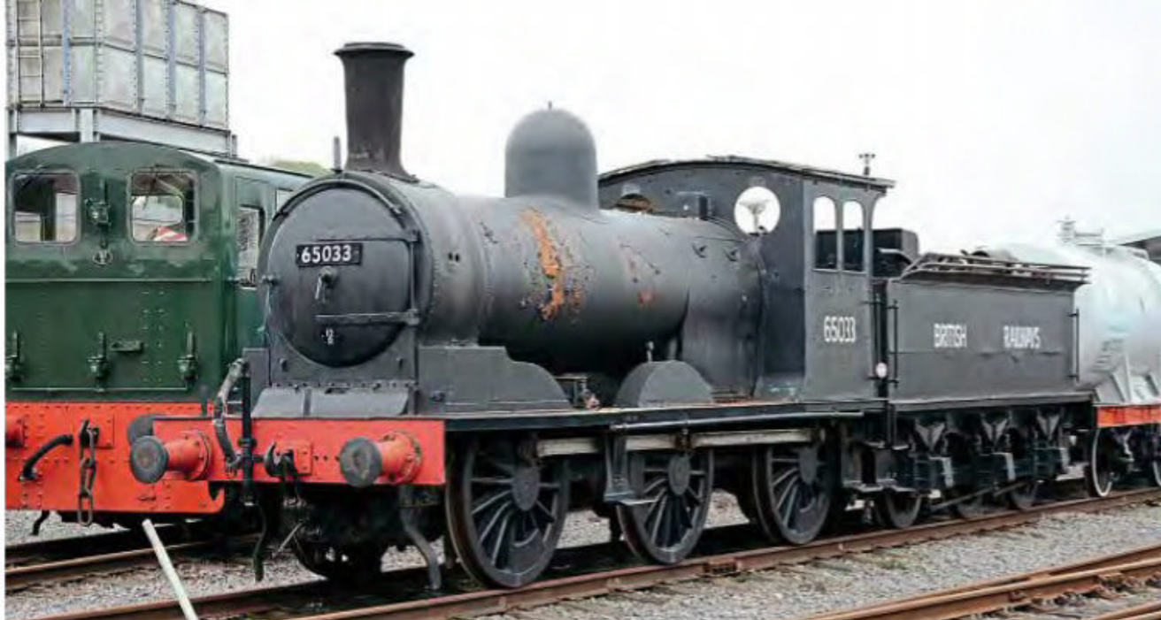
NER C class 0-6-0 No. 876, designed by William Worsdell and built in 1889, on display at Locomotion. Originally built as a compound, the engine was rebuilt as a simple 0-6-0 after William’s brother Wilson Worsdell took over as the NER’s locomotive superintendent. BRIAN SHARPE
