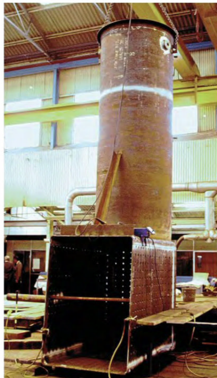
The boiler and the firebox following manufacture. VT
