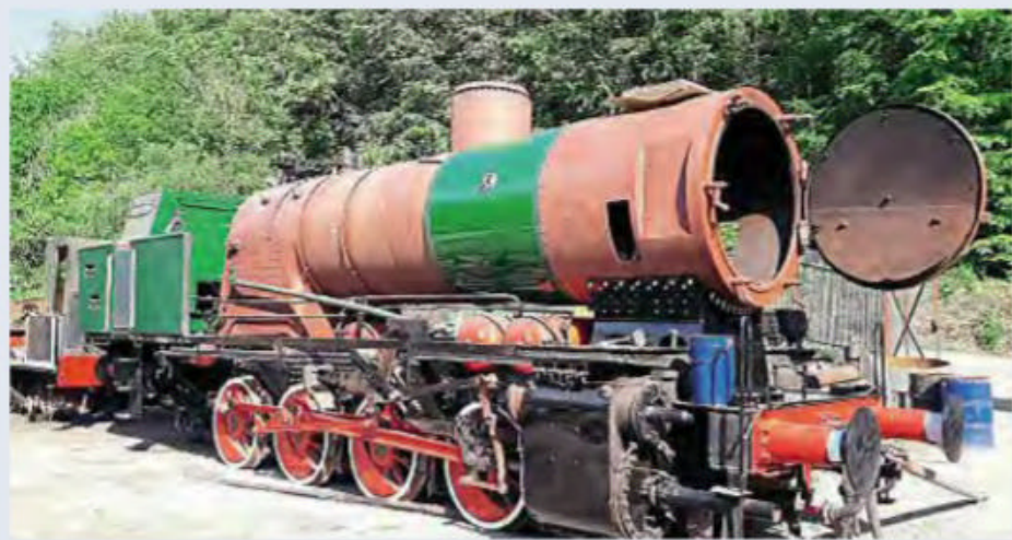
Polish TKp 'Slask' 0-8-0T No. 5485 with its new boiler at the Flour Mill workshop at Bream. FLOUR MILL
