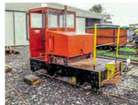
Motor Rail Simplex T3, now part of the Lincolnshire Coast Light Railway fleet. MIKE NEWBOLD/LCLR
