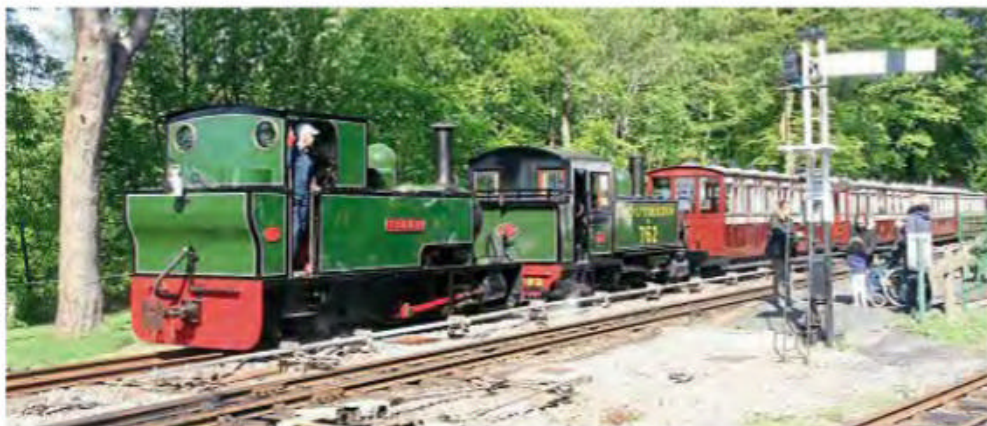
Right: Bagnall 0-4-2T Isaac , back in Lynton & Barnstaple service for the first time after many months' extensive work, double-headed the first and last trains on both days with Lyn . Built in 1952 for the South African platinum-mining industry, Isaac is privately-owned but permanently based on the L&B.
