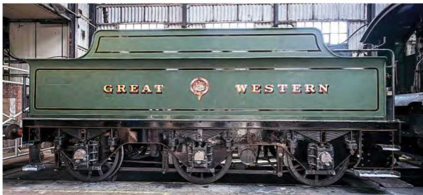
Signwriter Jon Leeson spent two weeks lettering and lining new Saint 4-6-0 No. 2999 Lady of Legend , pictured is one tender side with garter crest. The lettering might appear off centre, but that is deliberate as the practice of the period to which No. 2999 has been restored was to line up the crest with the centre axlebox. The locomotive is scheduled to be unveiled in all its glory over Didcot Railway Centre's June 7-9 weekend when No. 7903 Foremarke Hall is visiting and will be running all three days with the Saint. No. 7903, as one of the Modified Halls built after the Second World War, is the final development of 4-6-0s carrying the Swindon No. 1 boiler which was first fitted to Churchward's Saints. FRANK DUMBLETON
