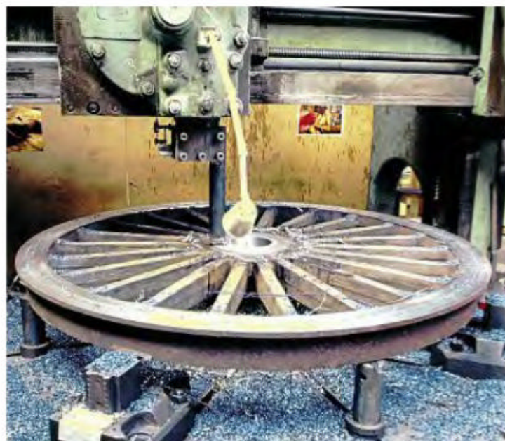
The 7ft driving wheel of the new Bloomer being machined. VT
