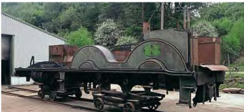
The chassis of No. 563 outside the Flour Mill workshop on May 17 following its exploratory dismantling. NICK LLOYD
