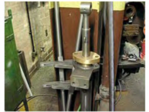
New non-ferrous components for the motion of No. 670 waiting to be fitted in the Tyseley workshops. ROBIN JONES
