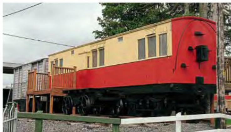
Coach No. 28 on display outside Donegal Railway Heritage Centre in August 2012. The paintwork was masking body decay. HUGH DOUGHERTY
