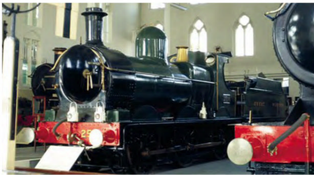
NER C class 0-6-0 No. 876, designed by William Worsdell and built in 1889, on display at Locomotion. Originally built as a compound, the engine was rebuilt as a simple 0-6-0 after William’s brother Wilson Worsdell took over as the NER’s locomotive superintendent. BRIAN SHARPE
