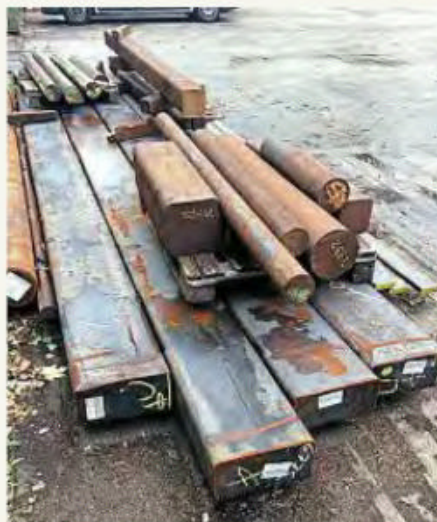
The blooms for the P2 heavy motion await forging at Stephenson Engineering. A1SLT
