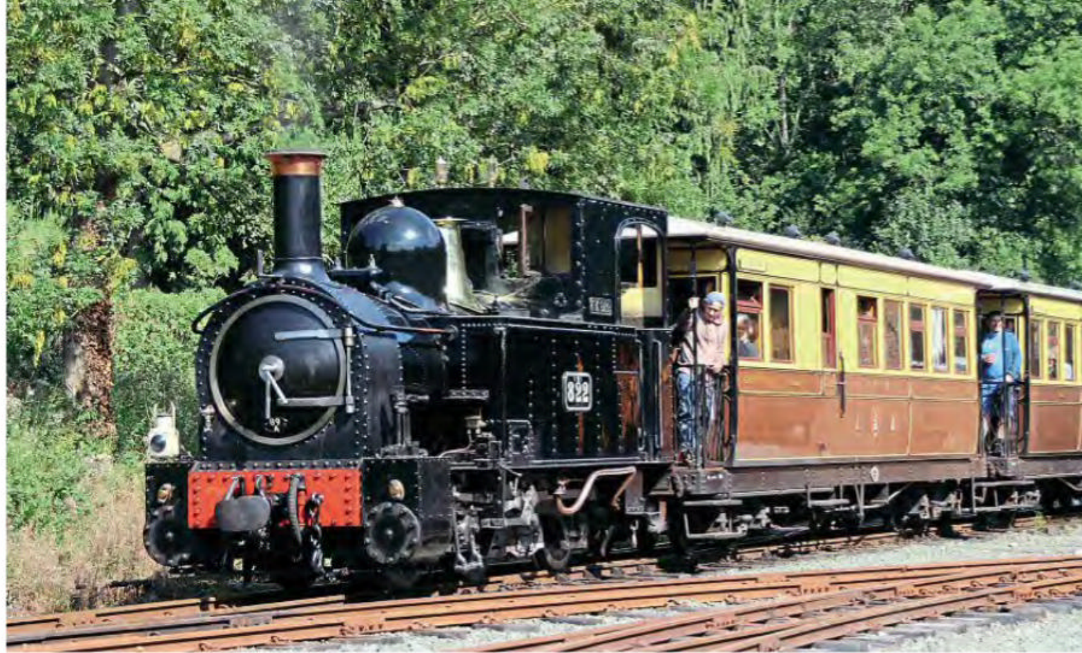
Beyer Peacock 0-6-0T The Earl departs Welshpool Raven Square on August 31, 2018 with the line's replica Pickering carriages. One of the line's two surviving original locomotives, the 1902-built machine is now to be overhauled in another part of the GWR narrow gauge empire – the Vale of Rheidol at Aberystwyth. GARETH EVANS
