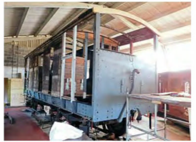
Jumbo the brake van being rebuilt so that it will soon be able to offer passenger rides. LWR
