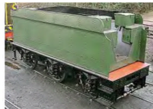
The newly-fitted tender tank and rewheeled chassis on No. 4930 Hagley Hall 's tender. FRIENDS OF HAGLEY HALL
