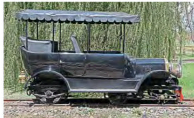
A railcar constructed at Sandstone from a 1913 BSA car body.
