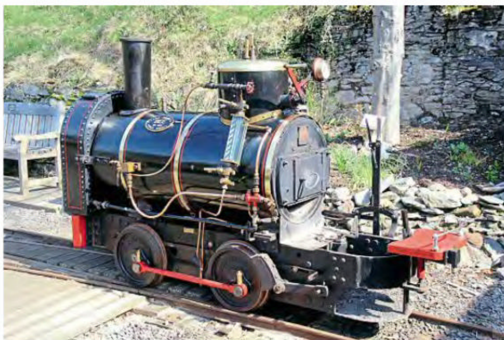
The Great Laxey Mines Railway operates two distinctive-looking replica Lewin 0-4-0s. Bee is seen on April 9. The smokebox is emptied at the end of each season. The water tank is mounted in front of the chimney. GARETH EVANS
