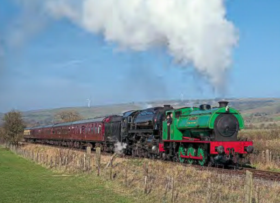
On loan from the Foxfield Railway, former NCB Hunslet Austerity 0-6-0ST No. 3694 of 1950 Whiston pilots S160 No. 5197 en route to Ipstones on February 23. DAVE GIBSON
