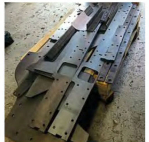
Various pieces of the running plate built by Keyte Smith Ltd which will be fitted around the front of Prince George . GFSLT
