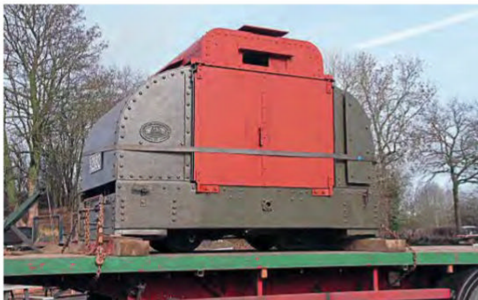
Armoured Simplex No. LR2182 newly delivered to the Leighton Buzzard Railway with its First World War cupola roof and steel protective doors permanently renewed. CLIFF THOMAS/GREENSAND RAILWAY MUSEUM TRUST
