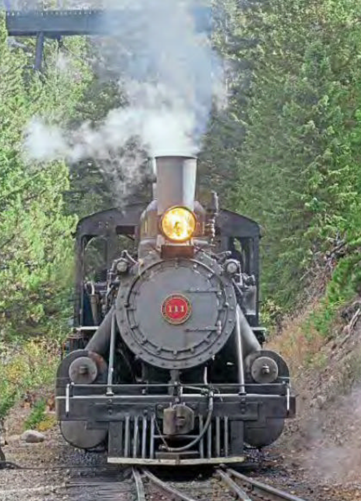
Baldwin-built No. 111 is currently one of two working steam locomotives on the Georgetown Loop Railroad. The 4.5-mile line ascends an elevation of 640ft, the 2-8-0 is seen at Georgetown October 2.
