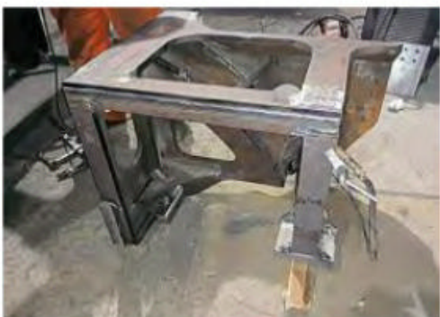
The P2's outside motion brackets have been made by North View Engineering Solutions in Darlington. A1SLT
