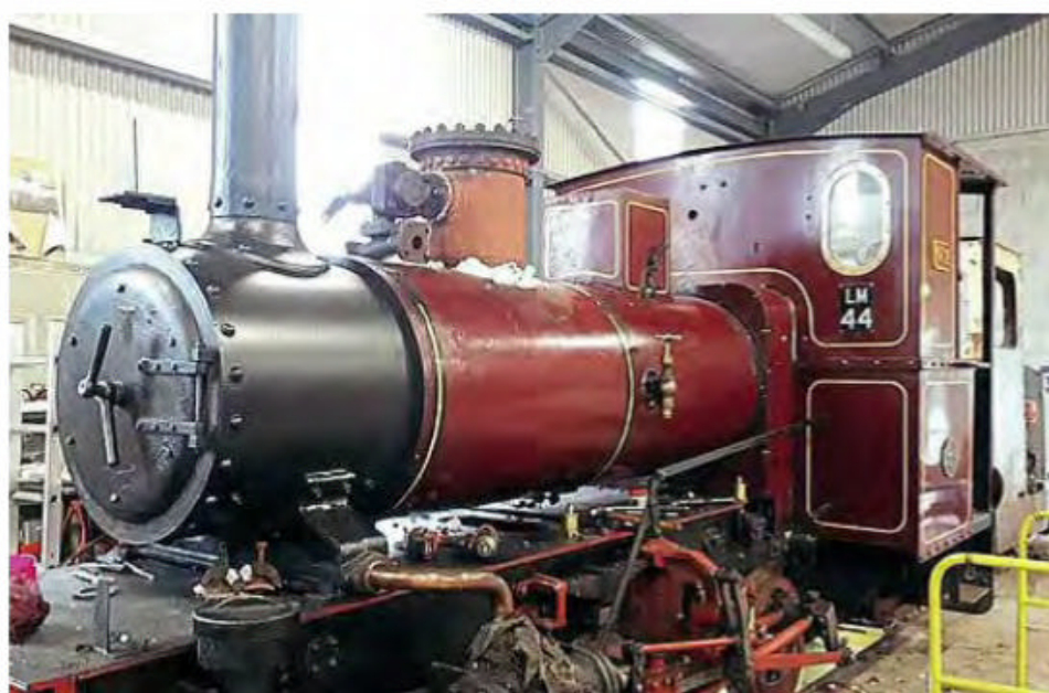
No. LM44 undergoing the last stages of its overhaul by the Stradbally Woodland Railway locomotive department on February 24. SWR
