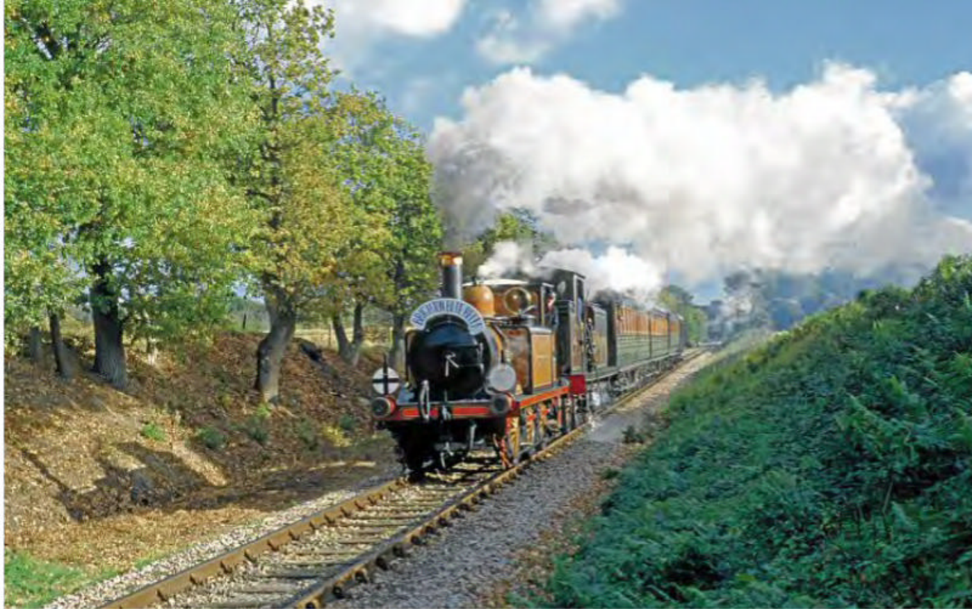
London Brighton & South Coast Railway Stroudley A1X 0-6-0T No. 55 Stepney of 1872 on the Bluebell Railway in Stroudley's 'improved engine green' livery on Freshfield Bank. BRIAN SHARPE
