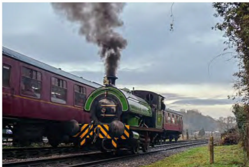
After an absence of many years, smaller engines have recently joined the NYMR fleet. The unsung hero of the 2018 Santa trains was Robert Stephenson & Hawthorns 0-4-0ST (7063/1942) No. 15 Eustace Forth which was employed on steam heating duties at Pickering. The former CEBG locomotive was resident on the line for a short time from 1972. TOM HOUSEMAN
