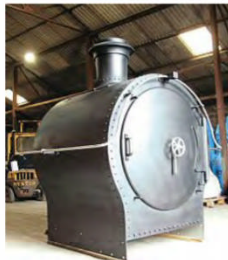
The completed smokebox for Prince George with the handrail in place. GFSLT
