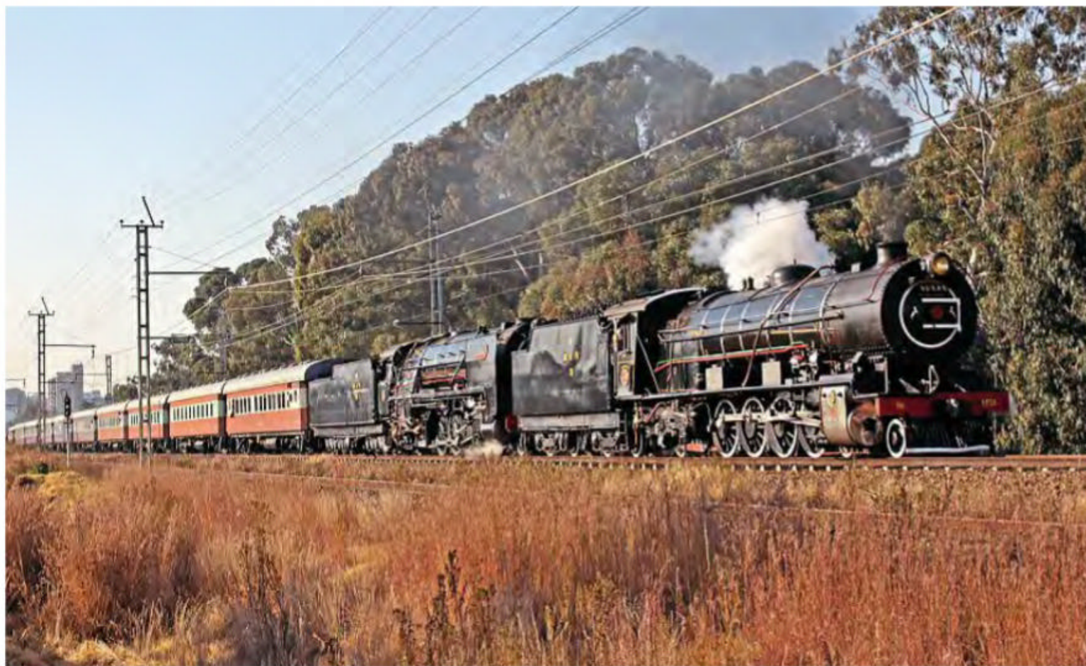
British power: Class 12AR No. 1535 (leading) and Class 15F No. 3046 double-head South Africa's 'Magaliesburg Express' on June 23, 2018. The two 4-8-2s, built by North British in 1919 and 1945 respectively, are producing a combined 84,180lb lb ft tractive effort as they climb the bank towards Hamberg west of Johannesburg. The train, one of the few remaining regular steam trips in the country, has been suspended after a row between its operator and South Africa's rail network company. GRAHAM MCWILLIAMS
