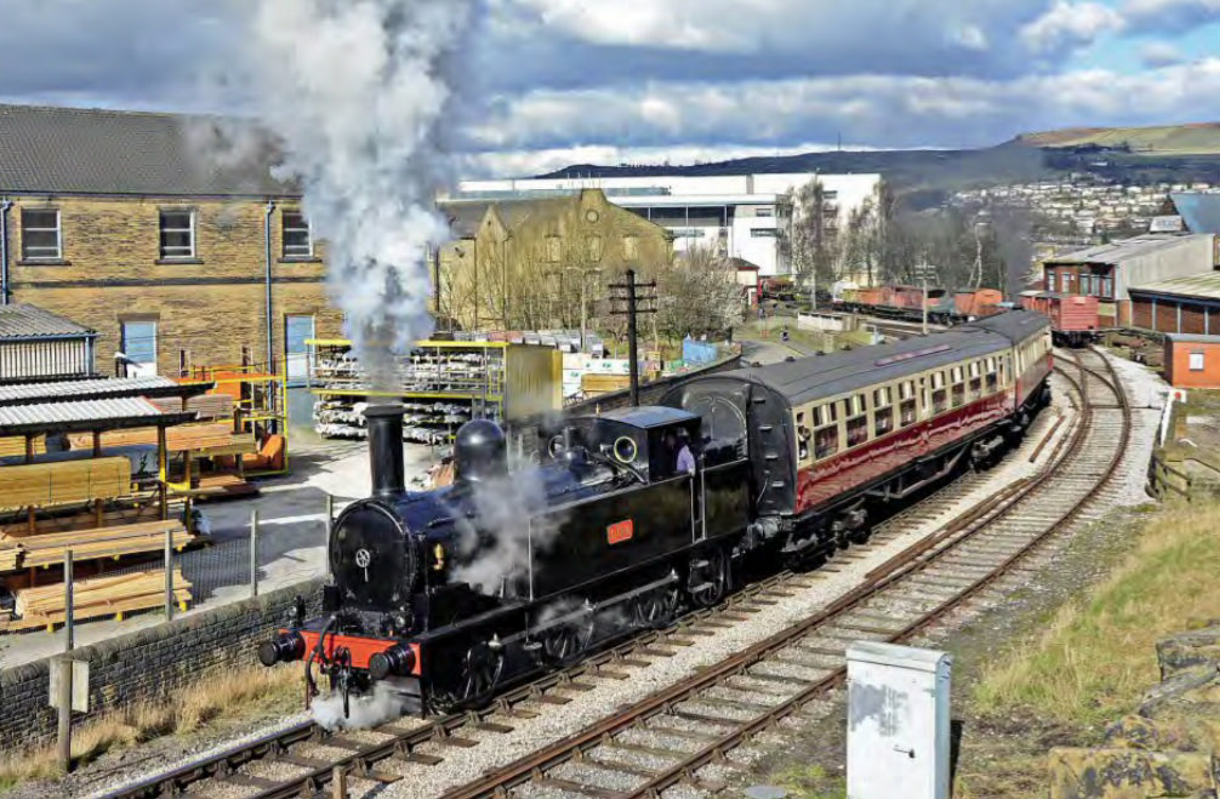
Above: Francis Webb's first locomotive design for the London & North Western Railway was the Coal Engine 0-6-0 in 1873. In 1882 he introduced an 0-6-2T version, the Coal Tank. No. 1054 was the 250th of the class, built in 1888. It is operated by the Bahamas Locomotive Society on the Keighley & Worth Valley Railway. BRIAN SHARPE
