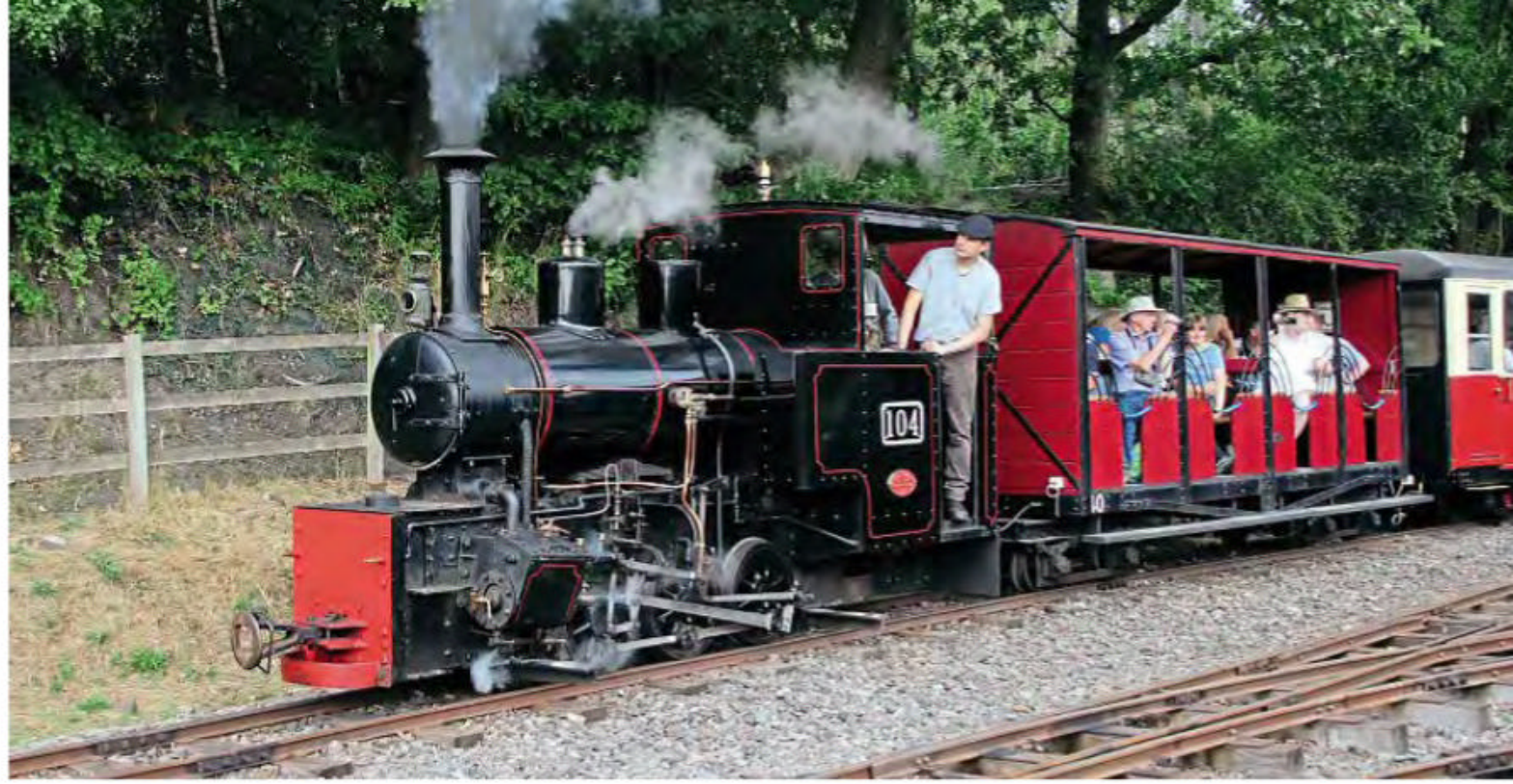
The 2ft gauge Apedale Valley Light Railway operates an interesting collection of rolling stock at weekends and Bank Holidays – including Hudswell Clarke 0-6-0WT No. 1238 of 1916. The locomotive is seen with a passenger train on July 14, 2018. GARETH EVANS
