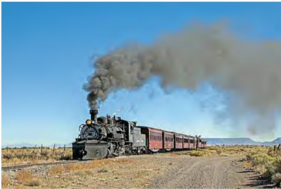
Built by Baldwin in 1925, No. 487 is an outside-framed K-36 class 2-8-2. It is seen with a Cumbres & Toltec Scenic Railroad train at Antonito on September 28.
