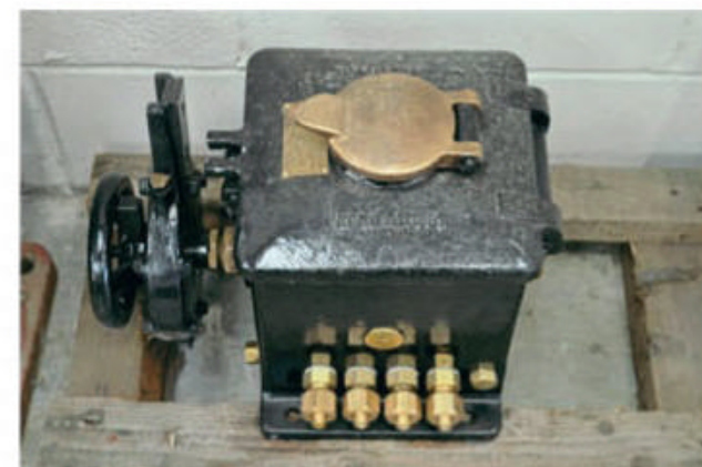
Some serviceable second-hand components have been sourced for use in the project – including three lubricators. Two of these are of the Wakefield mechanical variety and of differing types. This eight-feed example has been refurbished. MARK SMITHERS
