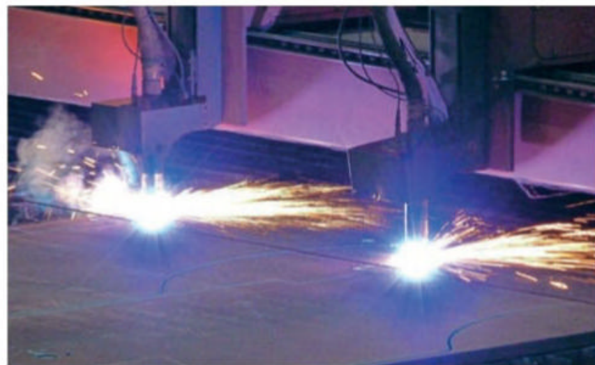
Above: History being made as the frames for the new County 4-4-0 are cut. CCT
