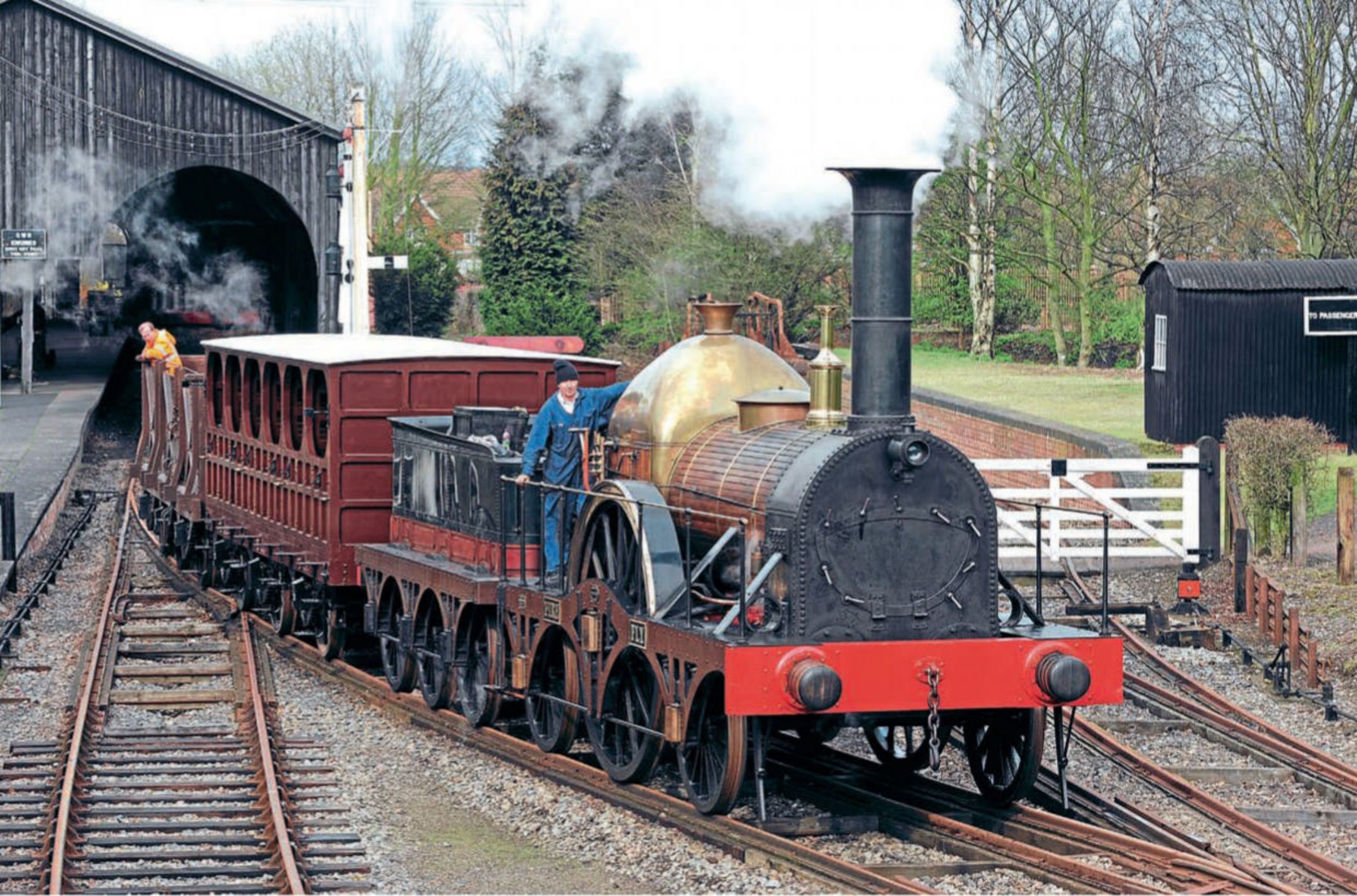
Fire Fly , the first of a class of 62 2-2-2s, was designed by Daniel Gooch for the GWR and built by Jones Turner & Evans in 1840. A replica was completed in 2005 and operates on the broad gauge line at the Great Western Society's Didcot Railway Centre. FRANK DUMBLETON/GWS
