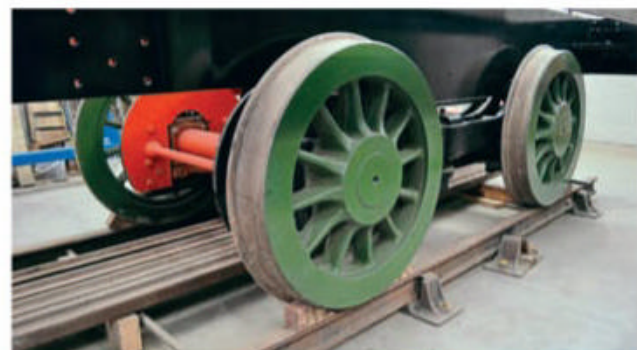
The external left-hand face of the bogie. Ahead of the bogie each side mainframe is 'kinked' inwards, reducing the overall mainframe assembly width to allow clearance for the bogie movement on curves. MARK SMITHERS
