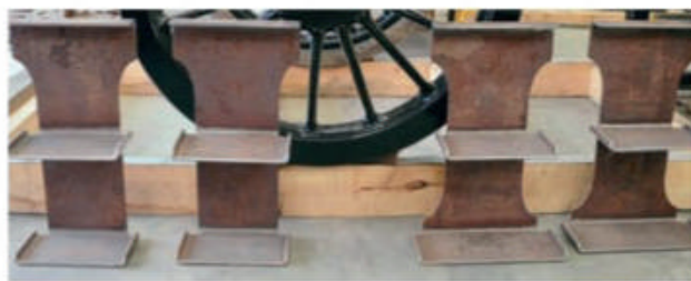
The leading pair of steps (left) and trailing pair (right) are seen in this photograph. The trailing pair give access to the cab and have wider bottom treads. MARK SMITHERS
