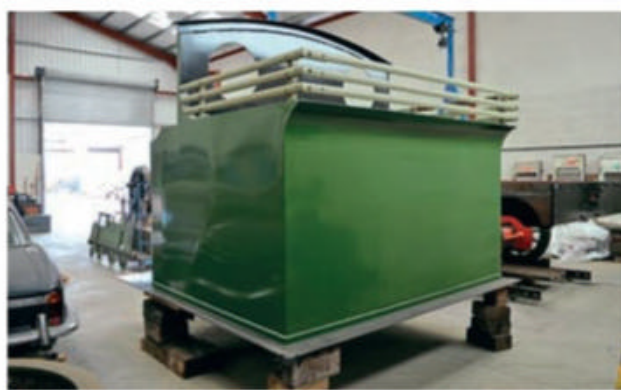
The rear spectacle plate and bunker are seen here photographed from behind. The coal rails have already been fitted. MARK SMITHERS
