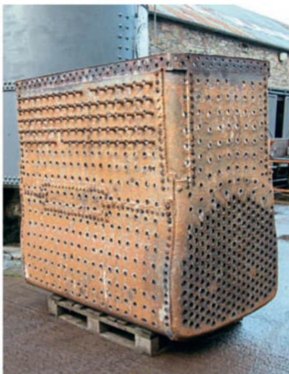
After several weeks' work carefully drilling out the copper stays, the firebox of the Swanage Railway's LSWR T3 4-4-0 No. 563 has been successfully removed intact. The engine, somewhat controversially gifted to the Swanage Railway by the National Railway Museum, is being assessed for repair at the Flour Mill workshop at Bream in the Forest of Dean. Steel sections of the boiler were inspected by Mike Brown of Royal Sun Alliance on November 30 and repair proposals will shortly be forthcoming. NATHAN AU/SWANAGE RAILWAY
