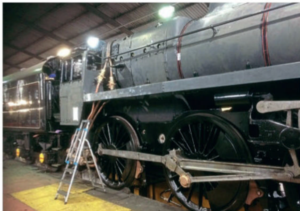
Right: Riddles BR Standard No. 75069, inside the workshops at Bridgnorth, has its boiler cladding and pipework fitted and is almost ready for testing. NEIL TAYLOR/SVR
