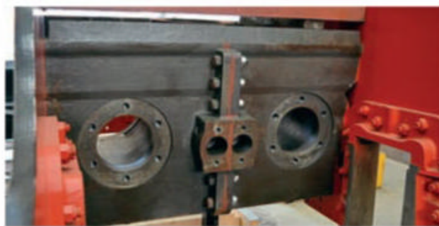
The cylinder block's basic two-piece construction is seen here. This will be advantageous should one half of the block ever require replacement, meaning an entire new component could be avoided in such an eventuality. The joining flange bisecting the block is very much in evidence, along with the securing bolts and the fact that the trailing cylinder covers have yet to be machined and fitted. MARK SMITHERS
