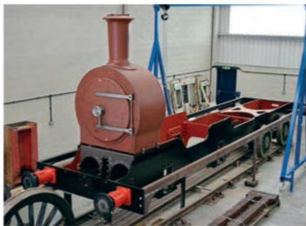
This overhead view shows the mainframe/bogie and smokebox assembly. The newly-fitted running board angle irons (supplied by Franklin Steel plc) can also be seen clearly. MARK SMITHERS
