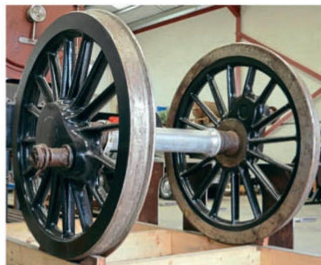
The leading wheelset has already been completed and is seen here on display close to the workshop entrance. The crankpins have also been fitted. MARK SMITHERS
