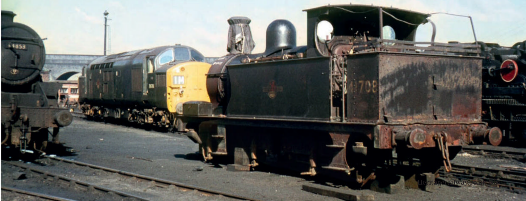
Below: A casualty was MR Johnson 1F 0-6-0T No. 41708, which had been purchased for preservation on the Keighley & Worth Valley Railway but ran hot during its journey from Sheffield. It was jacked up on sleepers for some time while under repair and is seen on March 16, 1967. HR
