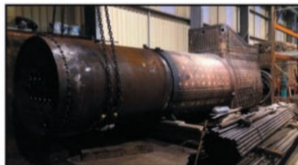
The newly assembled boiler at Tyseley in October 2018
