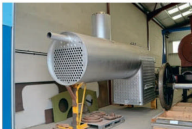
A front left three-quarter view of the boiler, which is of all-welded construction. The two leading firebox washout valves can be seen in this view, along with the 179 boiler tubes (as opposed to 205 on the original); steam and blower pipes; the leading ends of the longitudinal stays and the flanges for the safety valves. MARK SMITHERS
