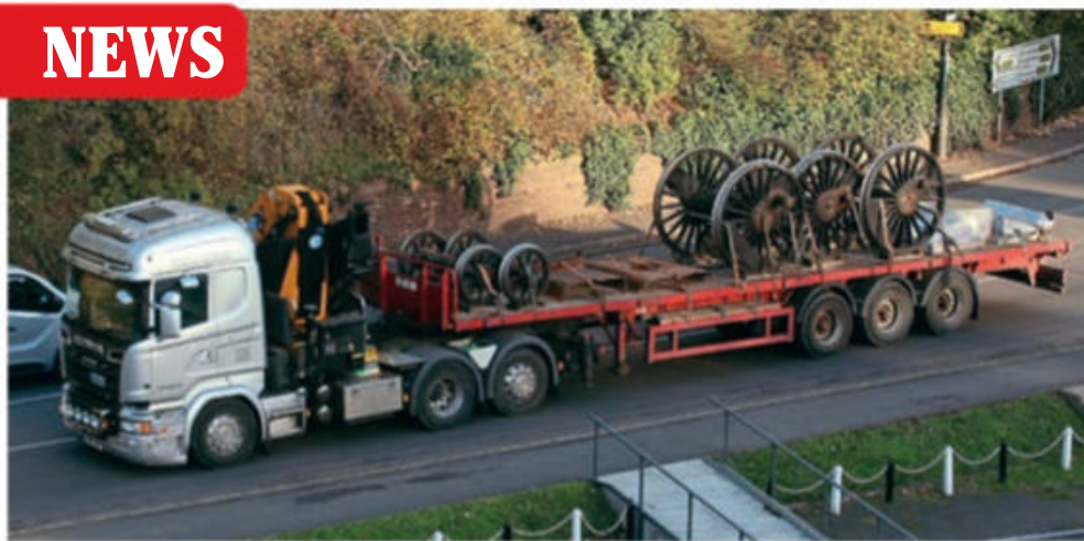
Above: No. 4930 Hagley Hall 's wheel sets are returned to Bridgnorth after being turned at South Devon Engineering. NEIL TAYLOR/SVR
