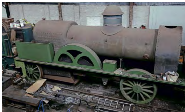
By no means forgotten is the scheme to build a LNWR 'Bloomer' 2-2-2, which began in the late 1980s when three tender underframes were discovered, and a grant obtained from Birmingham council. An all-welded steel boiler was completed in 1987 and the six steel wheels cast. Sadly, the early impetus was lost as Tyseley understandably developed its core business. However, the team hopes to have what could be a flagship locomotive for the city running in time for the opening of HS2 from London to Birmingham. ROBIN JONES
