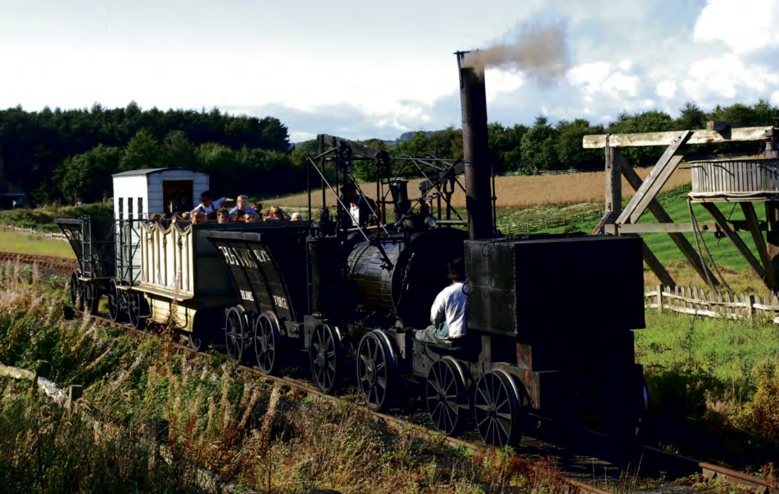
The replica of William Hedley's 1812-built Puffing Billy in action on the Pockerley Waggonway at the Beamish Museum. The driver and fireman are at opposite ends of the boiler. The two vertical cylinders drive one of the two pairs of wheels. BRIAN SHARPE
