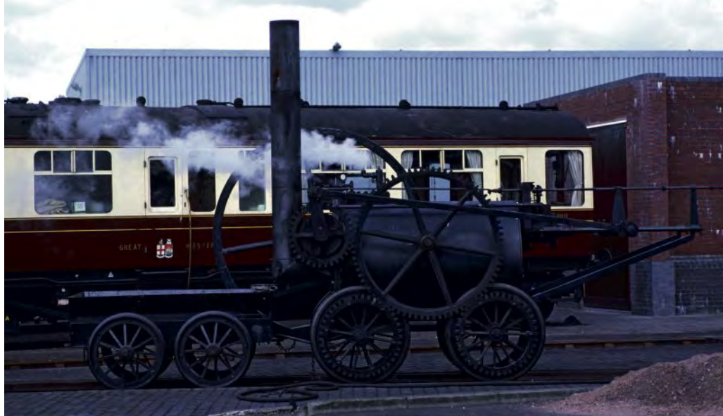
The replica of Richard Trevithick's 1804-built 0-4-0 for Pen-y-Darren ironworks, seen at Tyseley. Originally a stationary engine, it was temporarily converted to run on rails. The single cylinder is now at the other end of the boiler and the crankshaft is at the chimney end. The boiler has a single return flue and was mounted on a four-wheel frame. The cylinder has a very long stroke and a piston rod crosshead runs out along a slidebar, resembling a giant trombone. A large flywheel is mounted on one side to even out the motion. BRIAN SHARPE
