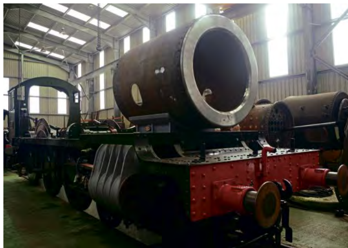
Visitors were able to view progress on the new-build GWR Grange 4-6-0, No. 6880 Betton Grange , typical of a class which ran past Tyseley in the early Sixties. The boiler is just about complete, but will stay at Tyseley until April, so jobs on the bottom half can be finished. It should then steam within weeks of returning to Llangollen. The 6880 Betton Grange (Society) estimates it needs £40,000 to finish the locomotive. ROBIN JONES
