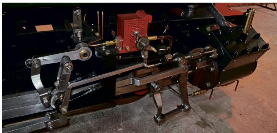
A leading right-hand view of the chassis. The reach rod from the reverser is located on this side of the locomotive, along with the mechanical lubricator.
