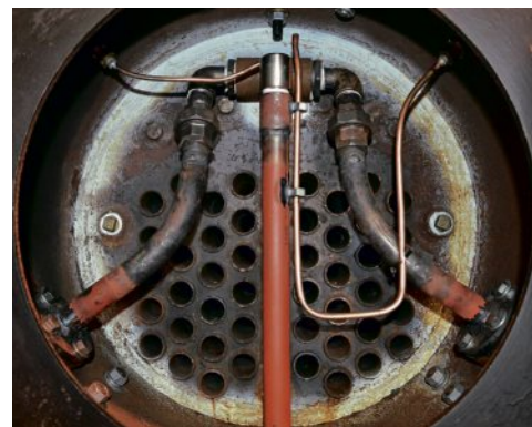
Inside the smokebox, the tube arrangement can be seen, along with the steam pipes and header (with lubricator feed pipe) and blastpipe. The basic U-shaped configuration of the blower pipe is also very much in evidence.
