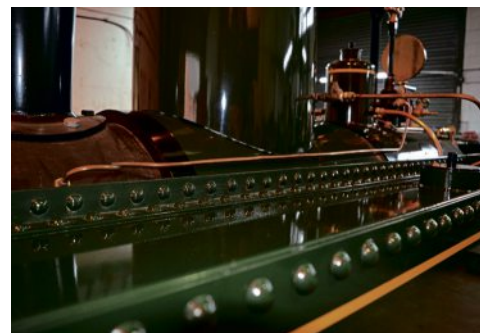
Visible here are the leading portion of the blower pipe, the upper surface of the left-hand side tank, part of the dome and the sandbox. Note the riveting and the tank filler.
