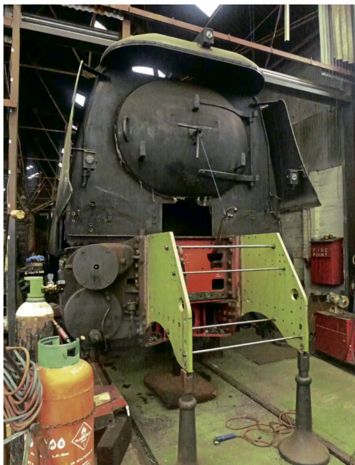
Repairs to the front of Swanage Railway-based Bulleid Battle of Britain Light Pacific No. 34070 Manston at Tyseley Locomotive Works are well underway. The buffer damage it sustained in a low-speed non-injury collision – during shunting operations – between Manston and BR Standard 4MT 2-6-4T No. 80104 in an area not open to the public between the signalbox and the engine shed at Swanage station just after 9am on Monday, July 24, 2017. ROBIN JONES
