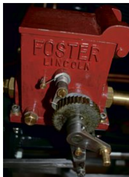
Edgar is fitted with a Foster mechanical lubricator.
