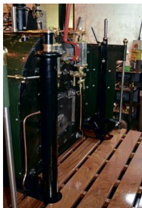
Left: A view of the backhead taken from the left-hand side. The handbrake column can be seen on the left, and reversing lever is to the right. As an aid to comfort for the driver, Edgar has wooden flooring on the cab footplate.
