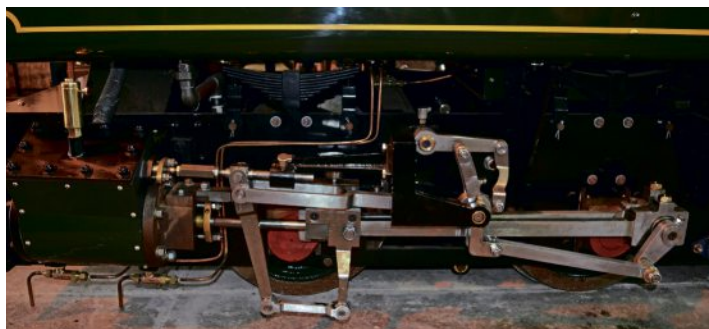
A leading right-hand view of the chassis. The reach rod from the reverser is located on this side of the locomotive, along with the mechanical lubricator.
