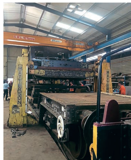
Above: No. 656 was lowered off the Matterson jacks and onto a Weltrol wagon inside Wansford works on August 8. SMALL LOCO GROUP
