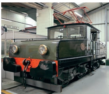
Built by Siemens in 1909, electric locomotive E4 now takes its power from batteries in a four-plank wagon.
