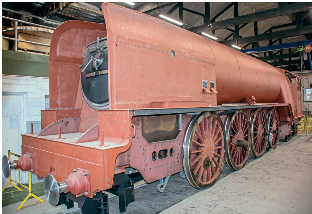
Wheely there: The world's fastest-growing standard gauge new-build steam locomotive project, P2 No. 2007 Prince of Wales , now has all eight driving wheels beneath it. MANDY GRANT
