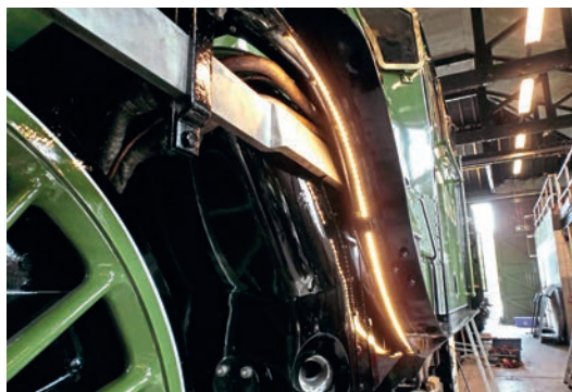
The outside frame LED lighting fitted to Tornado . ROB MORLAND
