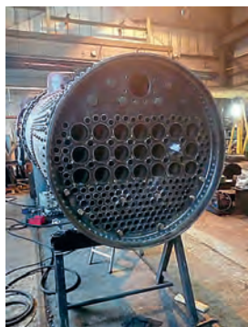
The boiler for No. 75069 is virtually complete inside Bridgnorth boiler shop, with all tubes, flue tubes and washout plugs fitted. SVR
