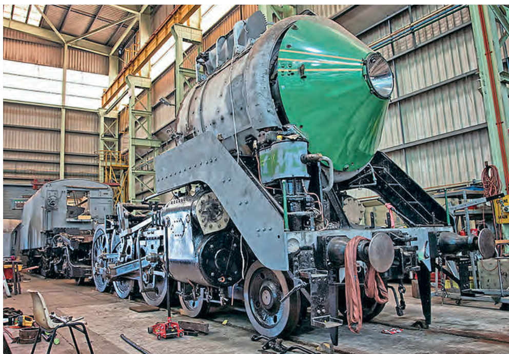
Right: Late delivery: The streamlined front of Class C38 No. 3801 looms large as its restoration continues in the state government-owned Chullora railway works near Sydney. The Pacific's overhaul was originally expected to be completed in 2011. TRANSPORT HERITAGE NEW SOUTH WALES
