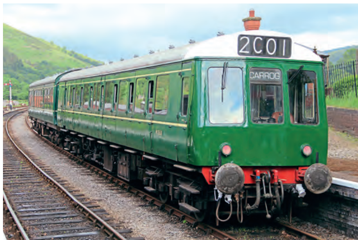
Class 127 Driving Motor Brake Second No. 51618 to the fore at Carrog during the gala. The car is one of eight surviving Class 127 vehicles. LR
