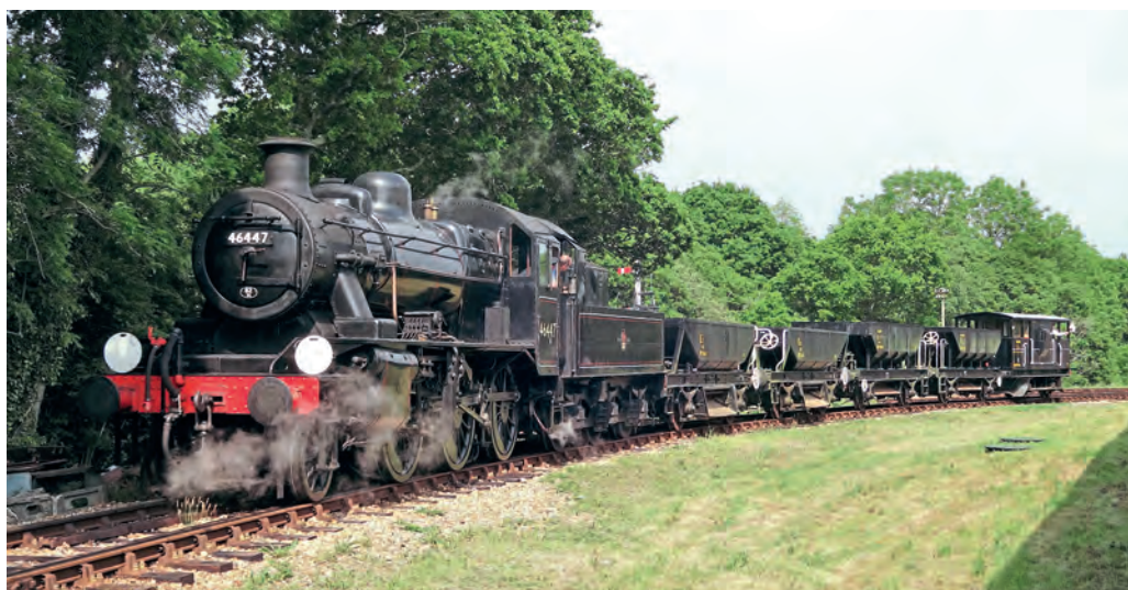
Ivatt 2MT 2-6-0 No. 46447 shunting a train of ballast hoppers plus a 20-ton ballast plough brakevan. The two Dogfish hoppers closest to the camera came from London Transport and the two furthest from the camera, came from Eurotunnel. STUART DUDDY
