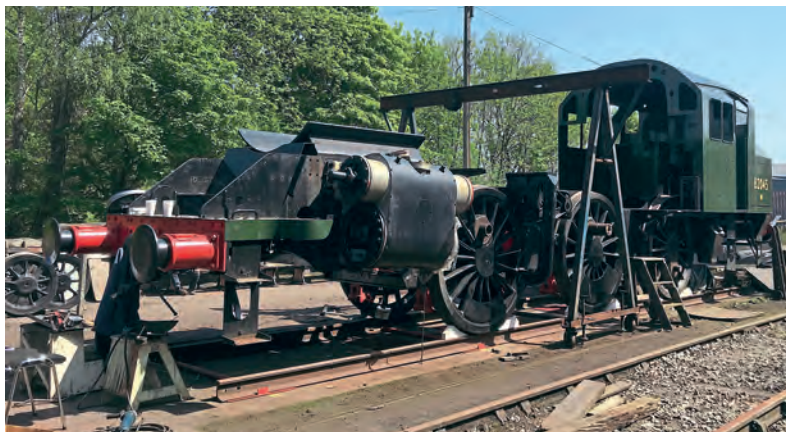
New-build BR Standard 3MT 2-6-2T No. 82045 was wheeled for the first time at Bridgnorth on April 17. PAUL APPLETON
