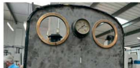
Katie's boiler backhead. The water gauge safety glasses are a modern refinement.
