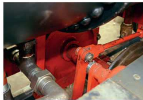
The left-hand leading pull-rod of the locomotive's brake linkage.
