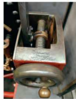
Left: The details of the combined screw and lever reverse mechanism, with the half-nut catch in the centre.
