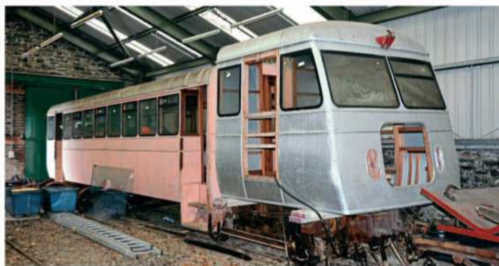
Railcar No. 20's cab paired with No. 19's coach body at Douglas, showing the extent of restoration on November 5, 2017. DAVID BOOTH, ISLE OF MAN STEAM RAILWAY SUPPORTERS' ASSOCIATION.
