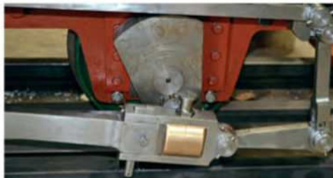
The 'big end', showing the cylindrical split enclosed bearing and the counterbalanced flycrank, both refinements introduced by Heywood on Muriel in 1894.
