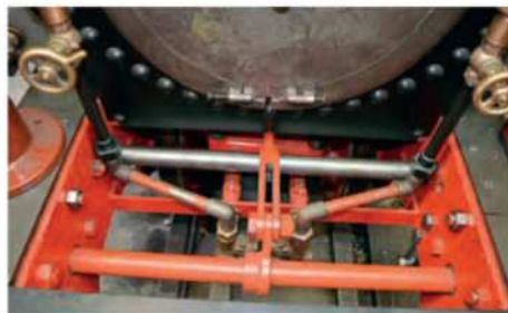
Katie's boiler backhead. The water gauge safety glasses are a modern refinement.
