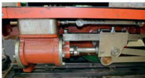
Katie's left-hand crosshead. Note the piston tail rod, single slide bar and adjustment provision in the valve rod for setting purposes.
