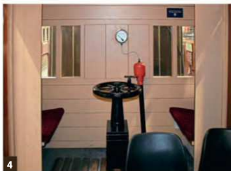
4 GNR No. 2856's fully rebuilt guard's compartment.
