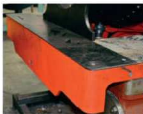
The leading headstock assembly. Unlike the original arrangement, functioning sandboxes have not been adopted on the reconstruction.
