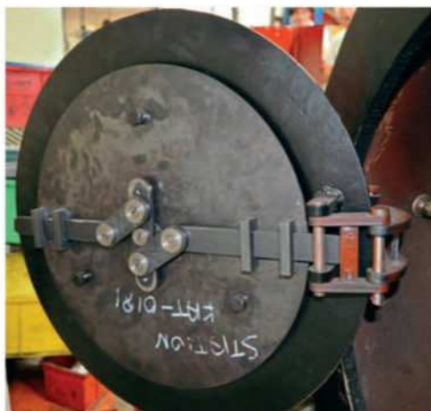
The internal locking arrangement for Katie's smokebox door consists of the rod-and-bellcrank mechanism. Unlike the internal hinge now fitted (which contains an intermediate link), it is likely that the original was a slip-hinge.
