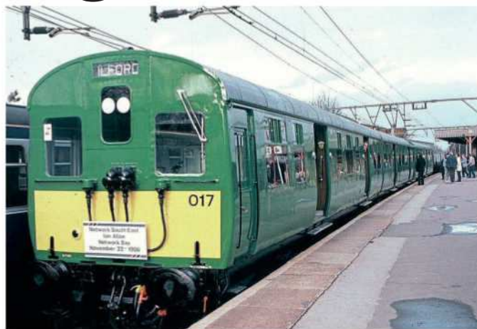
Class 306 EMU last survivor No. 306017 returned to service in original green livery to operate a Seven Kings-Shenfield shuttle service as part of a Network Day sponsored by Ian Allan to mark the launch day of Network SouthEast. This view also shows the carriage which was not modified when the trains were converted from the DC to AC power supply system.
