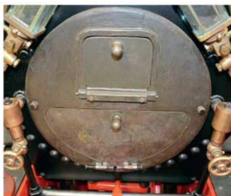
Katie's cast firebox backhead, with the firehole door (upper) and damper (lower).
