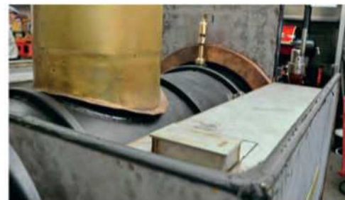
Katie's left-hand tank top is seen here. As with the original (and unlike the replica of Ursula ) it is double-skinned, i.e. it consists of the tank proper and an external valence. The rectangular filler (inspired by the surviving fitting on Muriel's tank) and boiler washout plug (not present on the original locomotive and not visible to the casual observer on the reconstruction) are also shown to advantage.
