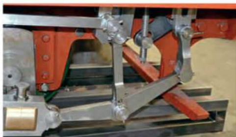
The bulk of the rear left-hand valve motion, including the swinging link; anchor and die block rods; die block and slide (John Wesley Hackworth-pattern) and the rear of the valve rod.
