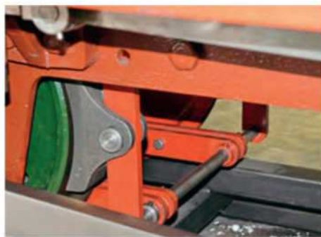
Katie's rear left-hand brake block, rear brake hangers and clasp rods.
