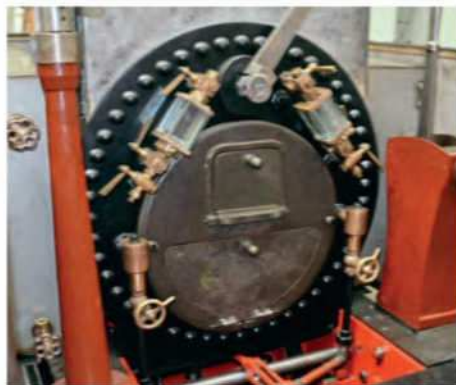
Katie's boiler backhead. The water gauge safety glasses are a modern refinement.
