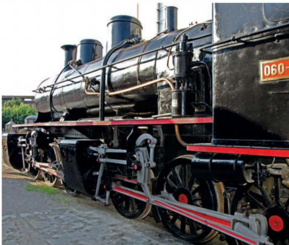
Mallets tend to be very attractive locomotives and to see one working is even better, 060-4013 built by Esslingen, Germany in 1906 is no exception.
