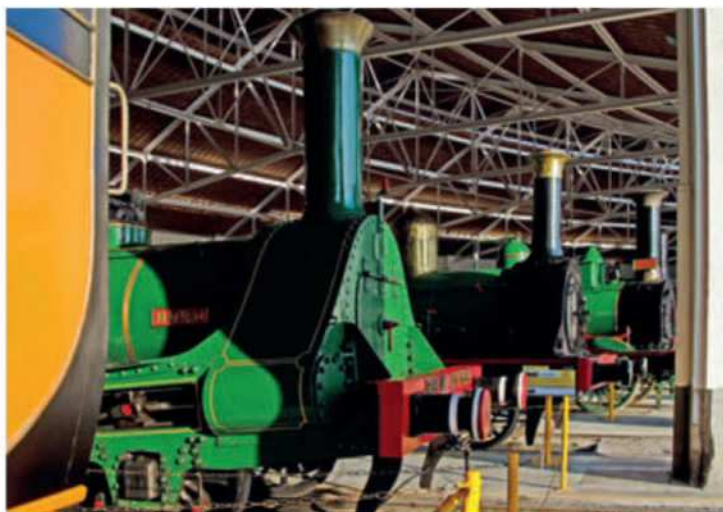
Three tall chimneys belonging to replica 2-2-2 Mataro built for the 100th anniversary of Spanish Railways, surely becoming historic in its own right; MZA 168 a Sharp Stewart 2-4-0T of 1853 and EB Wilson MZA 246 from 1857.
