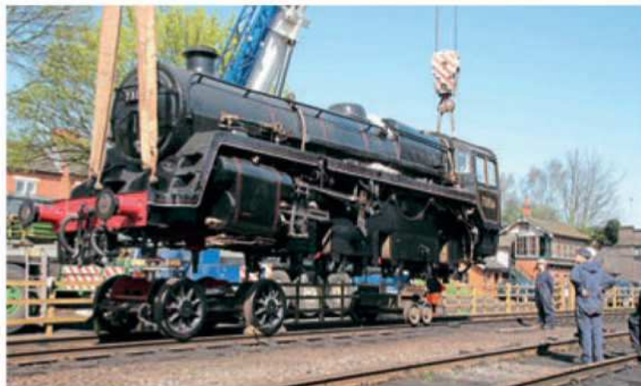
BR Standard 5MT 4-6-0 No. 73156 was successfully rewheeled by the team at the Great Central Railway's Loughborough shed on April 18 after receiving attention to the wheelsets. The recently-restored locomotive failed on the second day of the October 5-8 autumn steam gala and was withdrawn from traffic. Subject to testing, it was hoped that it would be available for the May 12-13 Goods Galore gala, at which it is planned to see six engines in steam. LES McWATT
