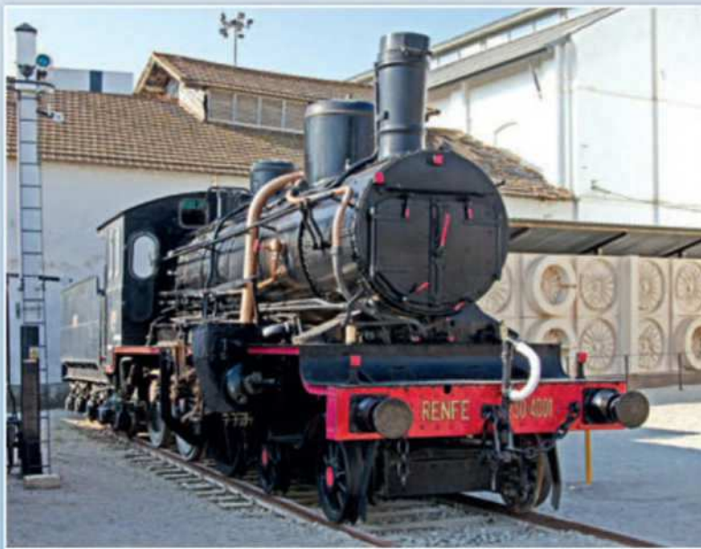
No. 230 4001; a 4-6-0 built by Hannoversche Maschinenbau AG, Germany in 1901. ALL PHOTOGRAPHS BY THE AUTHOR.
