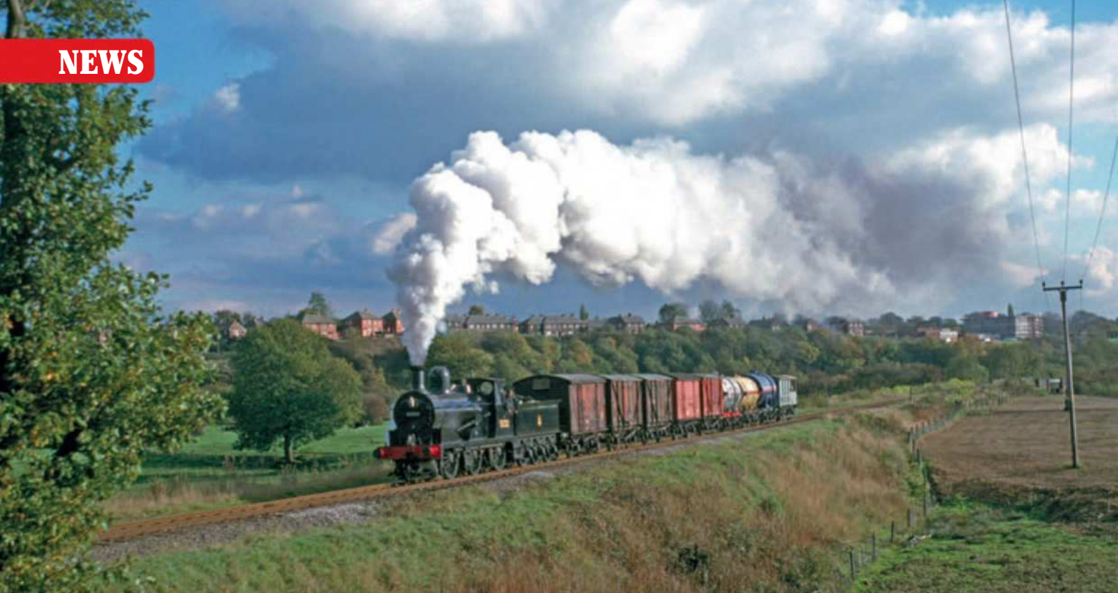
Venerable power: Former Lancashire & Yorkshire Railway Class 27 No. 1300 sports its final BR guise of No. 52322 as it heads a demonstration freight train at Burrs Country Park near Bury on the East Lancashire Railway in October 1995. The 0-6-0 was built at Horwich in 1896 and withdrawn in 1960 after 64 years' service with the LYR, LMS and BR. BRIAN SHARPE
