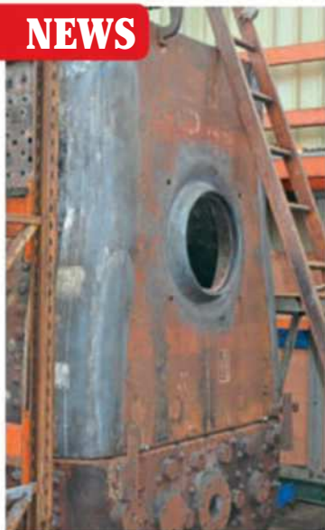
Trial fitting of the doorplate and backhead of the inverted boiler for No. 6880 at Tyseley Locomotive Works in early March. CHRIS MOORE
