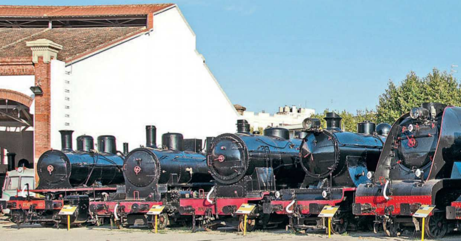
Where else is there a sight like this? The first three numbers denote number of axles. From the left are Mallet 060-4013, 230-2085, 240D2135, 240-2074, 241F2108, 151-3101, 240F2591 and 240F2705. The first three are German-built, then one from Belgium and the rest Spanish.
