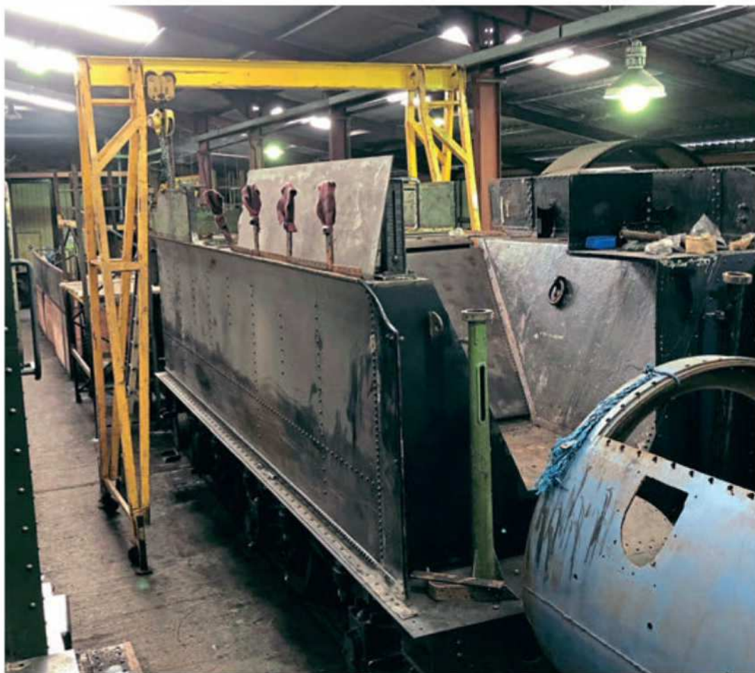
The tender earmarked for GWR 2-8-0 No. 3814 in the latter stages of overhaul inside the workshops at Llangollen. Agreement has been reached for it to run with No. 6880 Betton Grange while its owner's locomotive is still undergoing restoration. Little is known about this vehicle, other than it is a genuine GWR Collett 4000 gallon vehicle, with a six ton coal capacity – its number and its operating history remain a mystery. What is known is that it was bought from BR departmental use, possibly by the owners of West Country No. 34007, before being sold to its present owner, who also owns a Churchward 3500 gallon tender in unrestored condition. QUENTIN MCGUINNESS
