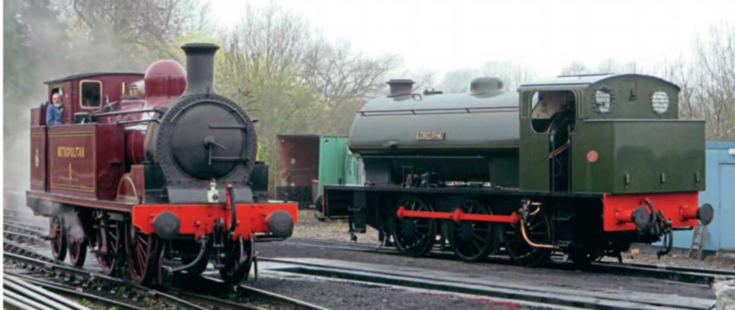
HUNSLET Austerity 0-6-0ST No. 3883 Lord Phil is to spend the season on loan at the Epping Ongar Railway and may stay on beyond. Built in 1944 for the War Department as Hunslet No. 2868, it was rebuilt as No. 3883 in 1963 as a trial for the Hunslet underfeed stoker and gas producer combustion system. It was also used for dynamometer car trials in 1963. It is pictured alongside Metropolitan Railway E class 0-4-4T No. 1 at North Weald on April 8. ANDREW SMITH
