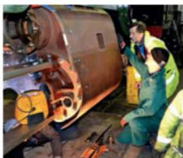
Work taking place on the right-hand cylinder cladding on No. 6880 Betton Grange at Llangollen in early March. LYNN MOORE
