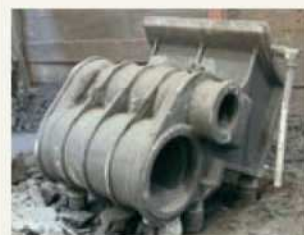
One of the new cylinder blocks for No. 3850. SHAKESPEARE CASTINGS
