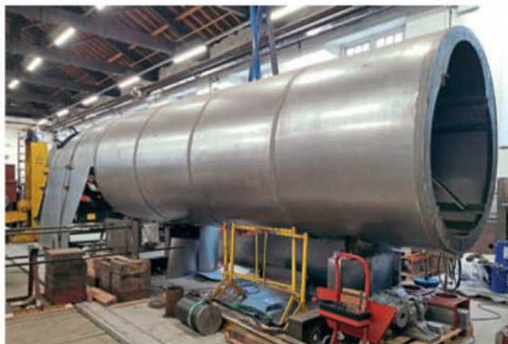
The boiler cladding for the new P2 Prince of Wales at Darlington Locomotive Works on March 4. MANDY GRANT/A1SLT
