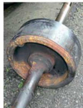
Right: The damaged front valve head as seen on April 14. A1SLT
