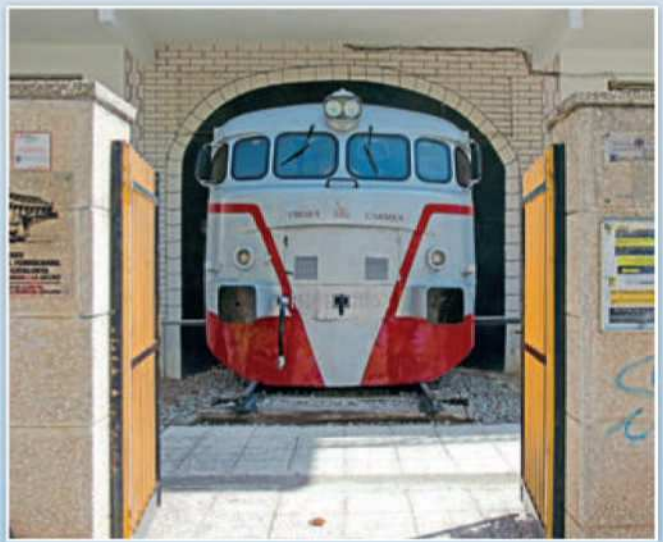
The entrance to the museum, with its Talgo train. Talgo trains are slightly unconventional because the wheels are not joined by an axle but mounted in pairs with the bogies shared between coaches, they can be fitted to enable a change of gauge from Spanish 5ft 6in to 4ft 8½in which enabled the first through train to run from Madrid to Paris in 1969.
