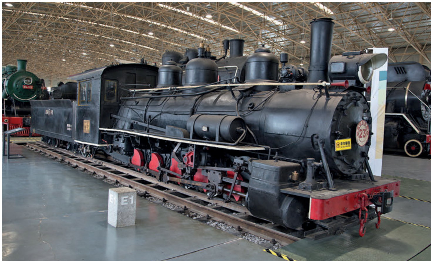
SN class 600mm gauge 0-10-0 built by Baldwin.
