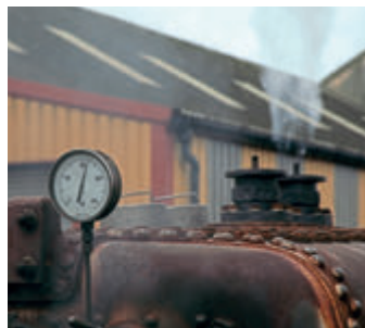
Bahamas' boiler passes its steam test at Tyseley on December 21. BLS
