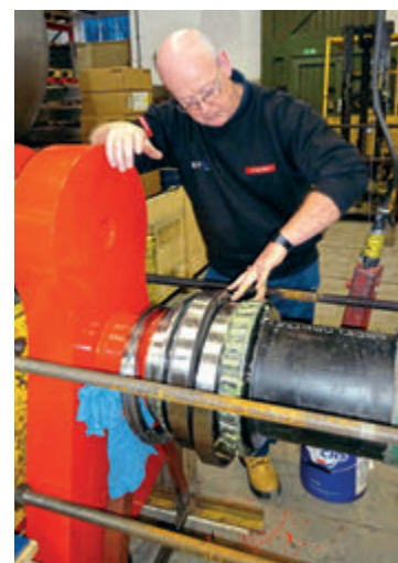
Bill Drumm applies grease to one of the bearings of No. 2007 on December 13. A1SLT
