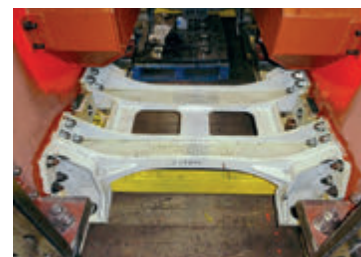
The P2's spring brackets and frame stay combined, as seen on December 21. A1SLT
