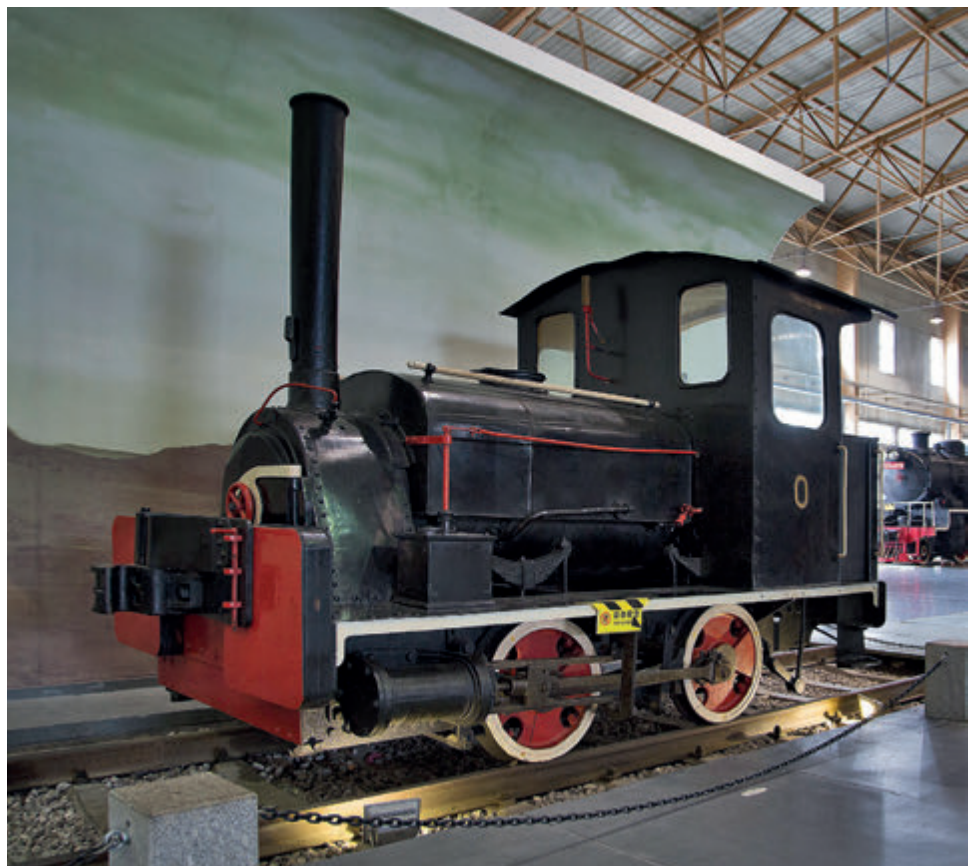
0-4-0ST No. 0, the first British-built locomotive to be imported by China in 1881, possibly built by Black Hawthorn & Co.
