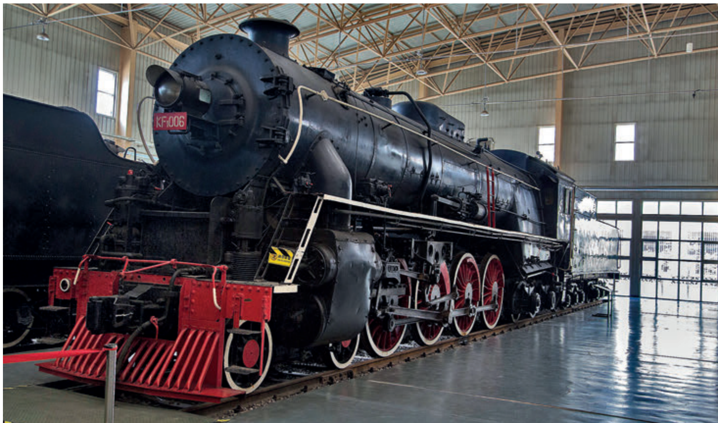
KF1 006, Vulcan Foundry built 4-8-4, of which a further preserved example is displayed in the NRM at York.
