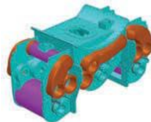
A drawing of the P2 cylinder block showing the Lentz-Franklin B valves. A1SLT
