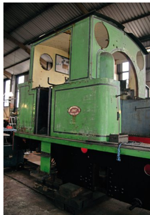
The right-hand cabside of Warwickshire . It will be seen that there are no radiuses on the corners of the cut-outs: apart from the bunker sides and upper spectacle plate areas the cab is made up totally of rectangular plates. This type of Manning Wardle cab, which may be termed an 'austerity cab', was introduced during the year preceding the outbreak of the First World War and persisted on a small number of locomotives constructed after the Armistice, including the 1922 rebuild of still extant No. 1207 of 1890 The Welshman . The size of the inverted 'U'-shaped firebox wrapper is well demonstrated, as are the positions of the spectacles, necessitated by the need for the best-possible view for the crew over the saddle tank.
