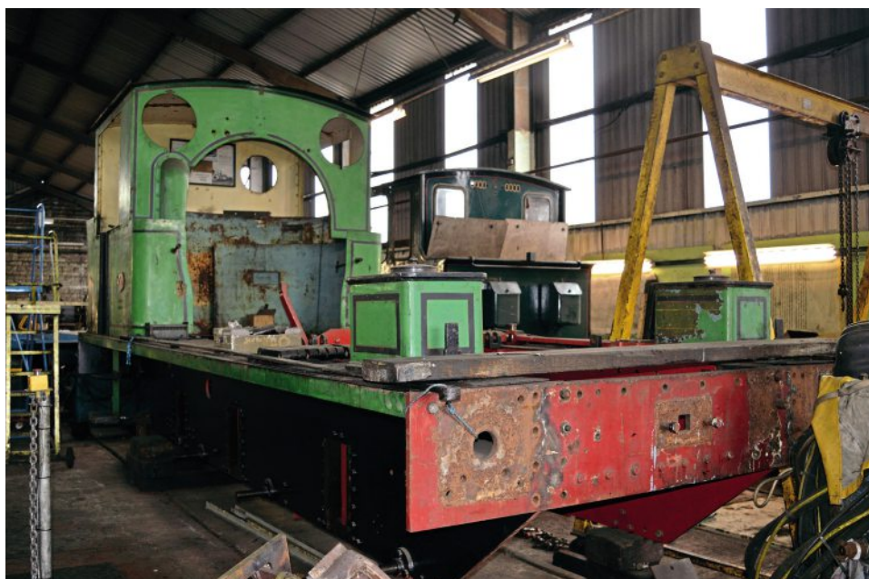
A front right hand three-quarter view of the mainframe/bufferbeam assembly and cab of Warwickshire undergoing restoration in the Bridgnorth workshops of the Severn Valley Railway. The components are restorable, as are the buffers, which had been removed.
