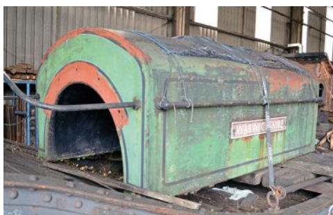
The saddle tank is restorable and currently awaits attention in the workshops at Bridgnorth. This front view shows the handrail, which passes around the chimney, and emphasises the cross-sectional profile, a standard Q class item, which was redesigned to be wider and lower during the early 1890s.
