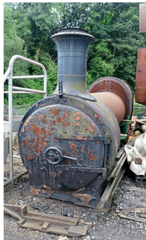
Warwickshire 's original boiler and smokebox assembly has been declared to be a total write-off and it currently sits in the yard at Bridgnorth. In addition to the domeless barrel and raised firebox wrapper, other trademark late Manning Wardle features are also visible, including the handwheel and reinforced seating strip for the smokebox door.
