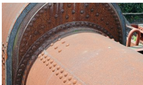
The lower left-hand area of this photograph illustrates well the longitudinal lap joint, that has proved to be the 'villain of the piece', ensuring that the original boiler, even if overhauled, would be effectively unsalvageable.
