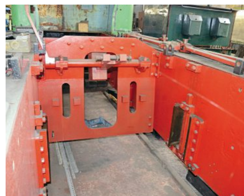
The area between the mainframes looking backwards from the rear of the cylinders to the motion stretcher. The weighshaft is fitted with a single 'Y'-ended bellcrank which raises or lowers the drop-links to produce the requisite forward/reverse and cut-off settings. Note the degree of protrusion of the stretcher above upper frame level, an indication of the raised boiler pitch necessitated by the position of the firebox.
