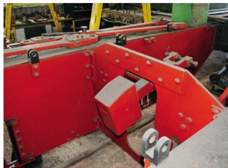
The balance weight for the weighshaft and the trailing face of the motion stretcher, with the hanger bearings for the leading springs. Unlike many six-coupled Manning Wardle products, Warwickshire was not equipped with compensating lever suspension between the leading and intermediate axles.
