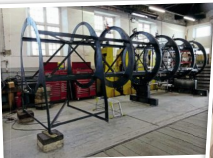
Above: The cladding assembly jig for Prince of Wales on July 14. A1SLT
