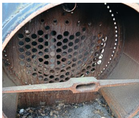
The life-expired smokebox and front tubeplate showing the tube arrangement. The uppermost two tubes appear to be of reduced diameter when compared with the others.
