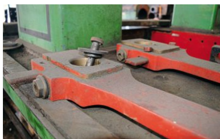
The leading and trailing split cotter pin bearings as used on the coupling rods of Warwickshire .
