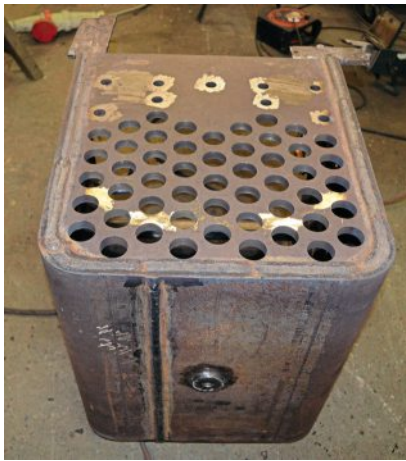
The 51-tube arrangement of the inner firebox of the Decauville locomotive, also showing the welded joints for the firebox crown and the inner wrapper/tubeplate connection.
