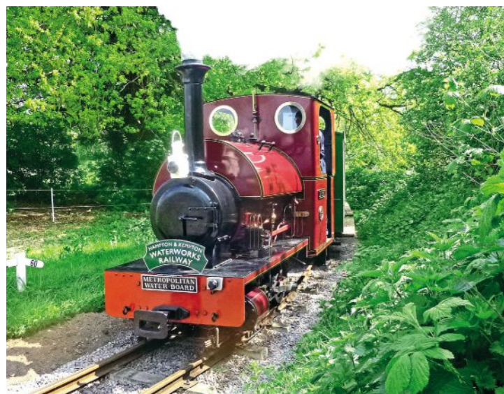
Steam near the Thames: Hampton & Kempton Waterworks Railway resident 0-4-0ST Darent , built by Andrew Barclay in 1903, heads a train on the line on April 23. The railway is currently in negotiations with Thames Water for a lease on part of the former 2ft gauge line that delivered coal from a wharf on the Thames to two waterworks. JIM HEWETT
