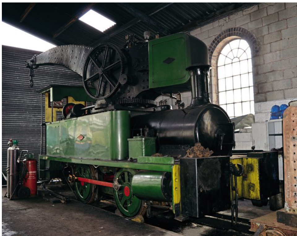
The ex-Shelton Iron & Steel Works Dubs 0-4-0 crane-tank (No. 4101 of 1901) in the shed at Caverswall Road undergoing attention to its right-hand crosshead and slide bar. The engine, which spent its revenue-earning career in Stoke-on-Trent, was expected to be back in service in readiness for the Foxfield Railway's 50th anniversary celebrations.
