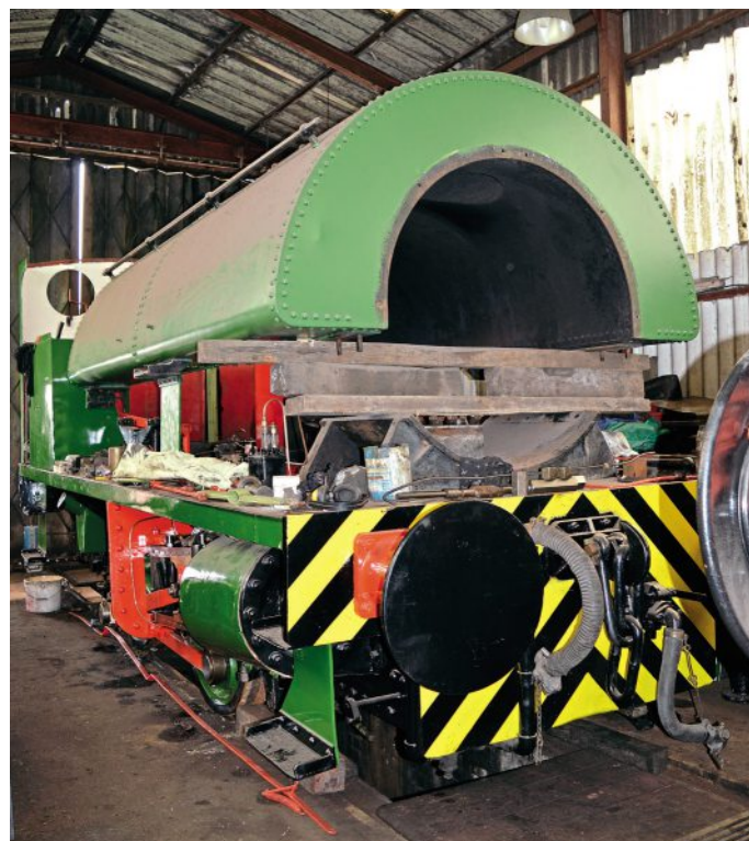
Above: The Bristol manufacturer Peckett produced some very workmanlike inside cylinder saddle tank locomotives, mostly six-coupled but there was also a small number of the four-coupled variety. The only known surviving inside cylinder Peckett locomotive is six-coupled 'X2' class Ackton Hall No. 3 (No. 1567 of 1920). The engine has been dismantled for restoration to working order.
