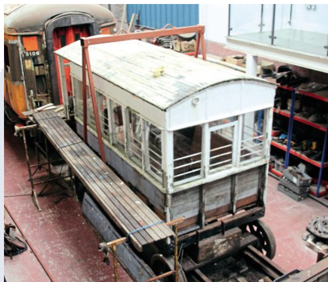
The tram trailer that was shown mercy by the nuns. Bessbrook & Newry Tramway No. 6 under restoration at Whitehead. The trailer is sitting on a 5ft 3in gauge boiler truck formerly used at the Great Northern Railway of Ireland's Dundalk works. HUGH DOUGHERTY
