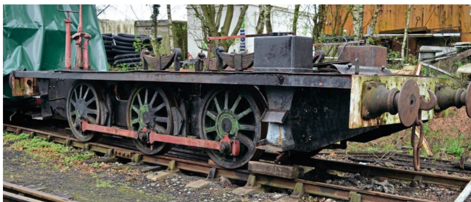
Above: The Bristol manufacturer Peckett produced some very workmanlike inside cylinder saddle tank locomotives, mostly six-coupled but there was also a small number of the four-coupled variety. The only known surviving inside cylinder Peckett locomotive is six-coupled 'X2' class Ackton Hall No. 3 (No. 1567 of 1920). The engine has been dismantled for restoration to working order.
