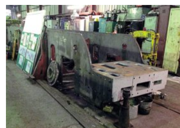
The B17’s dragbox undergoing a trial fit to the mainframes at Llangollen during the steam gala in March. B17SLT
