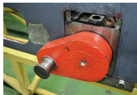
A close-up of the right-hand trailing crankpin and web. The latter component shows evidence of the arduous working conditions that were experienced by many industrial steam locomotives during their working lives.
