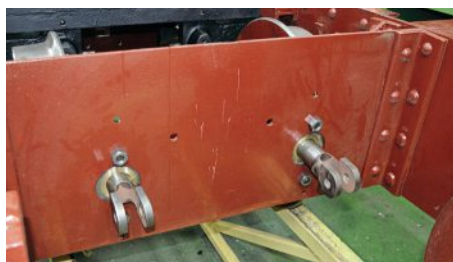
The valve rod stretcher. Unlike many Kerr Stuart, Manning Wardle and some early Hunslet narrow gauge locomotives, Liassic was fitted with two injectors and no pump as built, hence this stretcher has no provision for the fitting of a feed pump.
