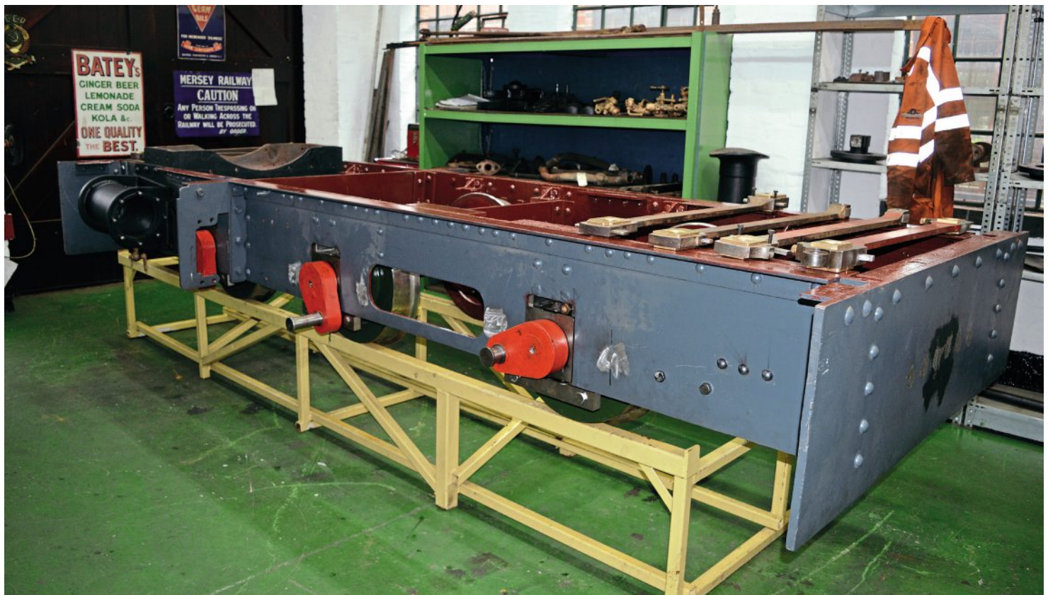
This rear three-quarter view of Liassic's chassis emphasises the nature of the locomotive's 'Quasi-Fell' wheelbase structure in which the firebox falls cleanly between the driving and trailing axles, necessitating a relatively long wheelbase.
