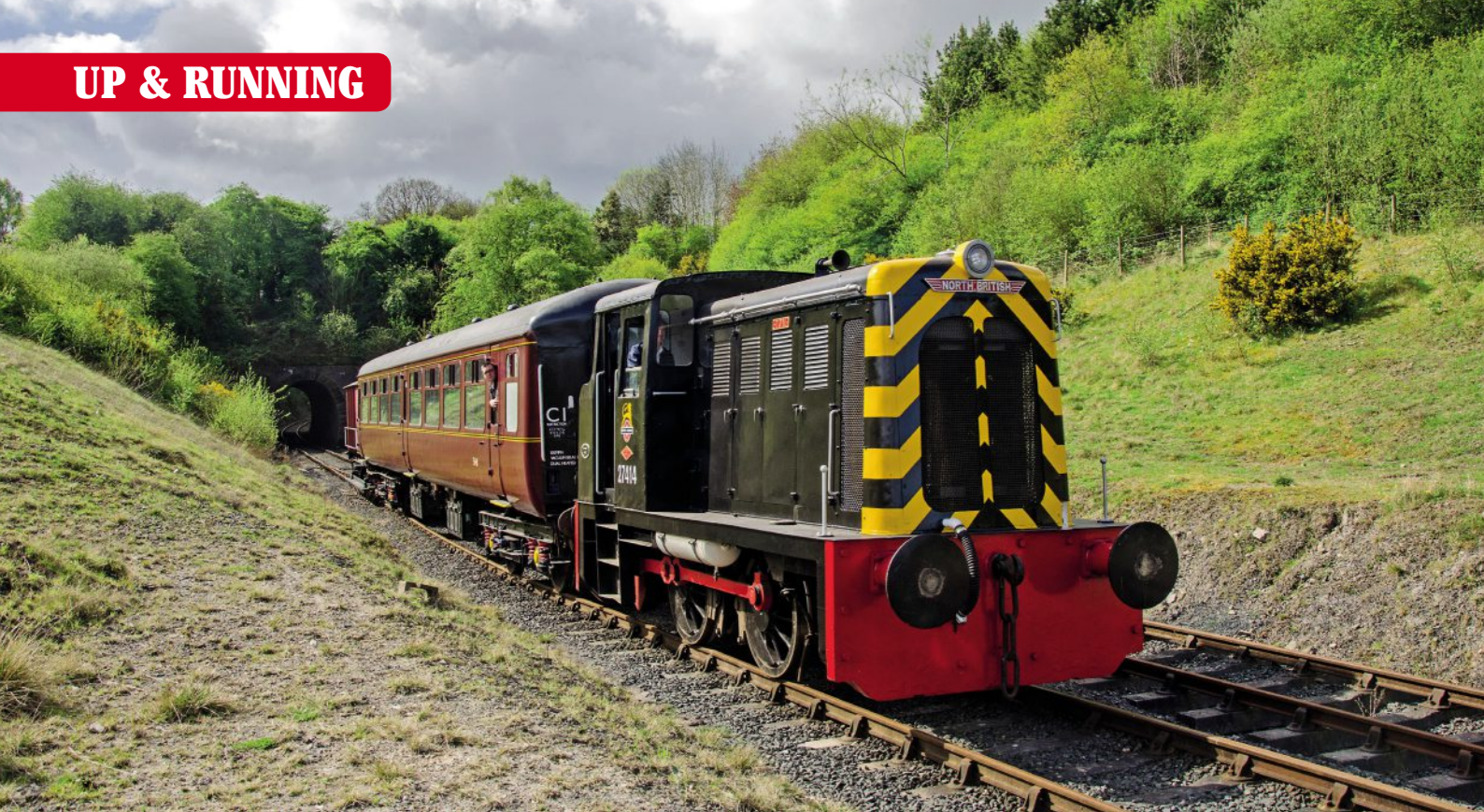
North British 0-4-ODM No. 27414 arrives at Lawley Village on the Telford Steam Railway on April 15 with its first ever passenger train in preservation, having been fitted with an eight-cylinder Rolls Royce power unit that was originally a standby generator at a hospital in Cork, Ireland. ALISTAIR GRIEVE
