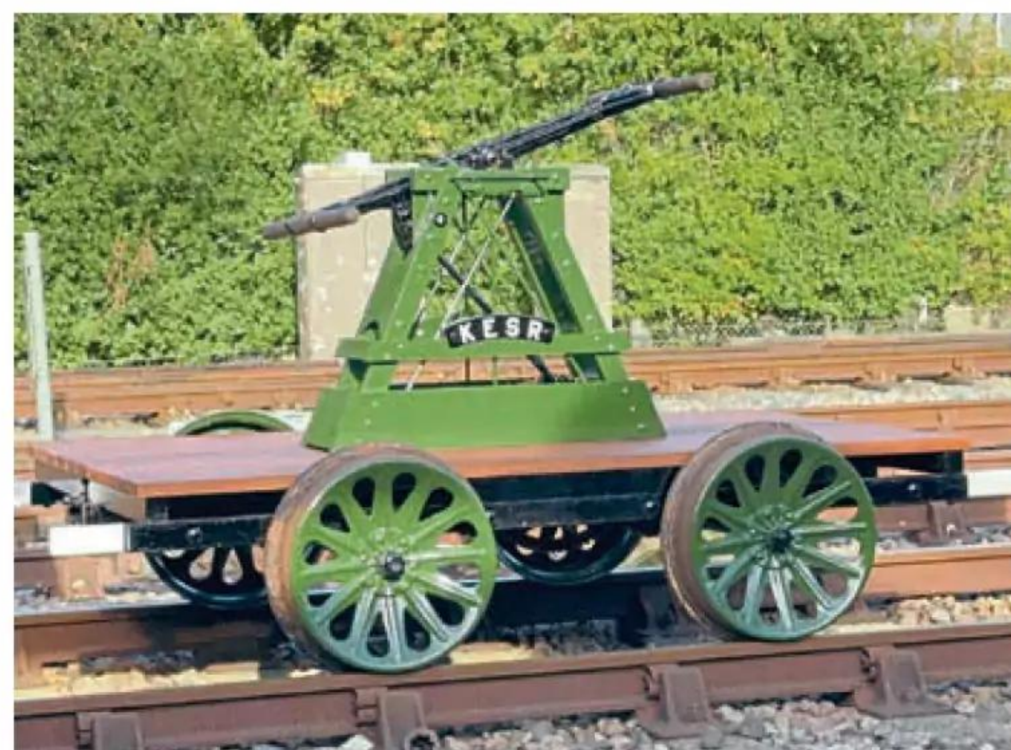
The newly refurbished KESR pump trolley, which is known to have been used on the line as far back as 1912. KESR
