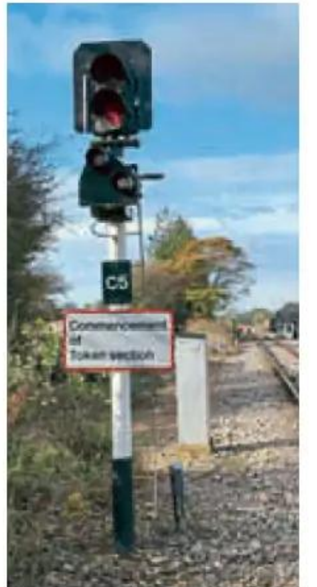
Above: A colour light signal in operation, pending the line's eventual transfer to semaphores. ESR
