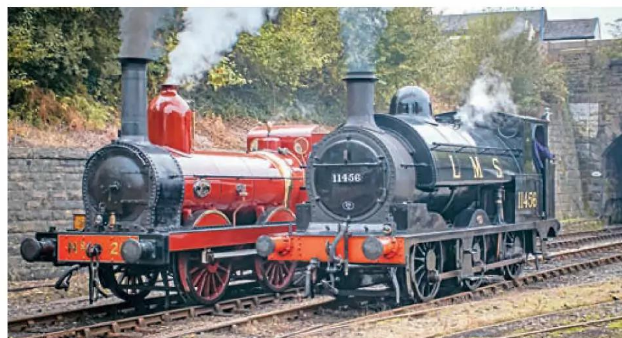
Nos. 20 and 11456 pause outside Bury Bolton Street. Both underwent rebuilds in their working lives, with the former starting as a tender locomotive, becoming a saddle tank, and then reverting to its original configuration in preservation, while the latter started as a tender locomotive and was later made into a saddle tank, the condition it which it has remained since. MATT DITCH
