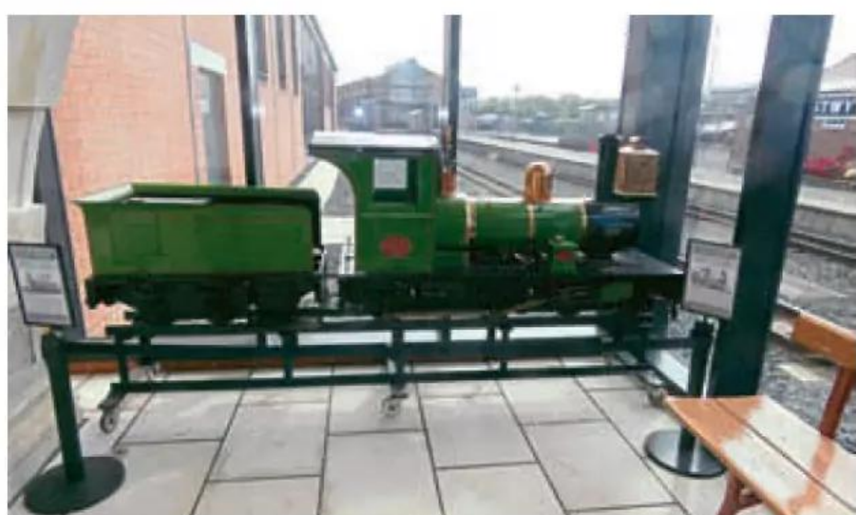
Above: Greeting visitors to the Engine Shed museum is this 7 1/4in gauge model of F2 4-4-0 No. NG104 Zulu, built by Brush Falcon on Loughborough in 1895 for the 2ft gauge Beira Railway in Mozambique – a type which was a particular favourite of Peter Rampton. The model was bought from the Bredgar & Wormshill Railway in 20020. ROBIN JONES
