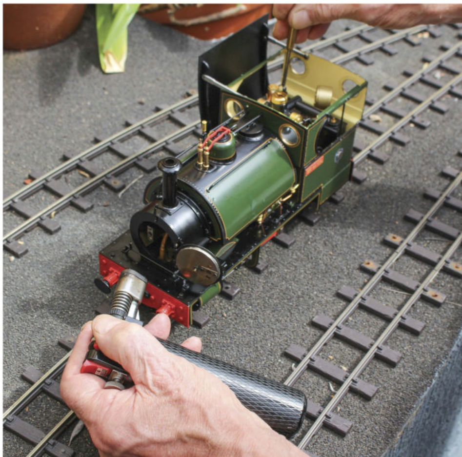
Lighting up is the traditional Accucraft way, smokebox door open, and introduce some fire. We tried gas torch and electronic lighters and both worked straight away.
