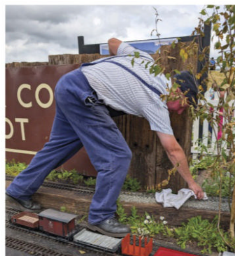
The gradient needed regular cleaning as oily track isn't conducive to adhesion.
