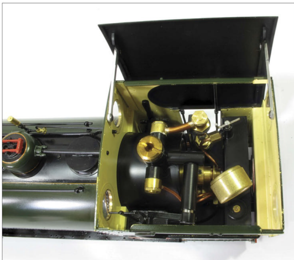
Looking inside the cab you can see the reversing lever in the top left, the moving around clockwise, we have a water gauge, gas control on top of the tank, pressure gauge, regulator and finally lubricator.
