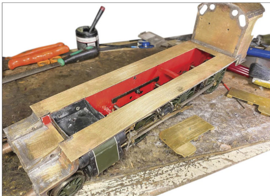
Footplate and cab assembled and bolted into place.
