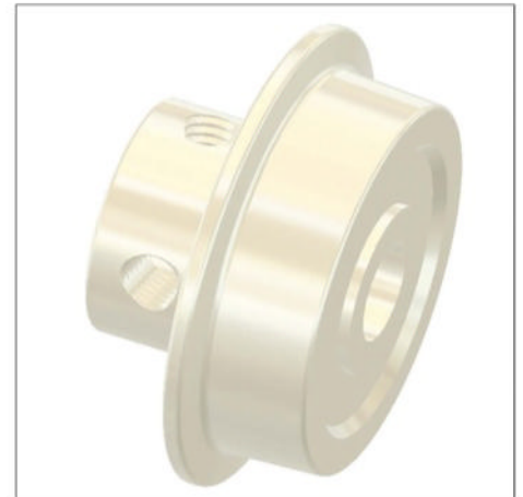
The CAD design for the wheels. Note the grub screw holes at the rear, I don't want any loose wheels!
