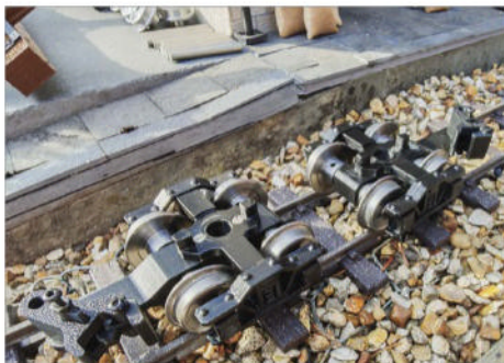
Assembled bogies, fitted with the wheels turned from metal blanks.
