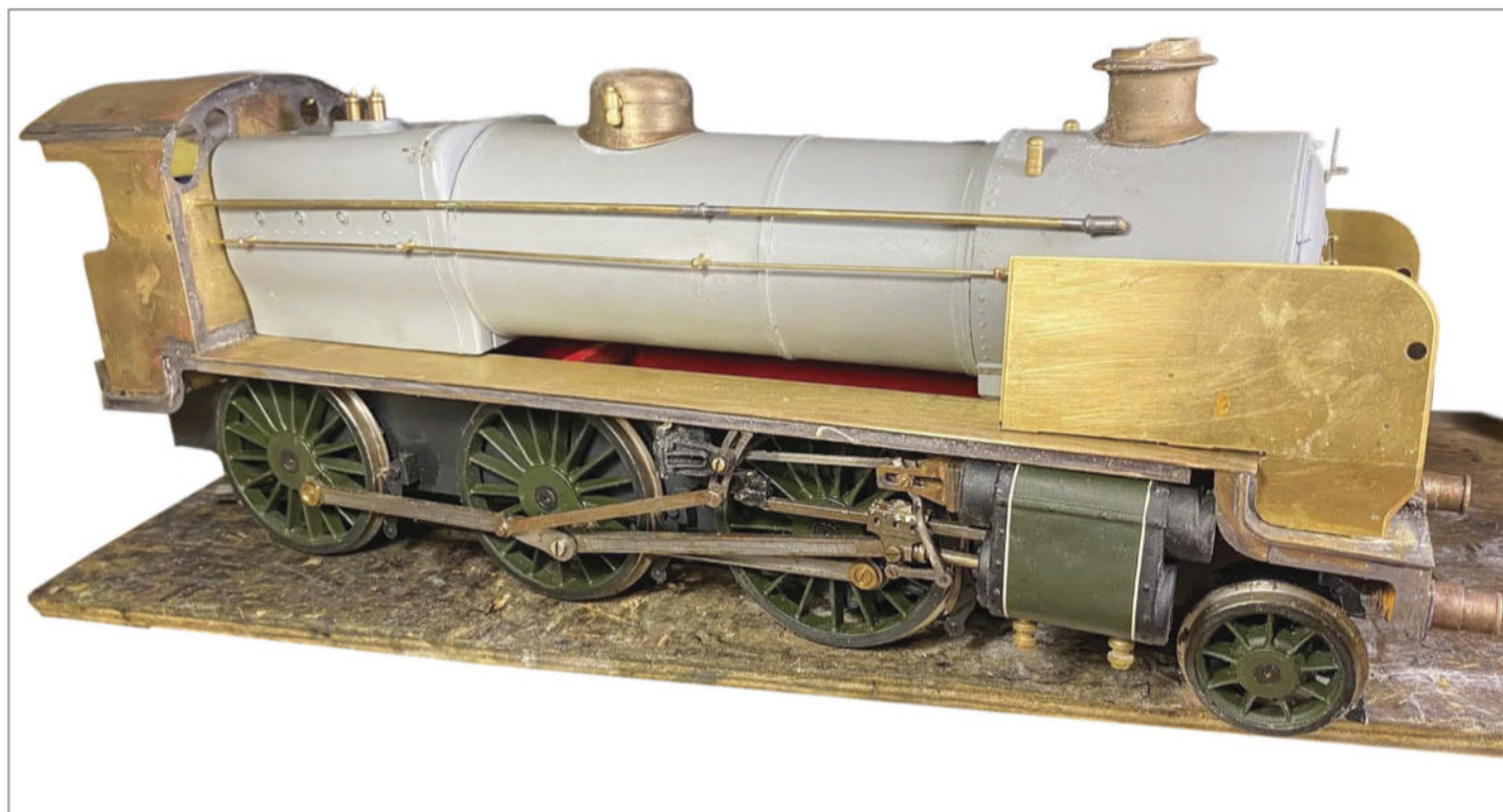
Boiler fittings, smoke deflectors and pipework being fitted.
