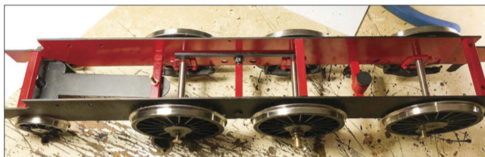
Looking down on the chassis, you can see the equalising beam between the non-powered driving wheels. Another aid to track holding.
