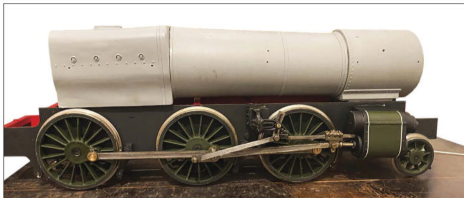
Test fitting the three large resin castings for firebox, boiler and smokebox.
