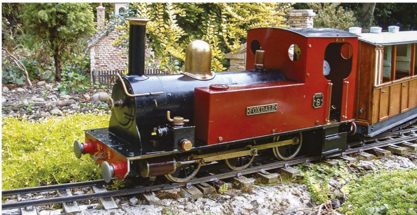
'Foxdale' after the Mamod repaint with a new dome and added handrails and cab steps.
