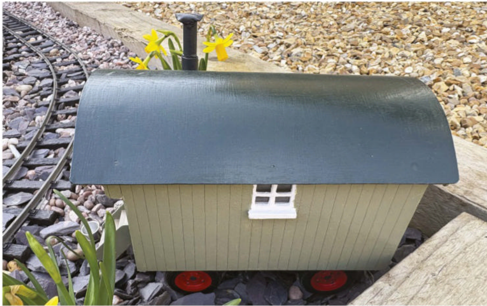
The side view of our Shepherd's Hut shows the curved roof, stove pipe and modern steel wheels, much like those fitted to many gypsy caravans nowadays.
