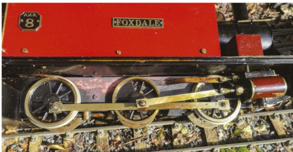
Close-up of the eccentric valve gear, fabricated rods and replacement wheels.
