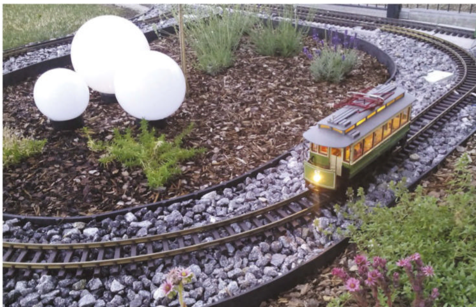
Return loops are much easier to wire up with digital control than normal DC.
