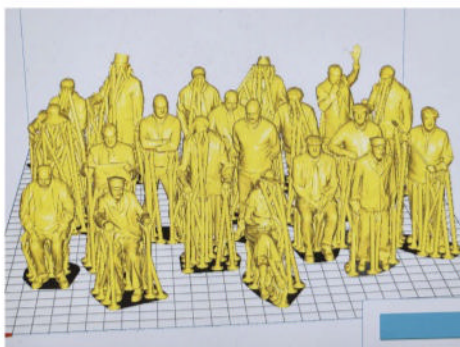
The digital display showing some of our figures ready to be printed with the support columns in place for the overhangs. This is what the printer will produce.
