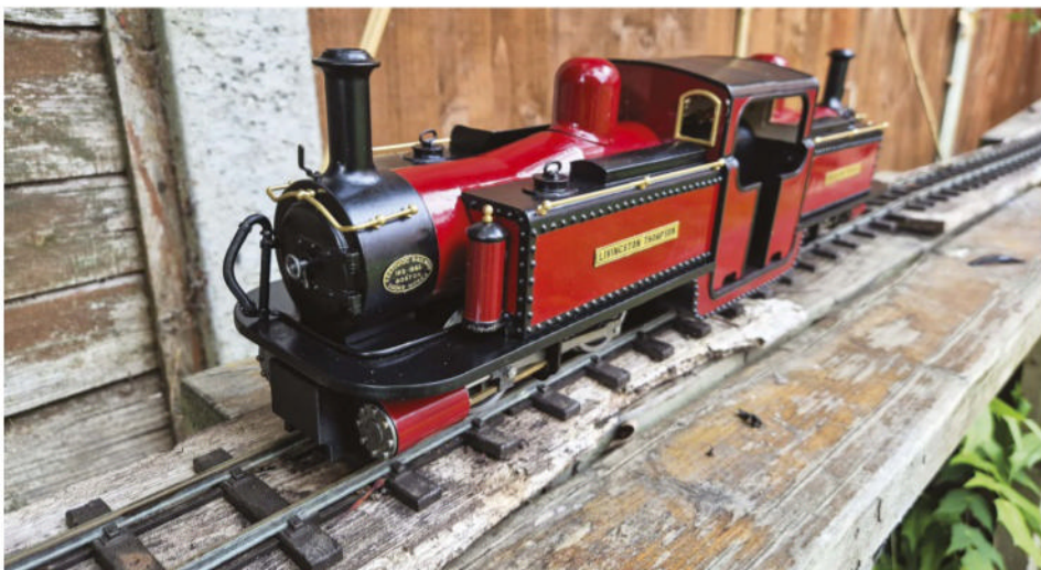
Sandpots, nameplates and worksplates added, the loco is definitely coming together
