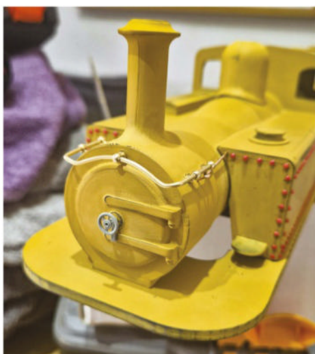
Smokebox handrails, blower pipe and rivet detail being fitted.
