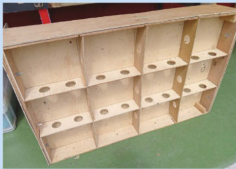
One of our baseboards. The plywood construction has stood up well to the rigours of exhibition use.
