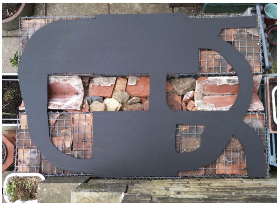
After marking out the 'final' (hah) trackplan, we took a Jigsaw to the Filcrist board. The shape could be, and indeed would be, modified further, not least the decision being taken to flip the trackplan over so the smaller of the two bridges would be on the other side.
