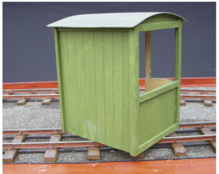
The back view of the cab, showing scribed planks. I think that the less-than-perfect paint job adds character.
