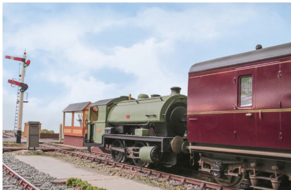
As well as the signal box, there is a covered ground frame, which is controlling this empty stock movement.
