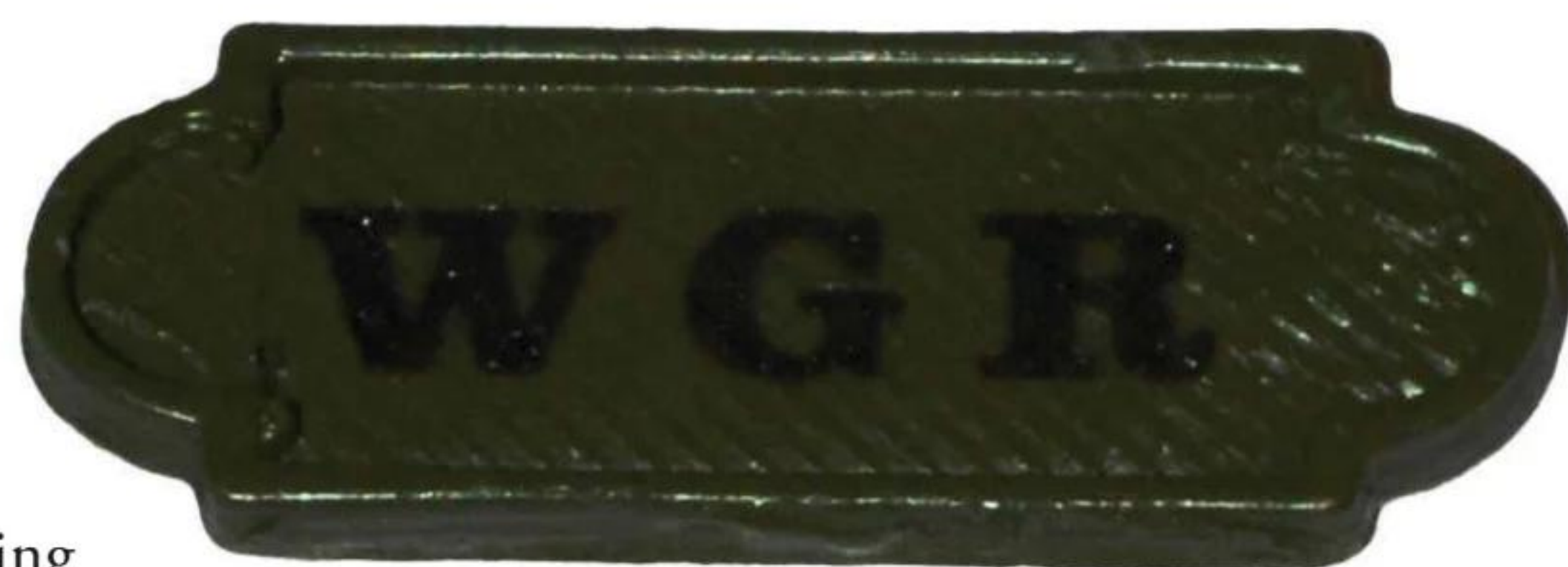
Sharp engraving, but FDM 3D printing struggles with small shapes.
