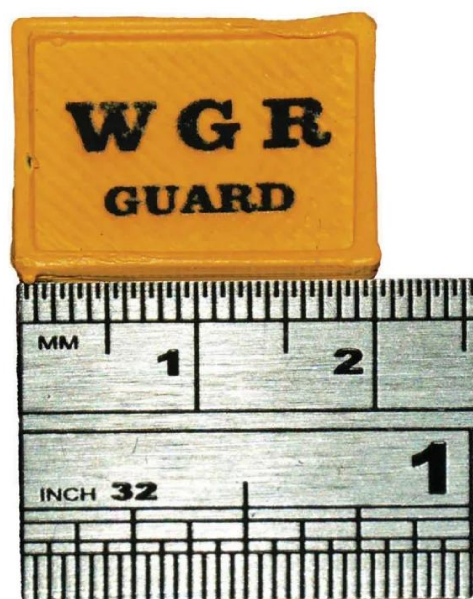
Sharp engraving, but FDM 3D printing struggles with small shapes.
