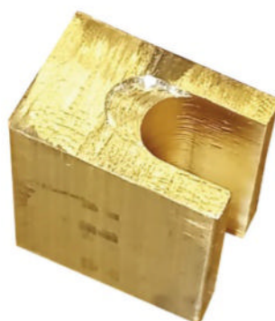
The "U" shaped jig was cut using a bullnosed slot drill. The sides were milled square.
