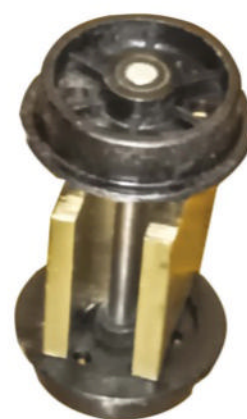
A wheelset to be closed to scale in a vice using a milled jig (U shaped on the milling machine) to ensure that the axles and wheels are supported at 90 degrees.
