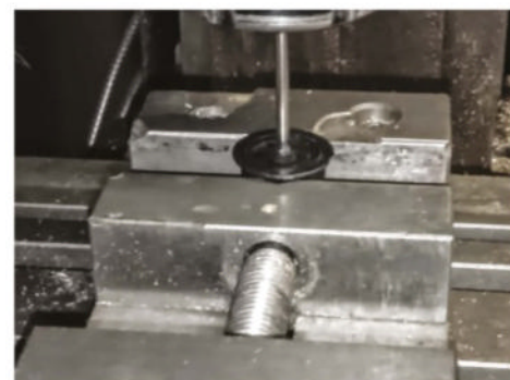
Using the drill press and vice to press the axle into the wheel at 90 degrees.
