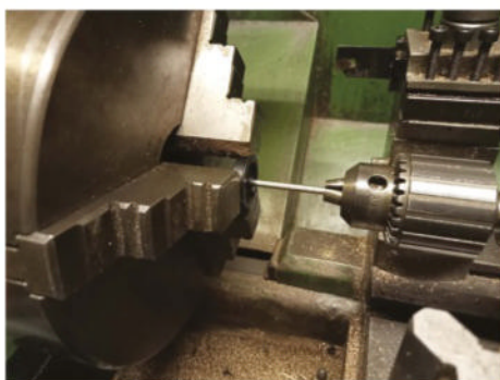
Wheel held in lathe chuck and axle is fed into hole while held in tailstock chuck. This ensures the two items are at 90 degrees.
