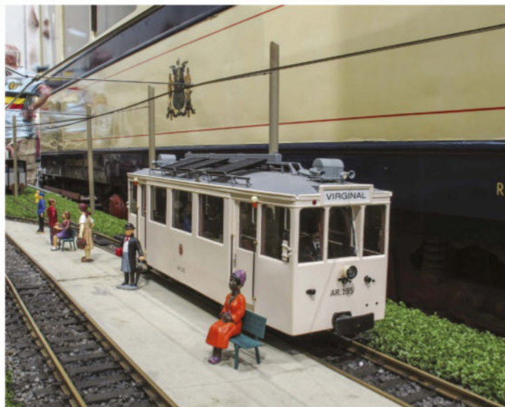
AR 195 - A metal bodied diesel Autorail built by Adrian Nicholes in Plastikard. Fitted with a decoder and sound.
