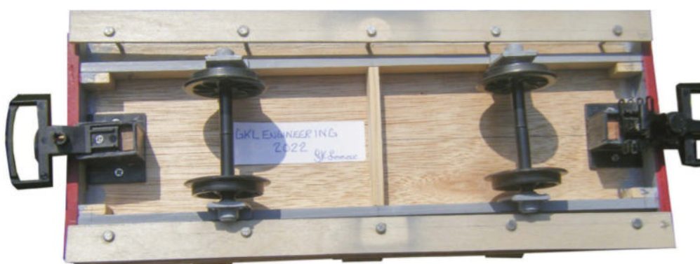
Looking underneath, you can see the LGB coupling fittings made from Plastikard.
