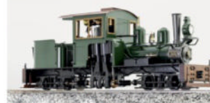
1:20.3 Scale 13-2 Class A Shay The model will be gauge-adjustable for 32mm and 45mm and will come with two types of stack as typically supplied by Lima when built. To be available in black, planished iron or green with expected prices of £2145.00 ready to steam or £1995.00 as a kit. Order for autumn 2023.
