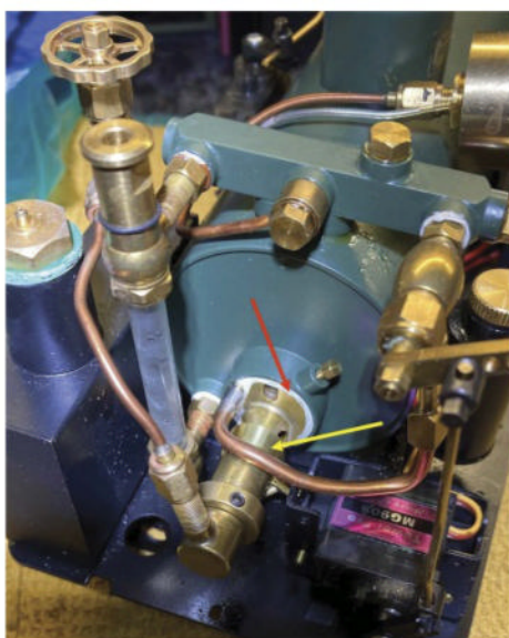
The air control ring (yellow arrow) and PTFE tape around the burner (red arrow).
