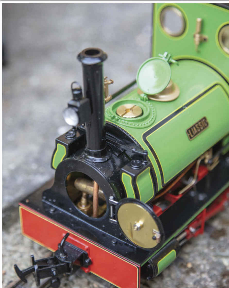
A view of the opening smokebox door, and water filler cap. On ‘Liassic’, the filler cap opens towards the cab to clear the nice little lubricator casting mounted on the chimney.
