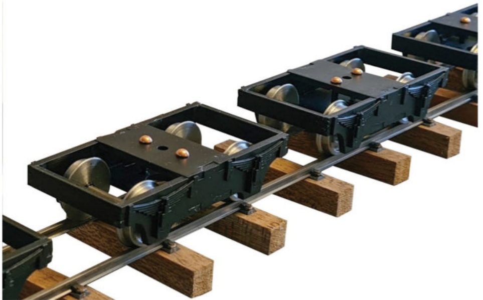
The bogies are fitted with round top rivets. The chassis sits on these and can rock slightly, providing compensation.
