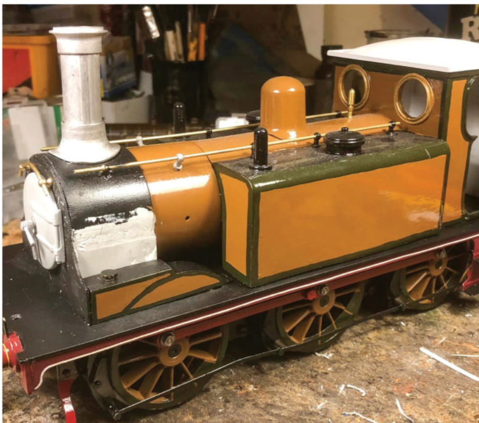
The D shape of the smokebox was created by adding sheets of Plastikard with lots of filler and rubbing back.
