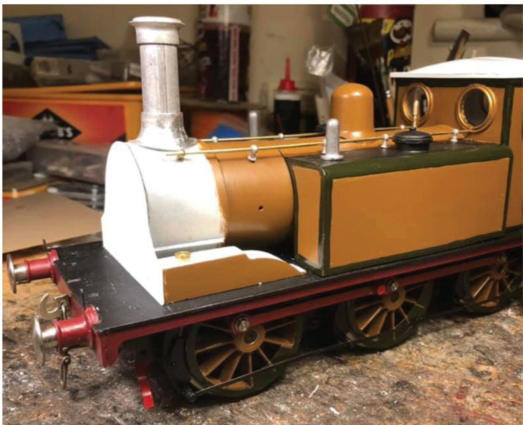
Wingplate fitted to the front, and the sandboxes added to the front splashers.
