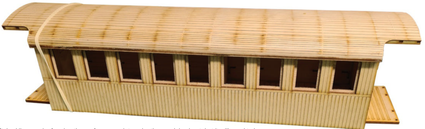
Etched lines make forming the roof curves a lot easier than a plain sheet, but it will need to be covered to hide them.
