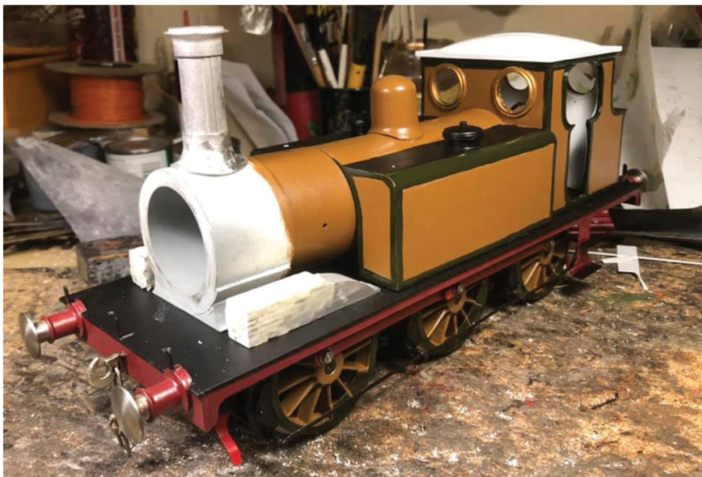
Wingplate fitted to the front, and the sandboxes added to the front splashers.
