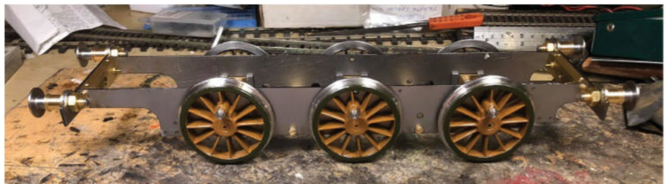
Chassis bolted together including the buffers, wheels and keeper plates.
