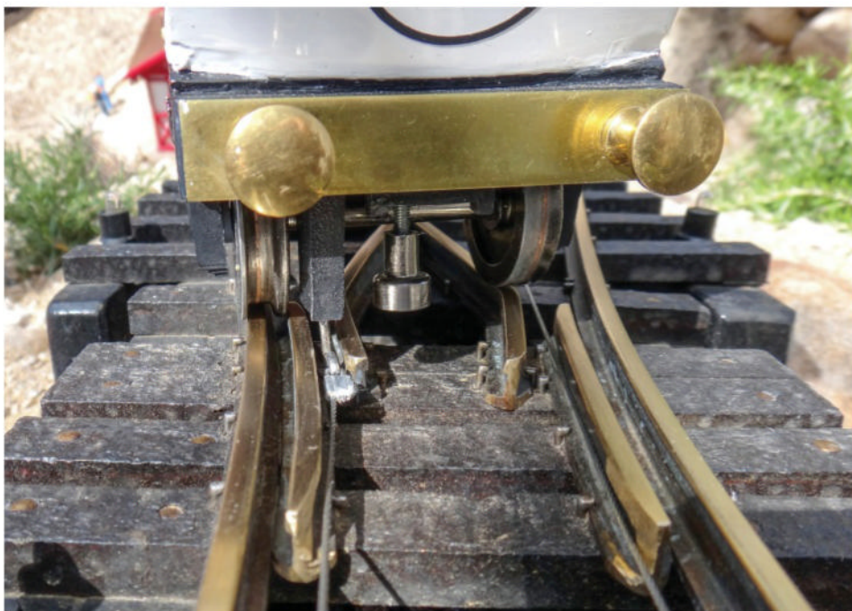
Wheels, cable hook and control magnet passing through lower ABT Switch.
