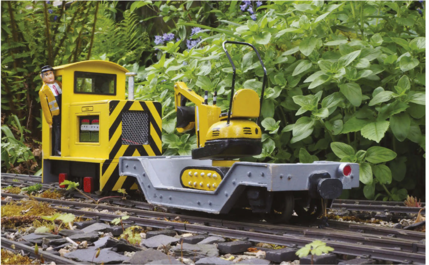
The HGLW semi-scale yard diesel has plenty of power and four-wheel drive on just 2.4 volts.
