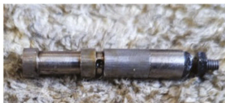
With the loco stripped down, Dave sent me a photo of the valves, which were lightly scored, thanks to the lack of lubrication.
