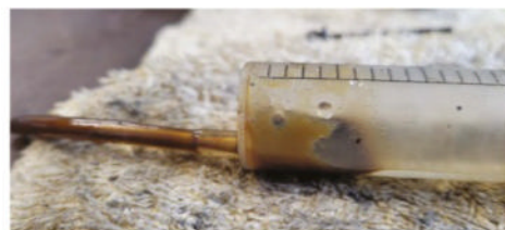
Brown gobs of oil blocking passageways and not lubricating the cylinders.
