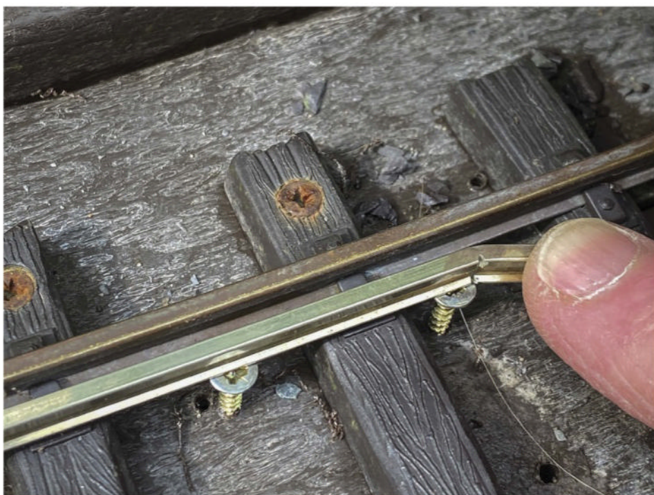
At the start and finish of the checkrail, it's important to angle the rail ends. Cut a notch in the head, and foot of the rail to make it easier to bend neatly.
