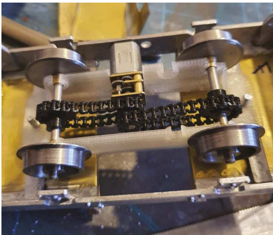
The Micromotor mounted underneath the chassis, and connected to both axles using Delrin chains.
