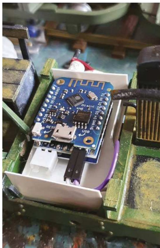
A LocoRemote control unit and the battery pack fit under the engine cover.
