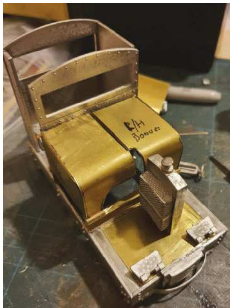
The engine cover was scratch-built with brass sheet. After this photo was taken, a 3D-printed radiator replaced the whitmetal one shown.
