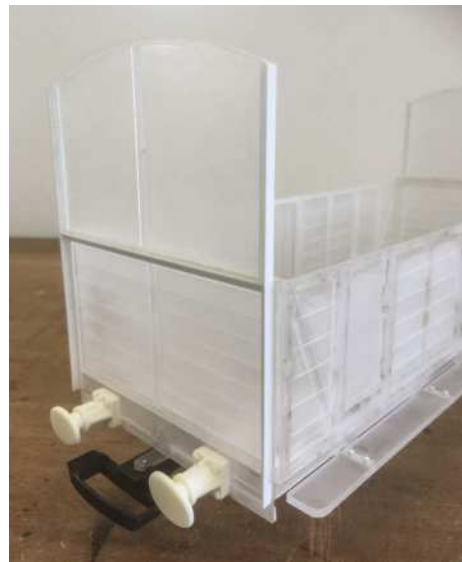
No12 end and side sections joined and test fitted to the chassis.
