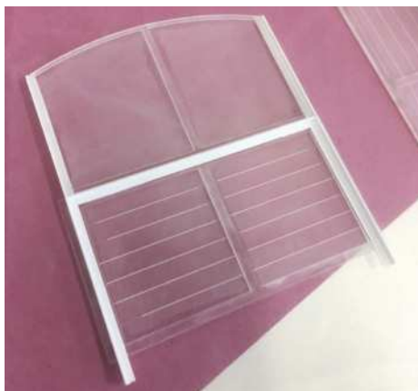
No12 end frames under construction. The panels are 2mm laser-etched and cut acrylic with styrene angle framing.
