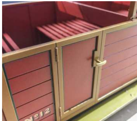
3D printed door handles are painted and fitted to No12.
