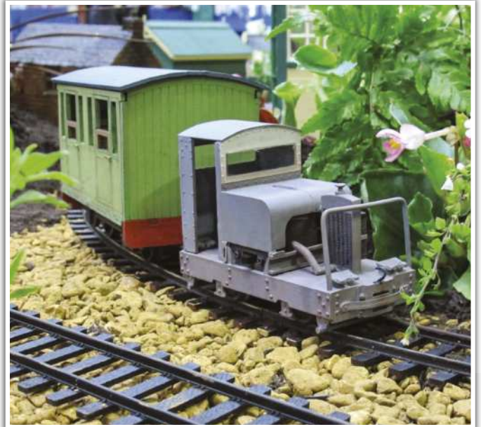
Made of whitemetal and with a double reduction gear set, this Simplex was sure to stay on the track and wasn't short of traction. The Ash Models coach and a single wagon didn't tax it at all.
