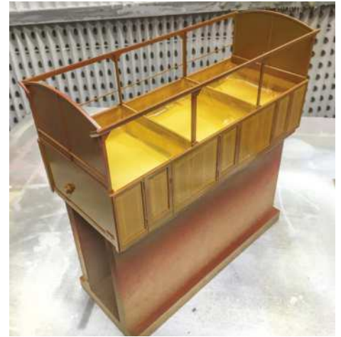
With interiors and panels masked, the bodies are sprayed in Tallyllyn Brown.
