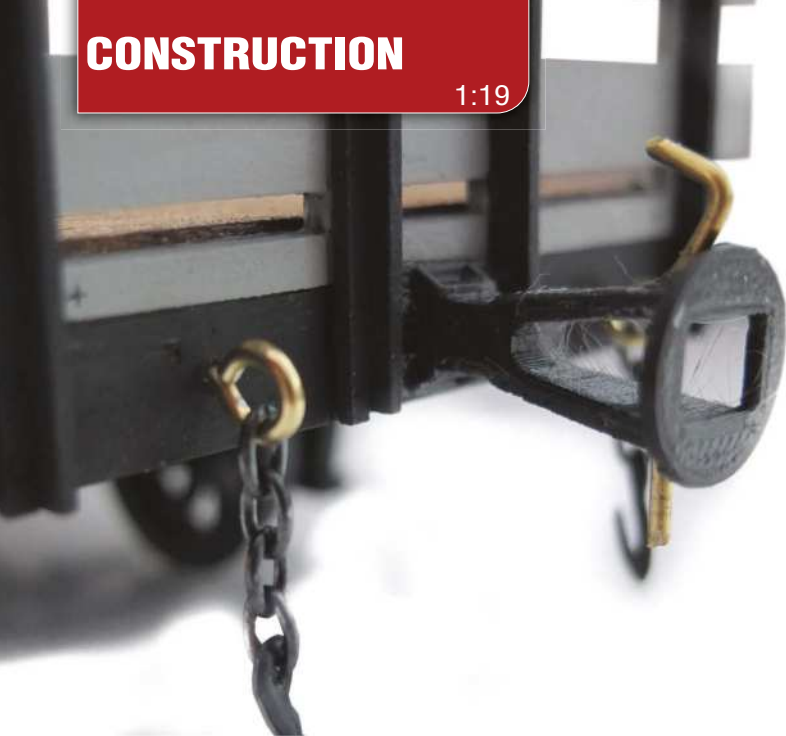
The SLR bell-mouthed couplings and security chains in situ.
