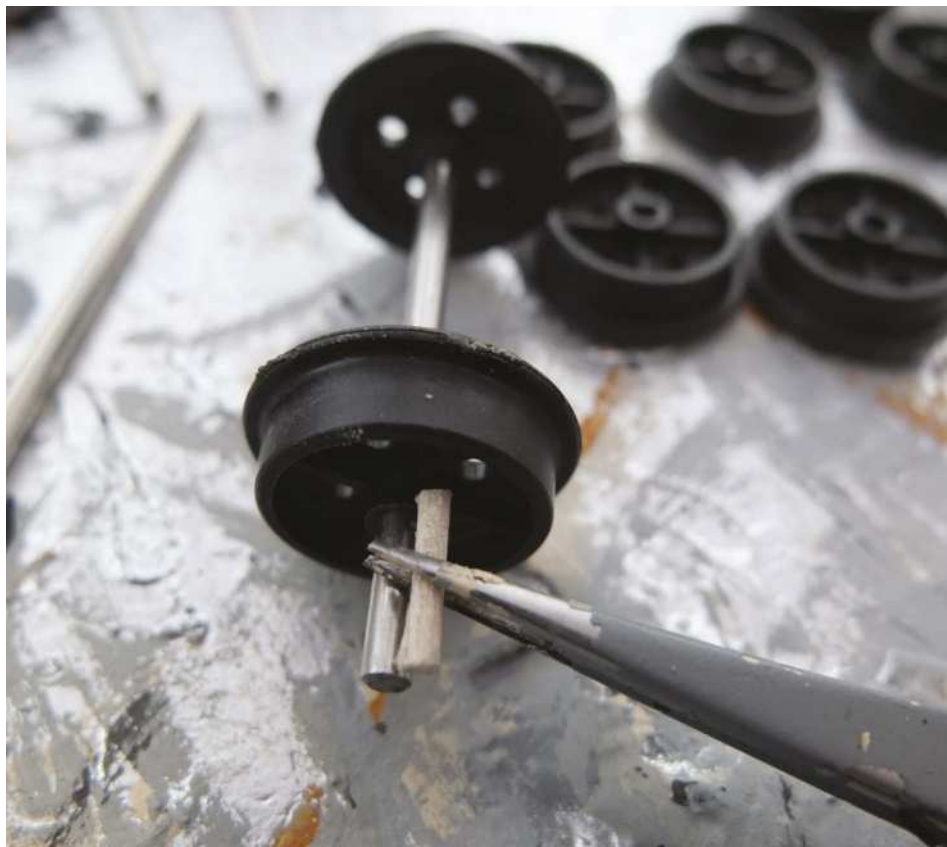
My simple and quick 'cocktail stick trick' to quickly and accurately gauge your wheel sets.
