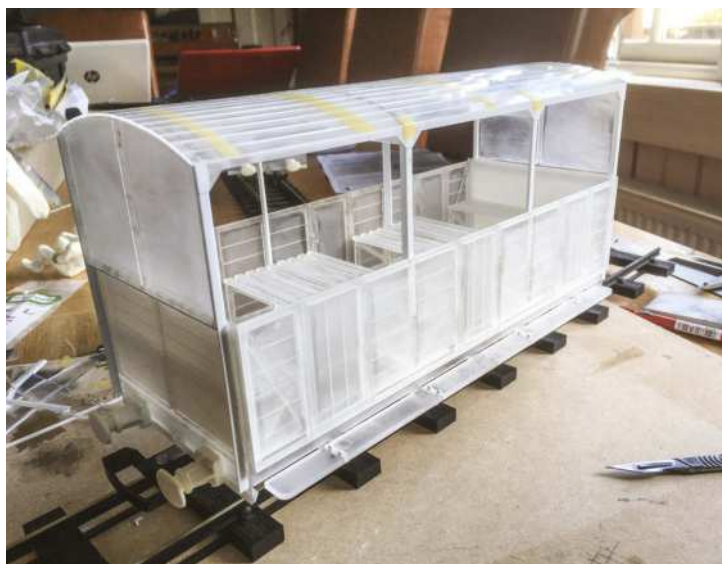
No12 side frames are added to the roof support structure. Inside, you can see the laser-cut seat frames, styrene seat backs will be added later.
