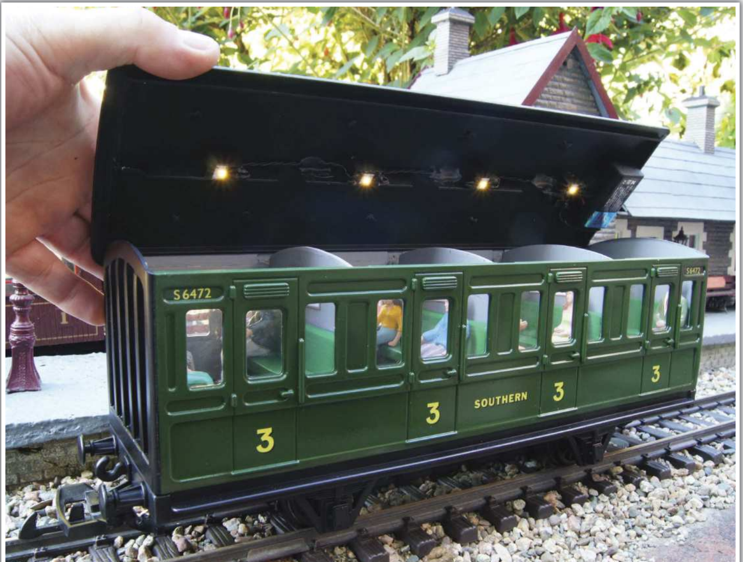
LED lights are glued to Lego blocks fitted under the roof.
