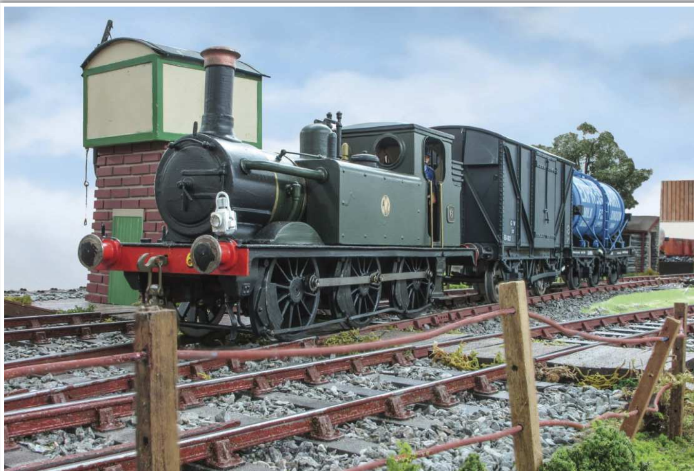
The A1X class Terrier is a GRS kit featuring a three piece resin body mounted onto a steel footplate and buffer beams.
