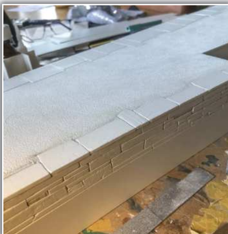
Platform section under construction using 3 and 5mm Foamex.
