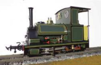
S19-38 'CRANMORE' Peckett 0-4-0ST in 1:19 The model is gauge-adjustable, gas-fired and fitted with a water top up valve. The anticipated UK RRP is £1595.00 and available in Q1 2022. Orders being taken now.
