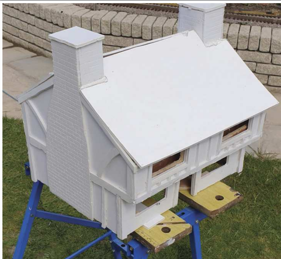
The mock-up was covered with foamboard and sprayed with a white undercoat.
