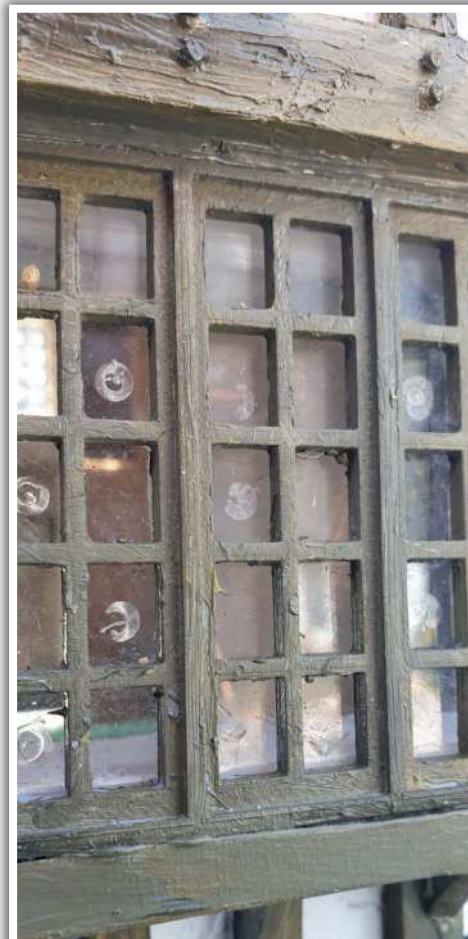
Windows are 3D-printed and glazed with old CD cases. The glass bullions, or bulls-eyes, are a dab of clear glue.
