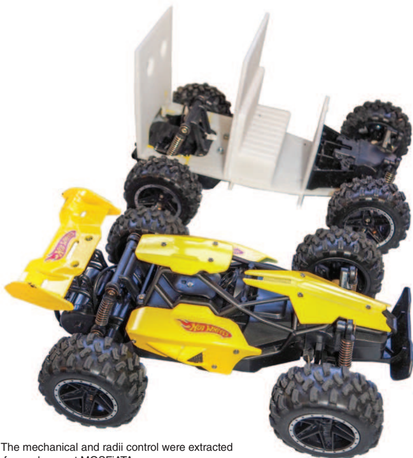
After unbolting from the donor race car, the drive steering and suspension were offered up to the Mostyn Seven chassis.
