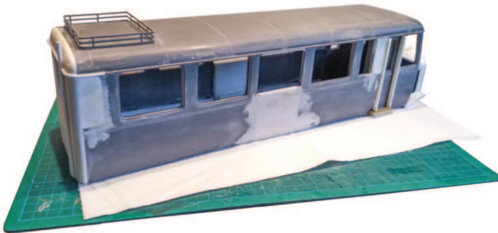
Body alterations showing new front doors, filled in middle doors and curved rear.
