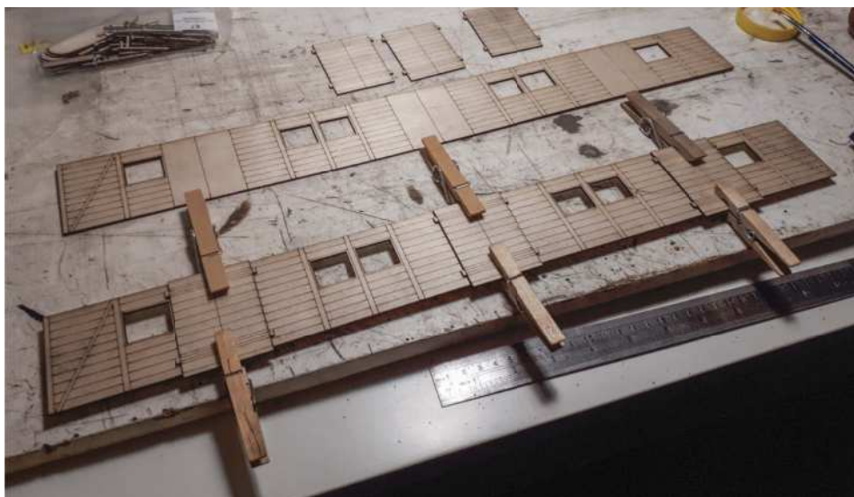
Early stages showing the basic sides to which I'm fitting the doors to make lining up on the underframe easier.
