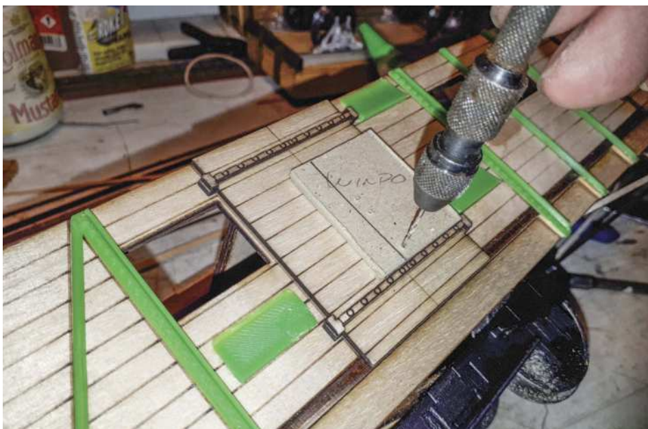
Scrap piece of MDF with three holes for the door handle and grab rail holes. When positioned on the door and drilled through, it ensures all doors are in the same place on each door. All the green parts are 3D-printed detail provided in the kit.
