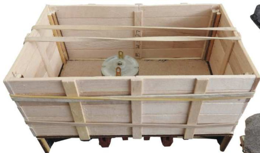
Bringing the sides together using elastic bands to hold everything in place while the glue dries. You can see the corner strengtheners that also support the load.
