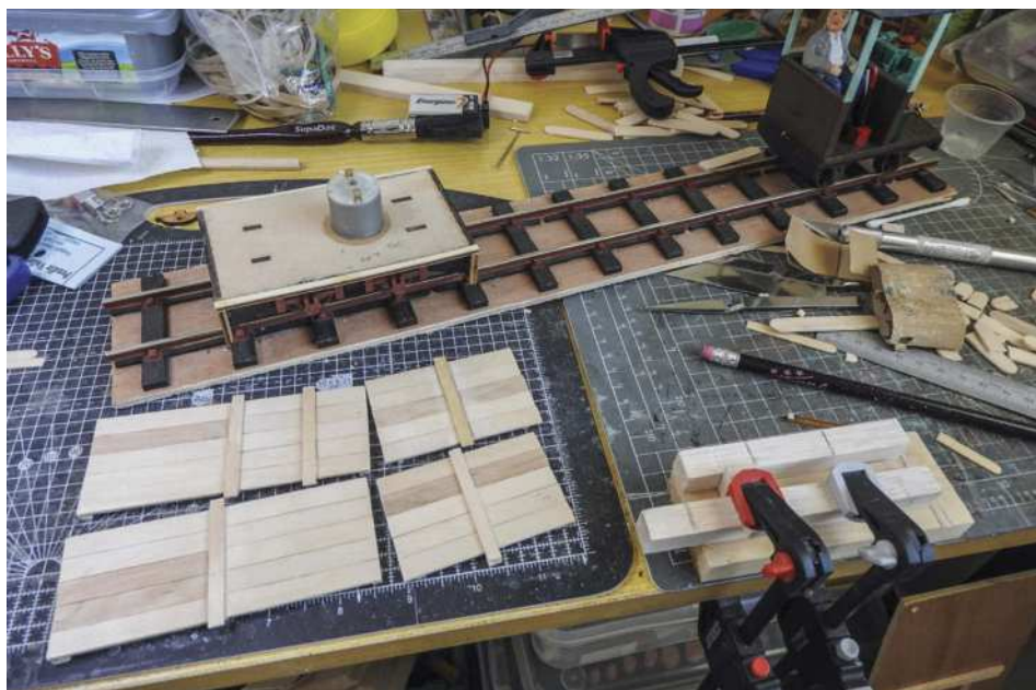
Assembling the wagon sides. Note the cutting jig to keep the plank lengths the same.
