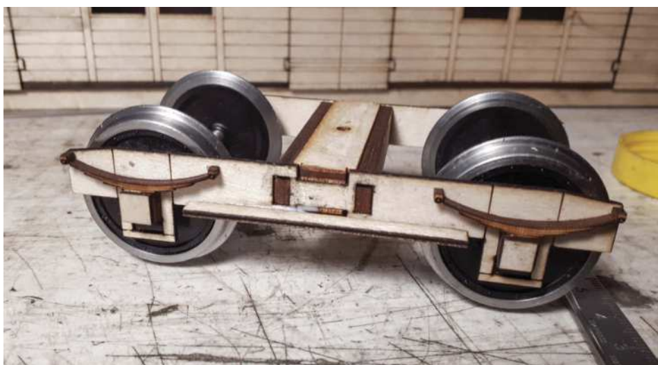
The kit is supplied with laser-cut bogies, which I tried but ultimately replaced with cast versions to add weight to the vehicle.
