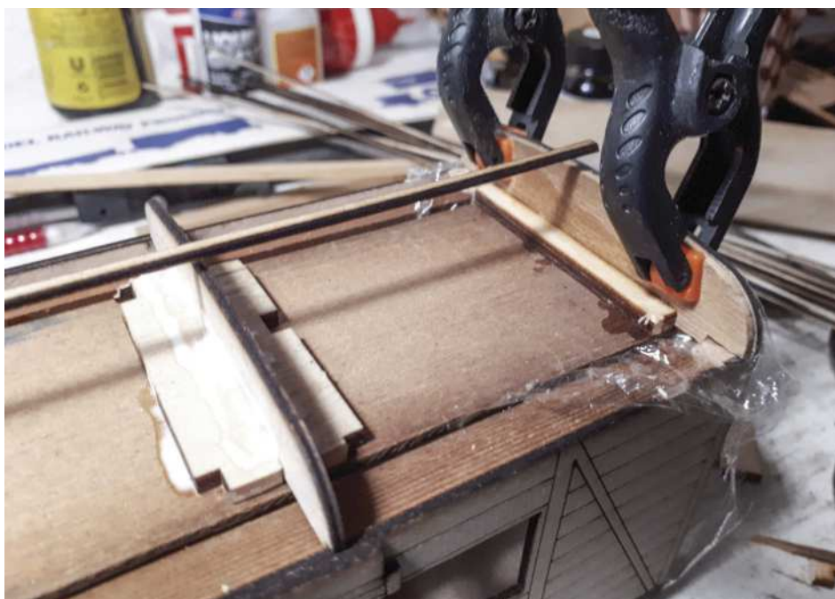
Roof construction showing the spine with the roof profiles mounted and clingfilm to stop everything sticking together.
