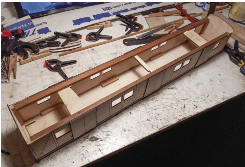
Body assembled, showing the strips of wood II added inside to strengthen corners and edges, side strengtheners and cross braces.
