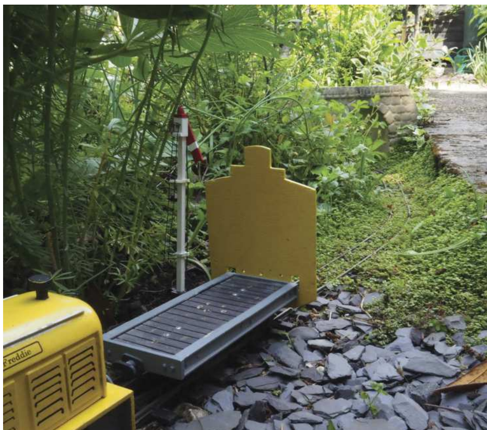
The long wheelbase track checker is mostly fitted with the track gauge. Scissors are still required to cut back the plants which would otherwise invade the tracks.
