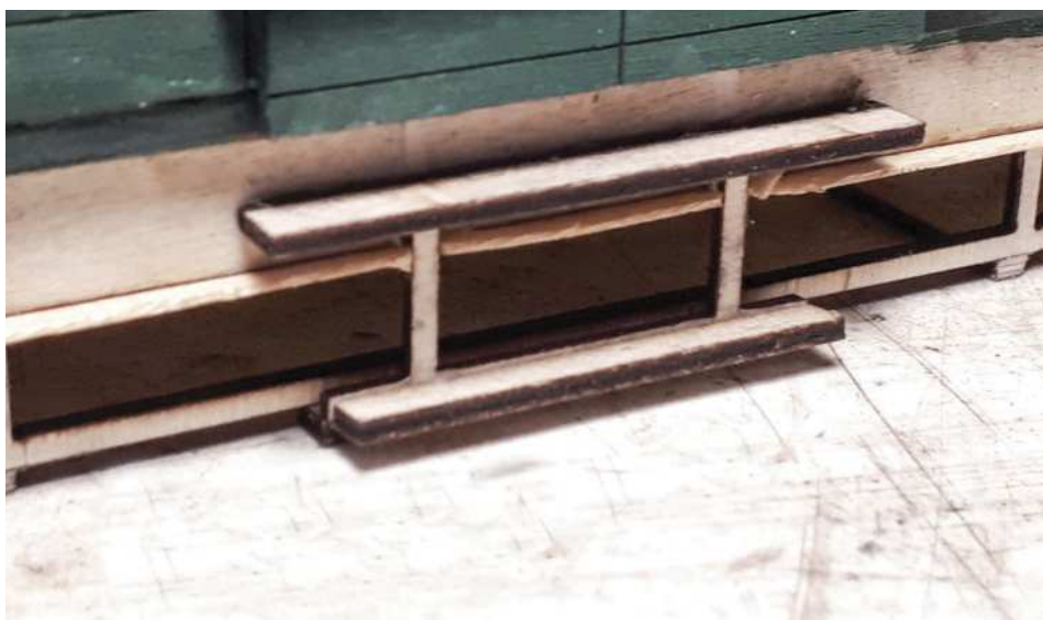
Centre step with strengthening piece to the Truss Rods.
