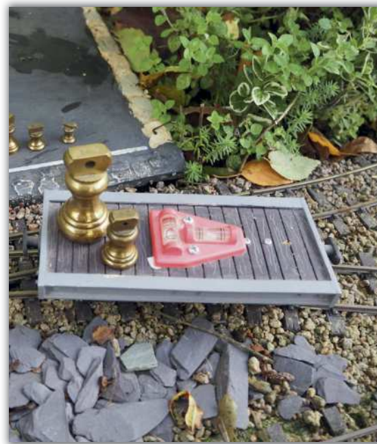
The track measuring wagon has a 3 axis spirit level which can detect tracks out of level and with a counter operating from a crank it measures track distances.
