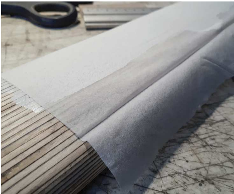
Close up of the roof covering showing the wider strips in the centre and narrow strips at the edge. These are then sanded smooth before the whole thing is covered in tissue paper.
