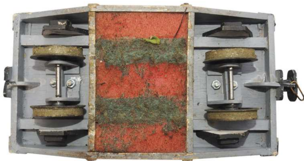
At the start of every days running the track cleaner is run around the track propelled by the yard shunter. A modified dish scrounger brushes the tracks clean. Full details in the July 218 issue.
