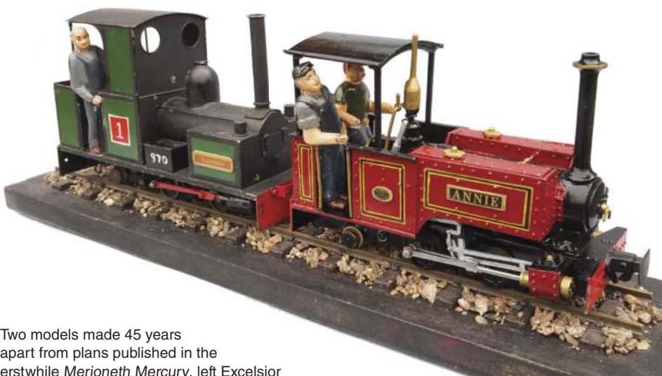
This was Dave's first attempt at lining. The lining was marked out and then drawn using black and yellow paint pens.
