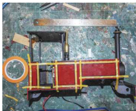
This was Dave's first attempt at lining. The lining was marked out and then drawn using black and yellow paint pens.
