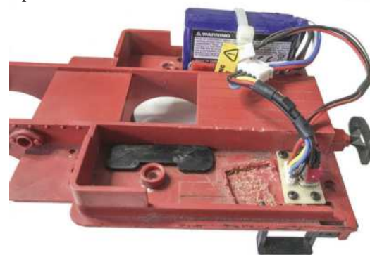
The battery and charging point wiring.
