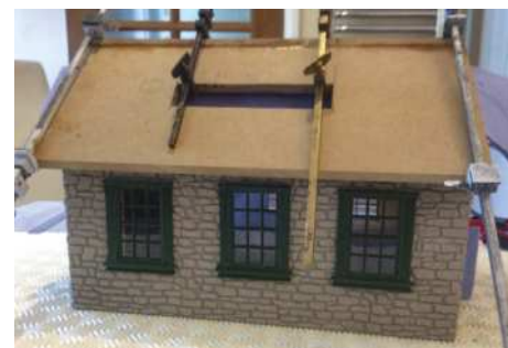
Roof clamped and glued along the ridge line.
