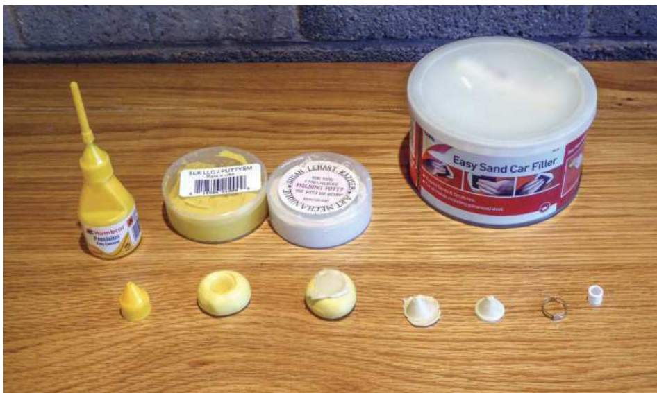
Making the roof vent. From left to right: The glue cap, the mould made by pressing the cap into some 2-part putty, casting with filler, the raw casting, cleaned up casting and finally, the extra detail parts.
