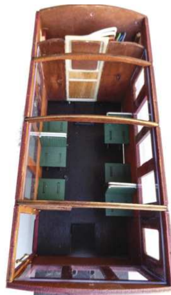
Blanking out the rear windows and adding a partition provides a home for the the electronics.
