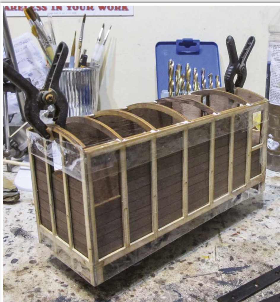
Strapping is added using a mix of clamps and sticky tape to hold it all in place while the glue dries.
