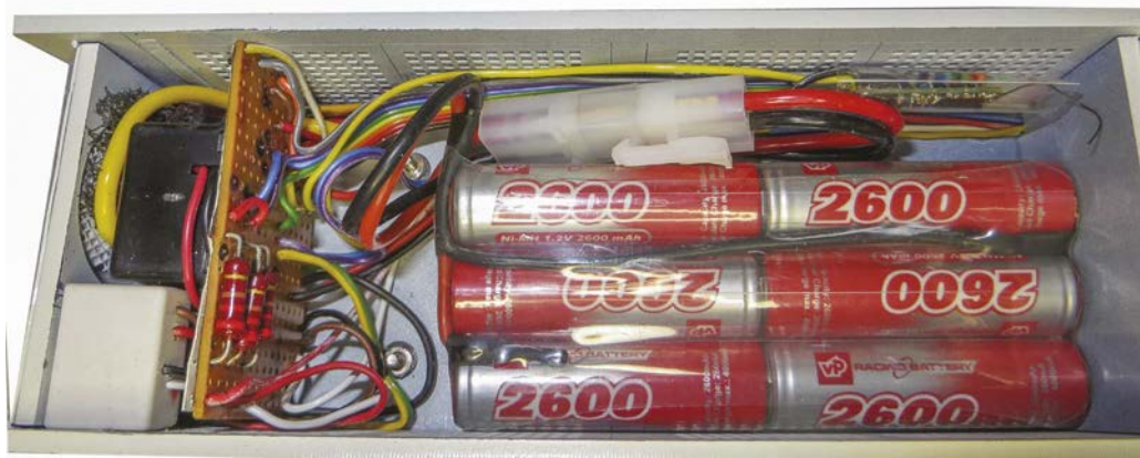
A white box covers the LEDs, the black box is the buzzer, followed by the PCB, batteries and tucked in at the back, the Micron Rx chip.
