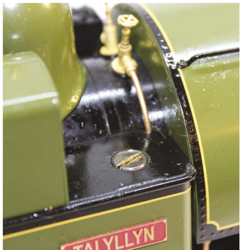
The displacement lubricator cap must be screwed down properly (right) or the oil leaks and the loco won't pull the skin off a rice pudding.
