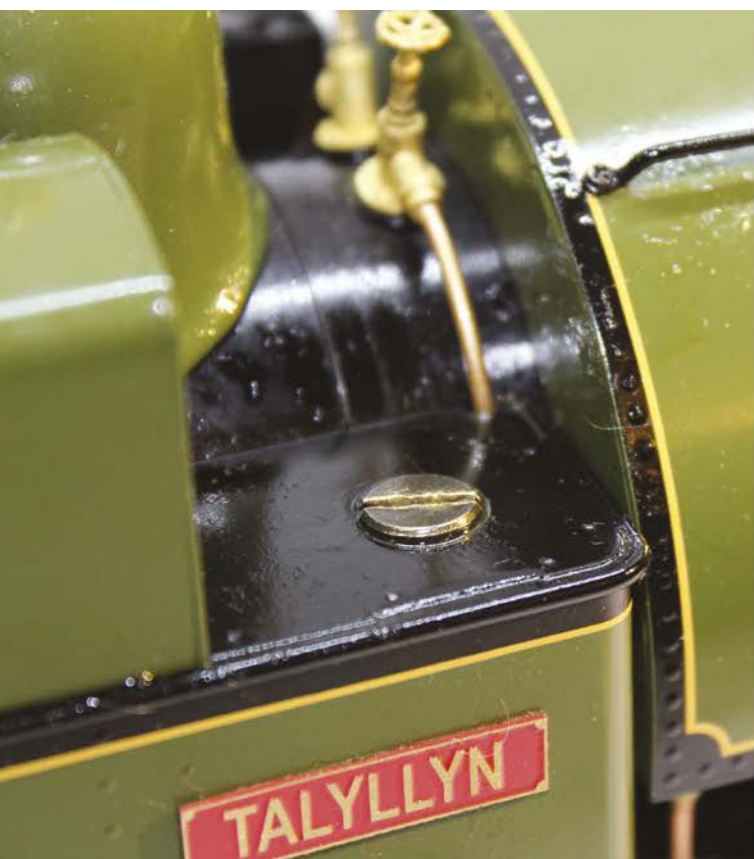
The displacement lubricator cap must be screwed down properly (right) or the oil leaks and the loco won't pull the skin off a rice pudding.
