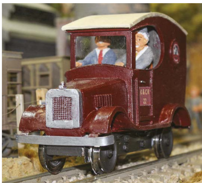
Vern Cracknell - The Kangaroo and Cockatoo Railway needed an Inspection Car for its Division Superintendent, and David Skertchly's Mostyn 7 plans and his method of making mudguards from cereal packet cardboard suited well. The body has been made narrower, and a frame fitted beneath with Bachmann wheels, Como drills motor and bevel gears for the running gear. The figures are handmade.
