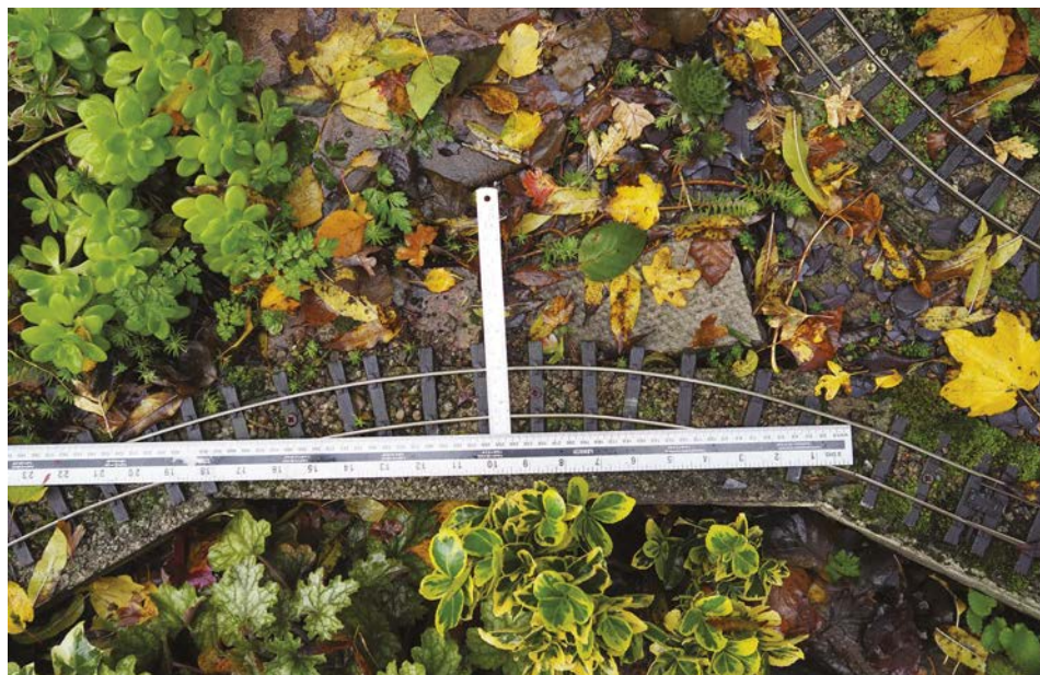
To measure the radius of our curves we can use a pair of rules to measure the width and height of the arc. Dave used a free programme from Handymath.com to do the calculations.
