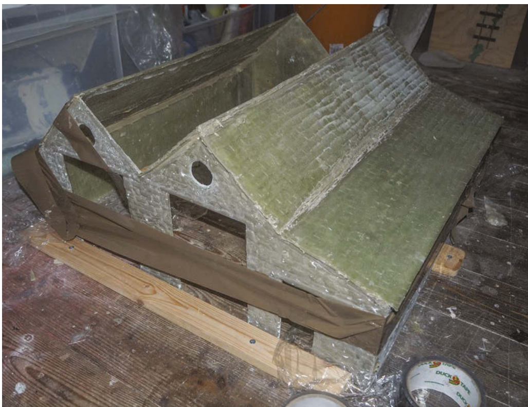
Eventually, Dave ran out of storage space, so the works had to be rebuilt. The walls are laminated using fibreglass on single-use tools cut from hardboard in reverse with block work outline created using a glue gun.
