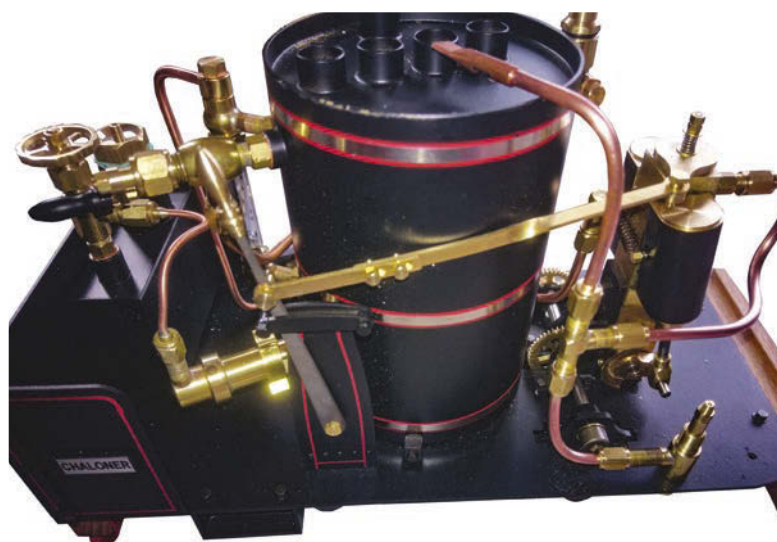
The exhaust is re-routed up the chimney instead of the condenser tank.
