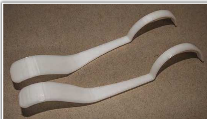
The trickiest part of Dave's original build was the mudguard/footboard pieces, which were laminated from card. 3D-printing allows these curvaceous parts to be made in one piece.
