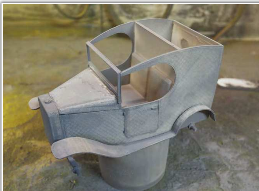
Painting shows up the nice panel lines. The 3D-printing is cross-hatched to try and minimise the filling.
