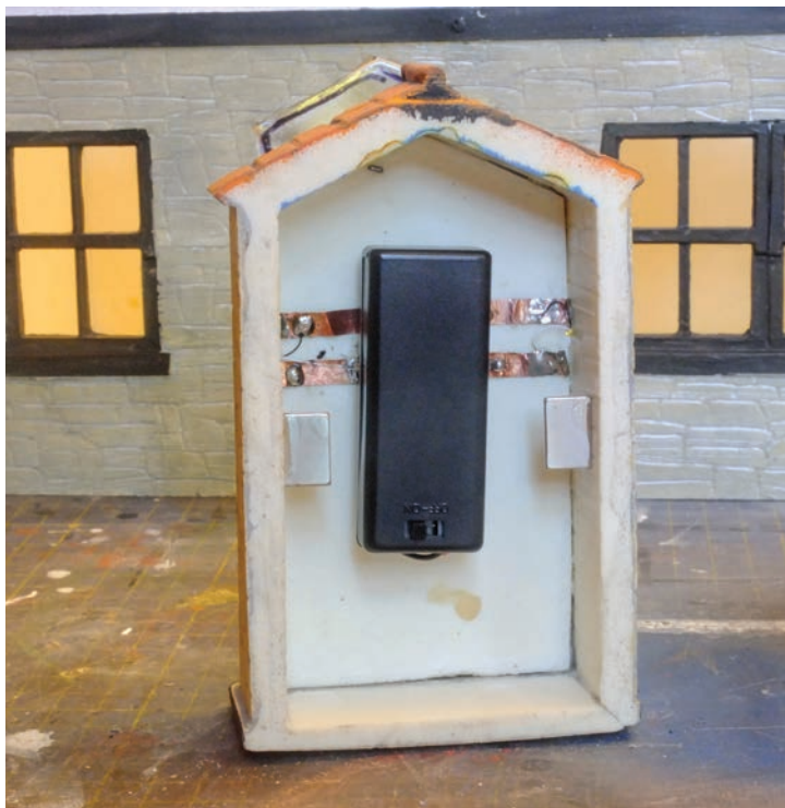
A simple switched AAA battery box hidden in the porch powers the two decorative lamps
