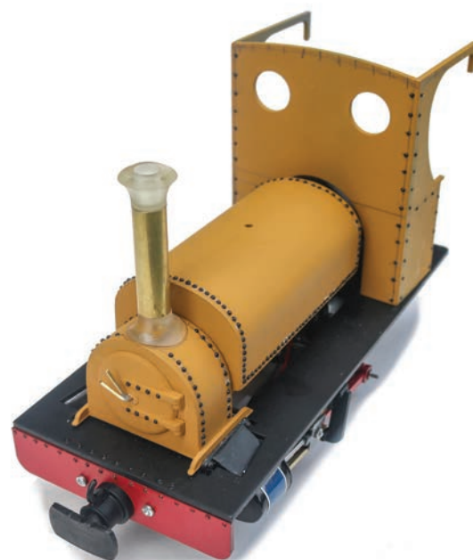
I added loads of plastic rivets from Cambrian Models.
