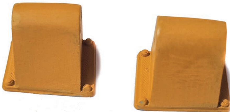
The cylinders are sprayed with high-build primer and sanded.
