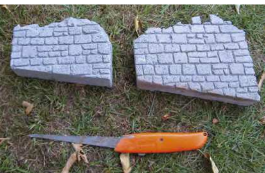
The sections were shaped to fit their intended locations and mortar courses scribed on with a flat-bladed screwdriver and a pad-saw blade.
