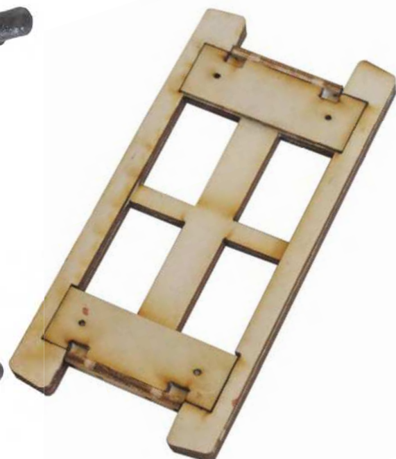
After adding the third and final layer, the chassis is ready for paint and wheels.
