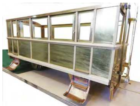
A panelling effect is created by sticking strips of wood onto the brass using superglue. The surface of the brass body is 'roughed' up to aid paint adhesion.
