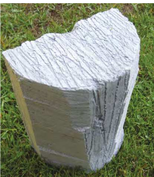
A card template for the semi-circular towers was used to mark the tops of the blocks, which were then roughly cut with the panel saw and finished off with a rasp and a flat file.
