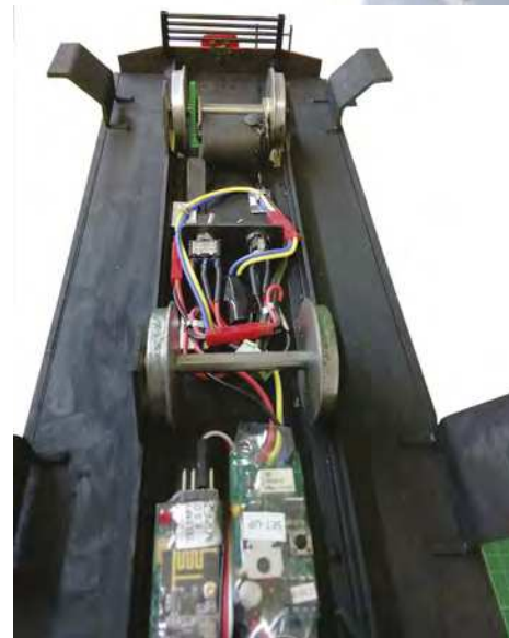
The underside showing the motorised wheel-set and electronics.
