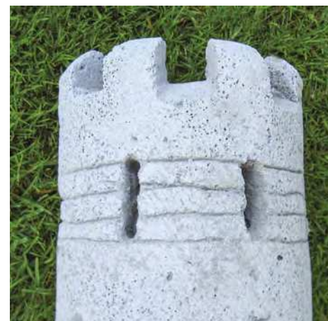
The battlements were then tidied up with the rasp and a flat file. Arrow slits were made with the drill bit and the mortar courses scribed on.
