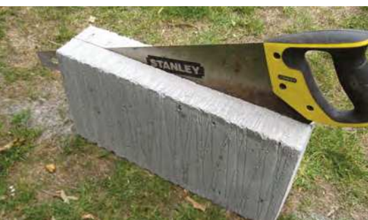
The main sections of the castle walls were roughly sawn with an old, pensioned-off panel saw.
