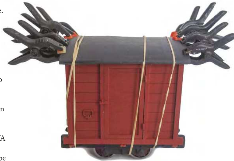
Lots of small clips ensured the roof remained in the right place while the PVA set.
