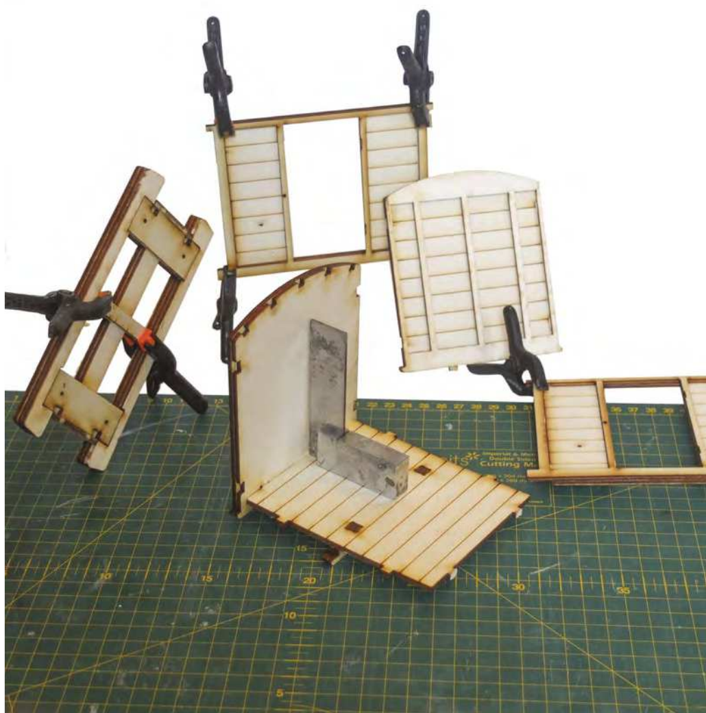
A collection of sub-assemblies for the body. All the parts build up straight and true.
