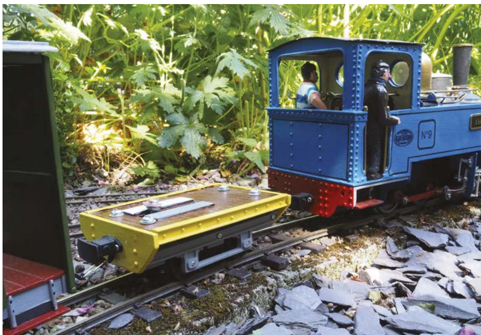
A set of carriages with 12 axles was selected to represent a standard train. The standard train weighed in at 1.7kg. The train was coupled up with the dynamometer between the engine and the train.
