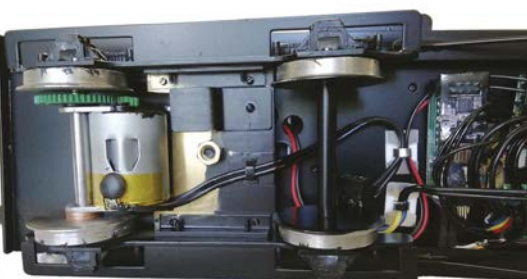
The underside of the power bogie showing Fosworks traction unit and radio control unit.
