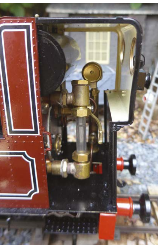
LHS of cab showing sight glass and regulator handle.
