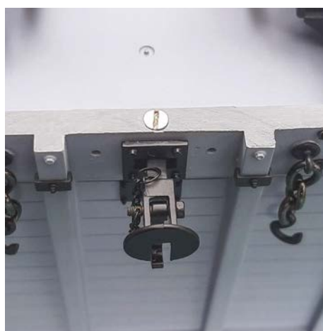
The new coupling is held in place with an 8BA x 1/2" long countersunk screw, which also acts as a pivot.
