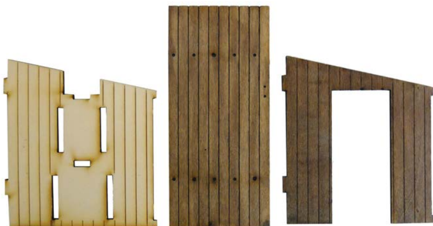
The results of the Colron wood dye. From left to right, bare wood, one coat, two coats.
