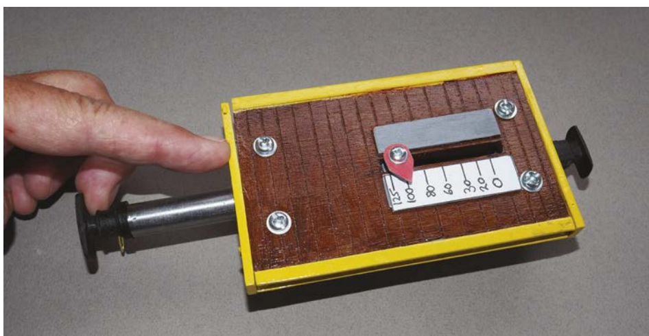
The dynamometer in Engineering department yellow and grey paint with a wooden floor. At rest or with no load the plunger is retracted. As the draw bar force increases against the spring the plunger extends enabling a reading of the force to be taken from the scale.
