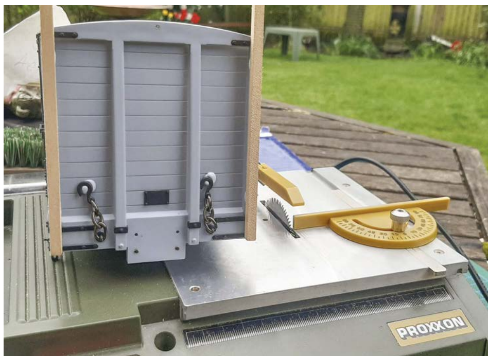
A couple of 3mm square packers were then attached to the end of the wagon with Blu Tack to keep everything square before the tab is cut off on the circular table saw.
