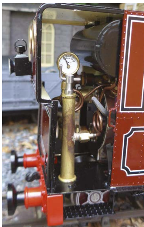
RHS of cab showing pressure gauge, gas regulator valve and reversing lever.
