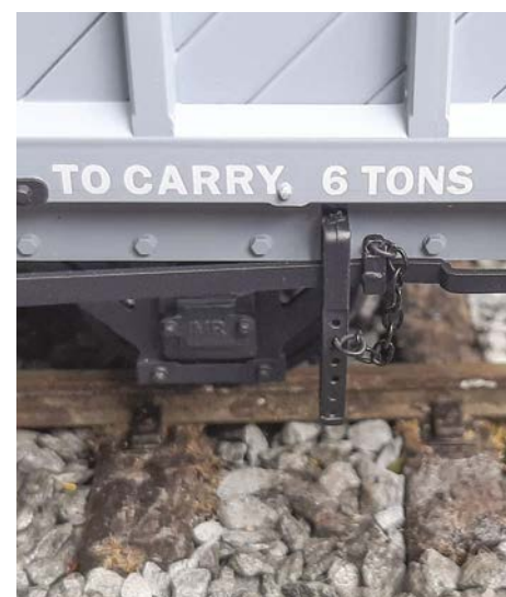
Flipping the brake lever over means the cranked handle now correctly steps-out from the frame rather than in, at the cost of the chain now being fitted to the top.
